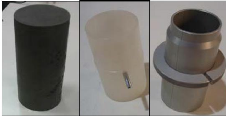
Fig. A 1.9 Trimmed cohesive specimen (left); membrane suction stretcher (middle); split-part mould for granular specimen preparation (right).
