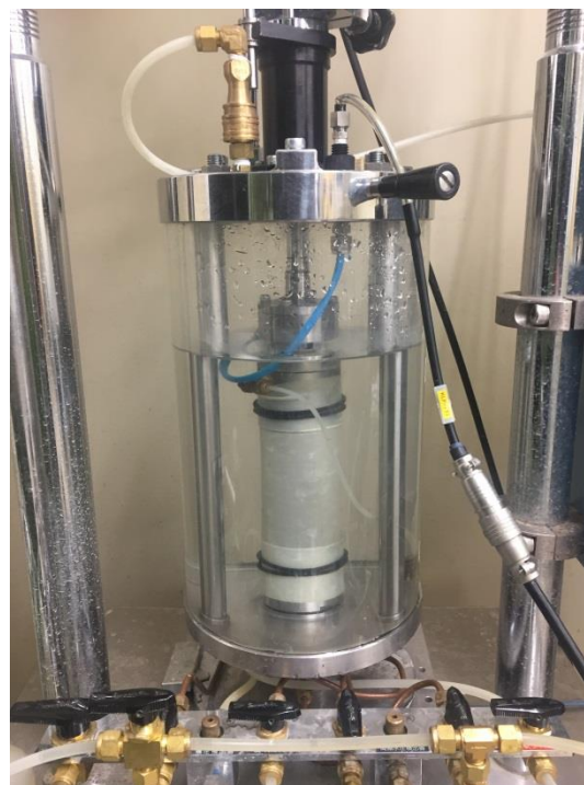
Fig. A 1.11 Specimen in Triaxial cell with Cell pressure 10kPa
