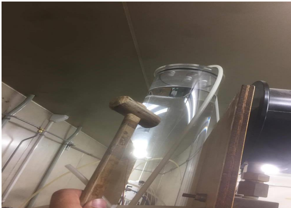
Fig. A1.8 Checking if the distilled water is completely de-aired or not
