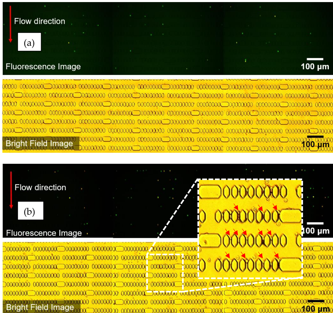
Figure 2.8 Microfluidic device show no clogging (cells clogging) using 1 \mu\text{L} (a) and 2 \mu\text{L} (b) of whole blood. The bright field images confirm the results. Images was taken at 6 \mu\text{m} gap size, centre of microfluidic device for comparison. Red arrows show the captured cells
