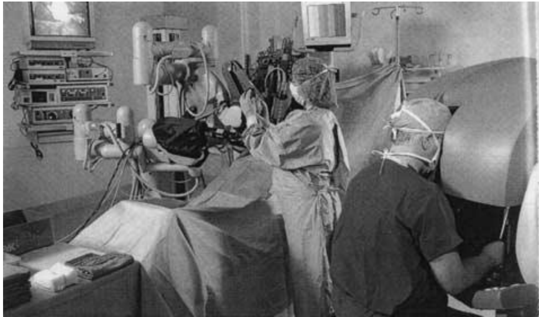
Figure 1.3. Simulated setup of the operating room for a telerobotic laparoscopic cholecystectomy using the da vinci telerobotic surgical system[34].
