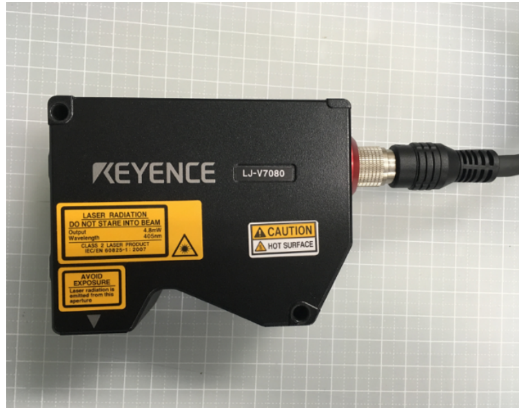
Figure 2.7: High-speed laser profiler (KEYENCE LJ-V7080) used to measure the profile of a relaxing granular heap.
