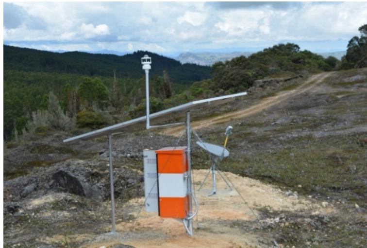
Figure 18. Data transmission via satellite internet link, MET sensor and enclosure at TEAT station.
