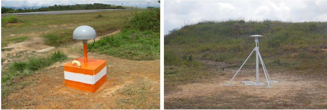
Figure 30. Monumentation type of PAL1 station (left) and PAL2 station (right).
