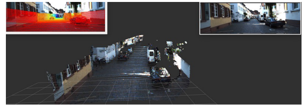
Fig. 5 Result of the real time Image-Cloud fusion using a Velodyne HDL-64 and a wide-angle camera.
