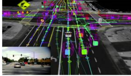
Figure 1-8: Understanding other road users' intentions and likely trajectories is very useful in highly dynamic environments.
