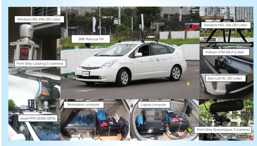
Figure 1-2: sensor suite for Nagoya University Autonomous vehicle.
