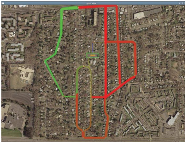
Figure 2-2: Global planning: DP propagates values through a crude discrete version of the environment map. The color of the RNDF is representative of the cost to move to the goal from each position in the graph. Low costs are green, and high costs are red [36].
