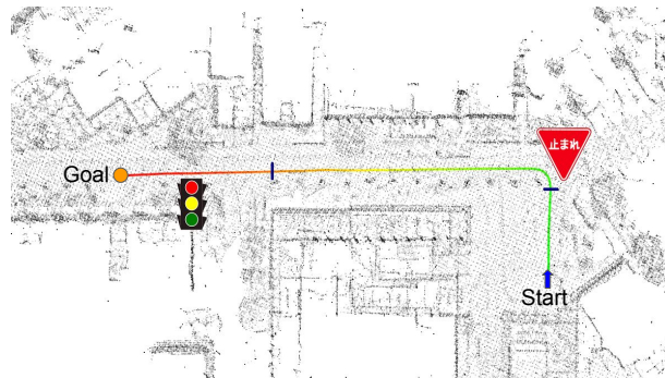
Figure 3-16: Experimental vector map with stop lines and traffic light.
