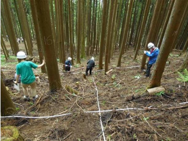
Fig. 1. Surveying plot setting (15 × 15 meters square)
