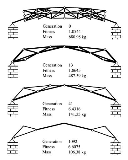
Fig. 42: Obtained Solutions of Planer Hybrid Arch
