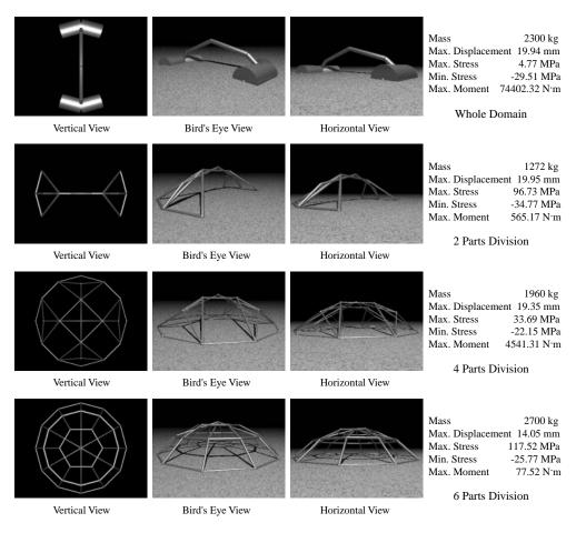
Fig. 40: Obtained Solutions of Sphere Frame Dome
