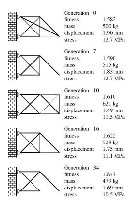
Fig. 24: Cantilever 15-Bar Truss
