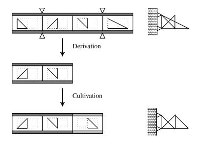
Fig. 18: Mutation Based on Triangular Element
