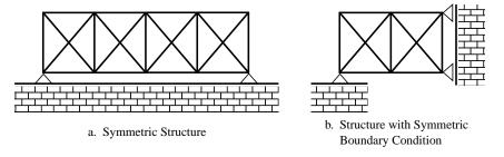
Fig. 14: Structural Analysis with Symmetric Boundry Conditioner
