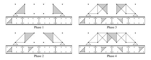
Fig. 16: Generation of Truss Topology with Topological Symmetricity
