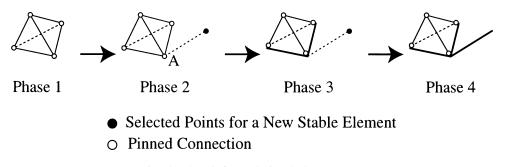
Fig. 13: The rule for producing the 3D structures
