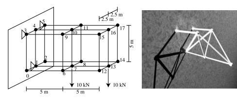
Fig. 26: 3-Dimensional Cantilever Truss
