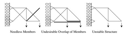
Fig. 1: Undesirable Structures
