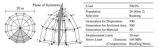
Fig. 27: Sphere Truss Dome
