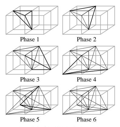
Fig. 6: Producing of The Initial 3-Dimensional Truss Topology
