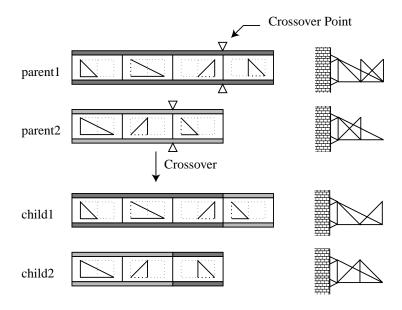
Fig. 17: Crossover Based on Triangular Element
