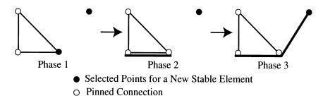
Fig. 11: The Rule for Producing Planer Discrete Structures
