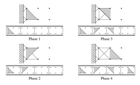
Fig. 3: Truss Topology Consisting of Triangles
