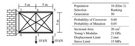
Fig. 22: 15-Bar Cantilever Truss
