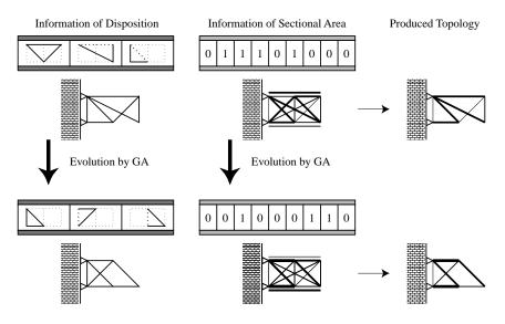
Fig. 19: Expression of Truss Topology by Plural Variables
