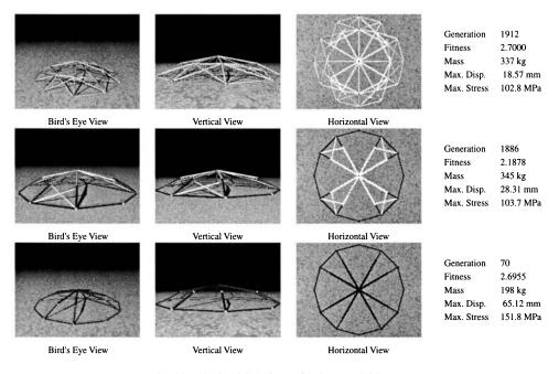
Fig. 44: Obtained Solutions of Sphere Hybrid Dome
