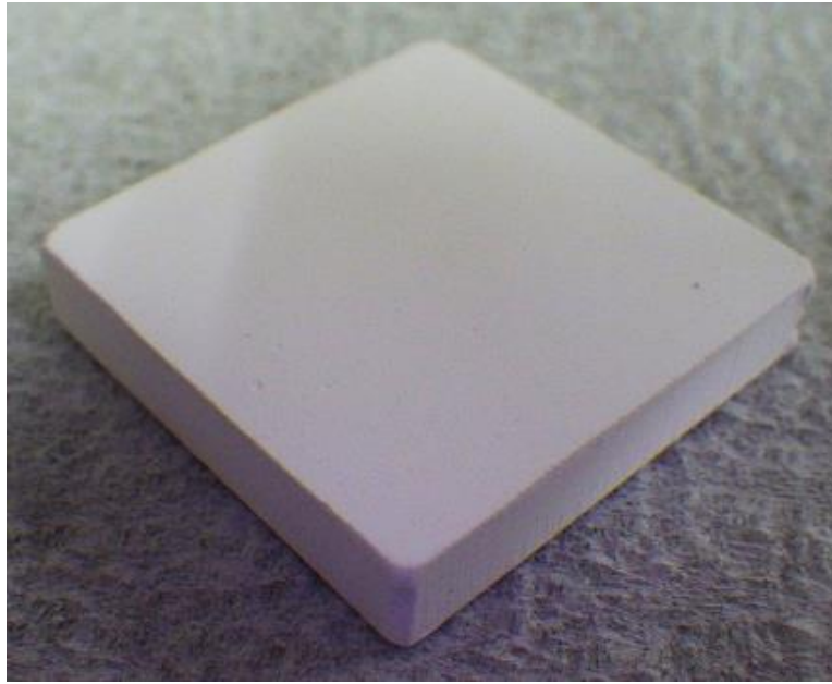
Fig. 55 Photograph of sample for Thermal conductivity measurement (Improved \text{CaSO}_4 )
