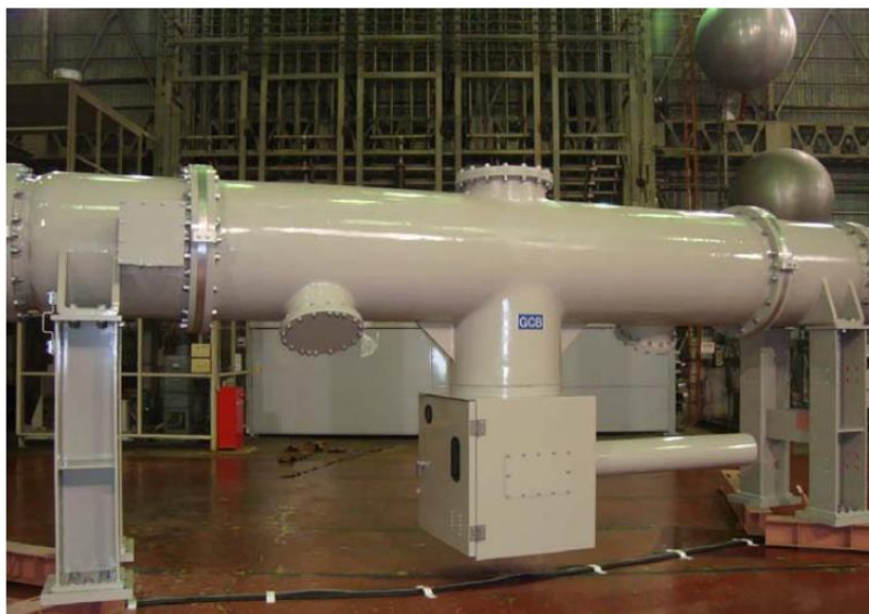
Figure. 1-3. 550 kV/63 kA SF 6 gas circuit-breaker (GCB) with spring mechanism [9].
