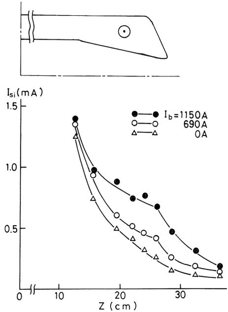
Fig. 26(b) Configuration of surmac coil (upper) and the axial distribution of the second peak (lower).
