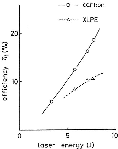
Fig. 17 Dependence of  $\eta_1$  on laser energy.
