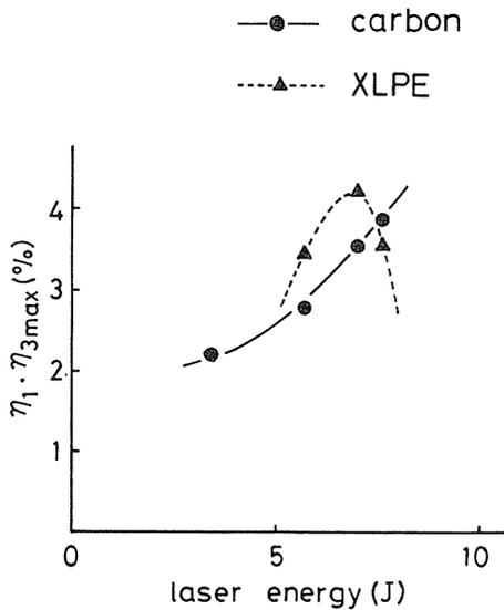
Fig. 15 Dependence of  $\eta_1 \eta_{3max}$  on laser energy.
