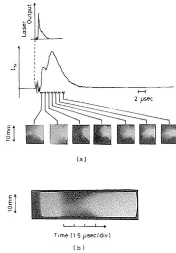
Fig. 24 Laser output (top), typical waveform of the saturation current (middle) and framing-mode pictures taken at intervals of 1 μs and framing rate of  $1 \times 10^6$  frames per second for the generation process of laser-produced plasma (bottom) (a) and the photograph of the streak mode taken at 3 cm from the target (b).
