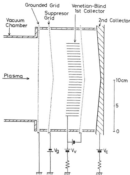
Fig. 10 The PDC with two collectors.
