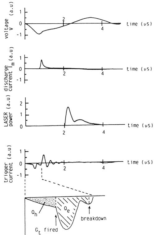
Fig. 5 Temporal characteristics of voltage across the main electrode, main discharge current, laser output power, trigger current. The definition of  $Q_h$  and  $Q_e$  is also shown in the lowest figure.
