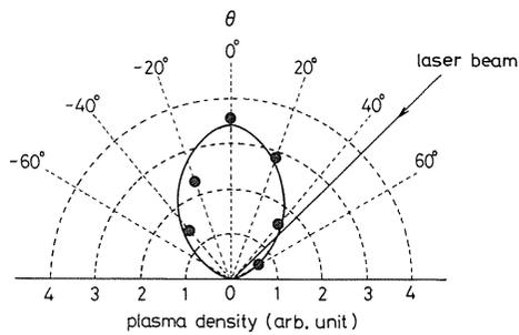
Fig. 14 Angle dependence of the expansion plasma.
