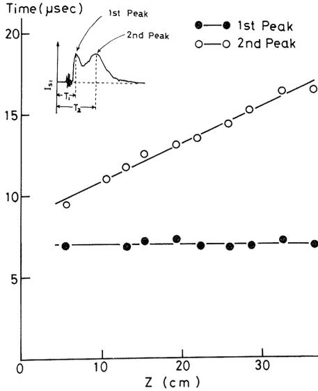
Fig. 26(a) Arrival time of the first and the second peaks of ion saturation current with position along the Z-direction.
