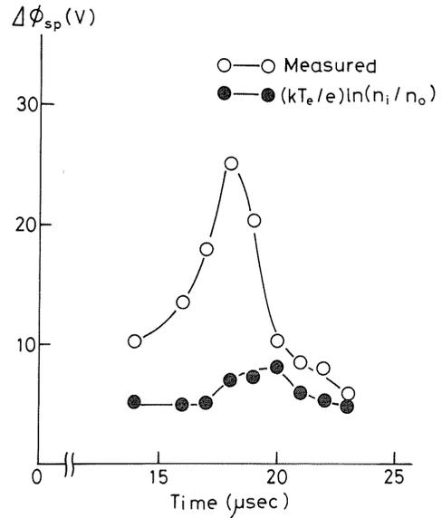
Fig. 29 Potential difference  $\Delta\Phi_{sp}$  calculated by the measured plasma densities using the equation of the ambipolar ( $\bullet$ ) and the measured plasma potential ( $\circ$ ).
