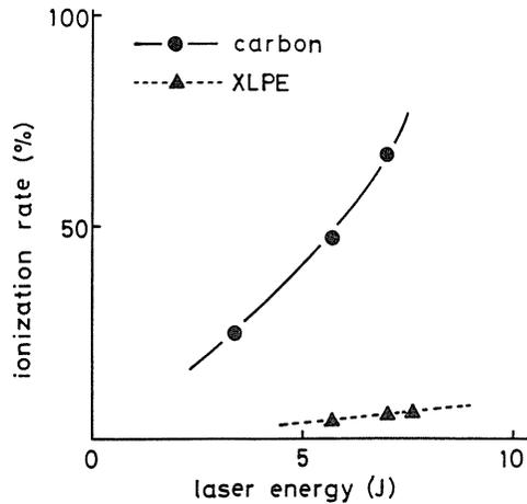
Fig. 19 Dependence of ionization rate on laser energy.
