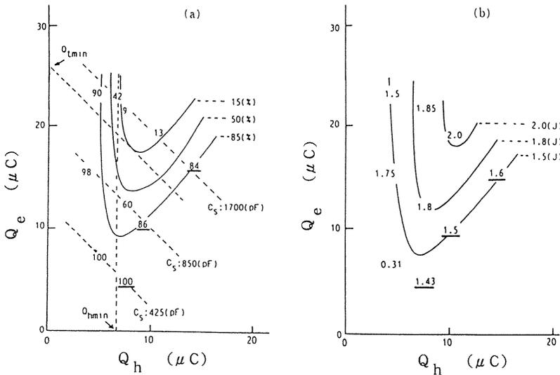
Fig. 8 Contour lines of (a) glow-to-arc transition rate and (b) laser output as functions of electrical charge  $Q_h$  and  $Q_e$ .
