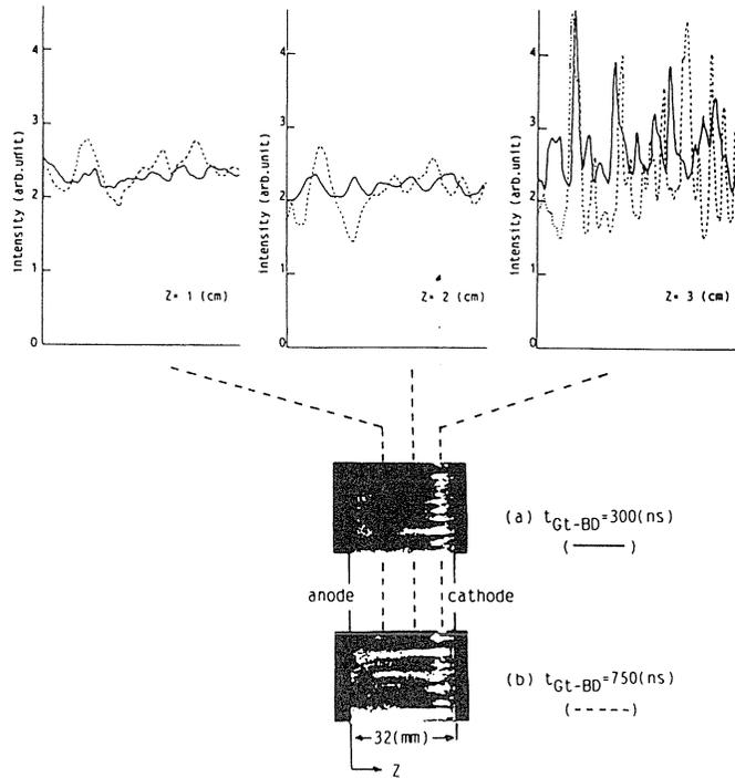
Fig. 6 Spatial distribution and time-integrated photographs of radiation intensity along the glass tube at (a)  $t_{Gt-BD}=300$  ns, and (b)  $t_{Gt-BD}=750$  ns.
