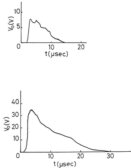
Fig. 30 Output from the PDC as a function of time for without (a) and with (b) magnetic field.
