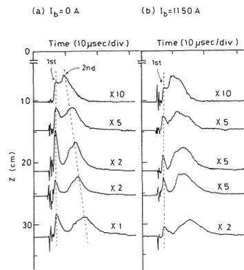
Fig. 25 Axial distribution of ion saturation current  $I_{si}$  as a function of time without (a) and with (b) magnetic field.
