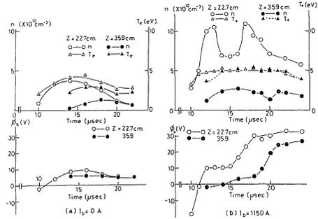
Fig. 28 Time evolution of  $T_e$ ,  $n$  and  $\Phi_s$  at  $Z=22.7$  cm and  $35.9$  cm without (a) and with (b) magnetic field.
