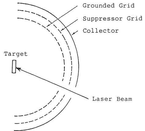
Fig. 16 The PDC distributed around the target hemispherically.
