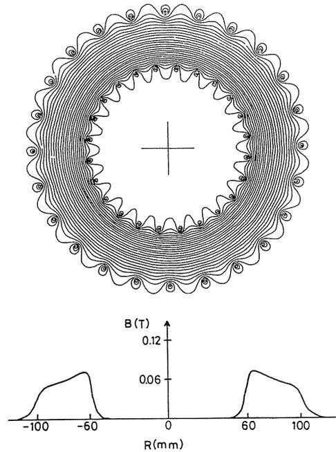
Fig. 23 Calculated distribution of the magnetic line of force at the central cross section of the surmac coil (a) and the calculated magnetic flux density at the coil current  $I_0=1000$  A (b).
