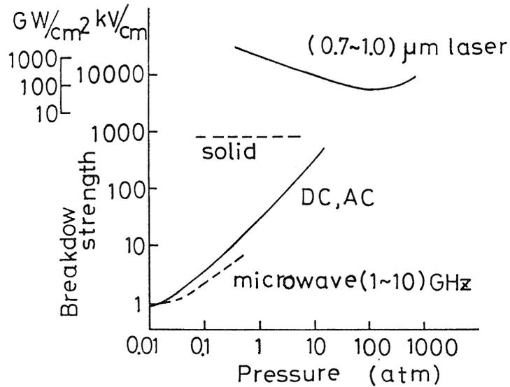
Fig. 2 Breakdown strength of air against pressure.
