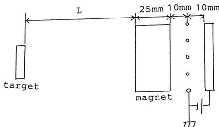
Fig. 33 Measurements of percent of magnetic separation.
