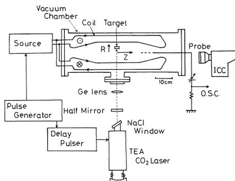
Fig. 21 Experimental set up for the surface magnetic confinement.
