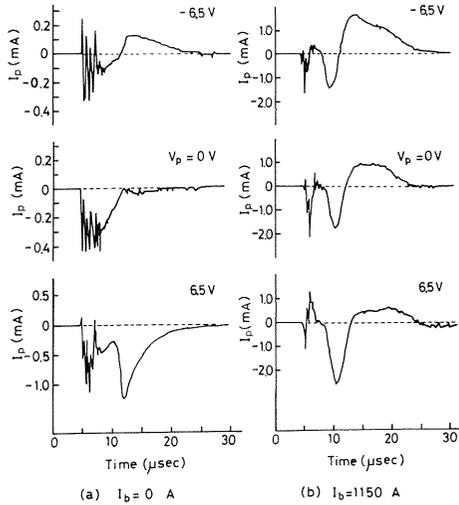
Fig. 27 Probe current measured at the point  $R=0$  and  $Z=22.7$  cm by varying the probe voltage  $V_p$ .
