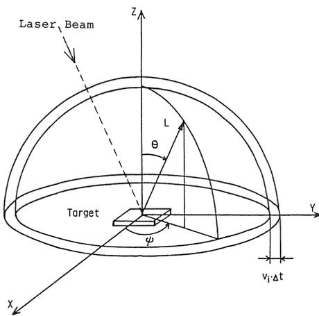
Fig. 13 Polar coordinates used for the calculation.
