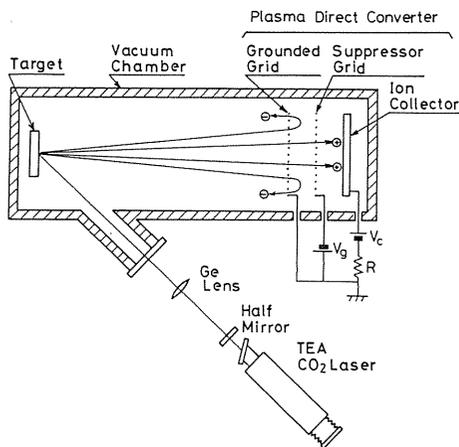
Fig. 9 Principle of energy conversion from laser energy to electricity.
