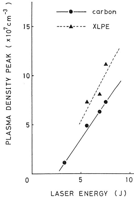
Fig. 18 Dependence of ion density on laser energy.
