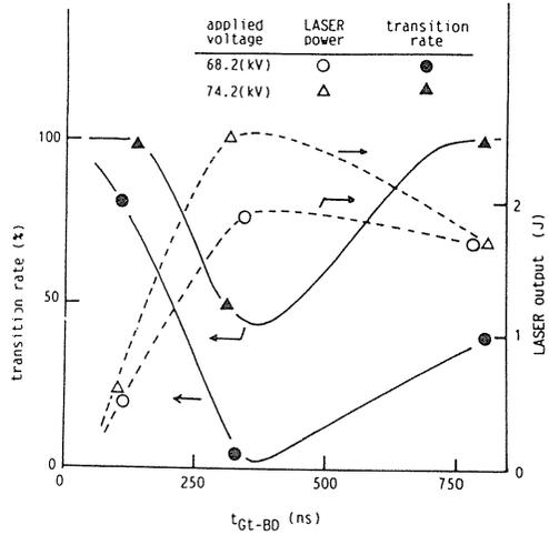
Fig. 7 Transition rate and laser output versus delay time  $t_{Gt-BD}$  for various applied voltage.
