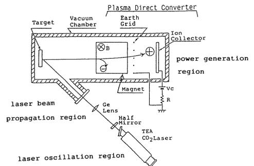
Fig. 32 Energy conversion system from laser beam to electricity by magnetic separation type PDC.
