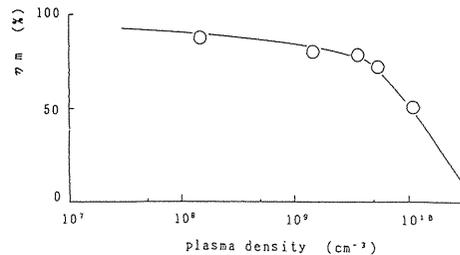
Fig. 34 Percent of magnetic separation as a function of plasma density.
