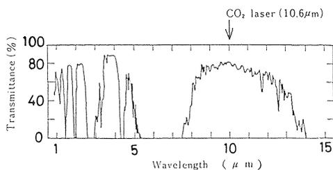
Fig. 3 Wavelength dependence of the transmittance of laser beam in the atmosphere.
