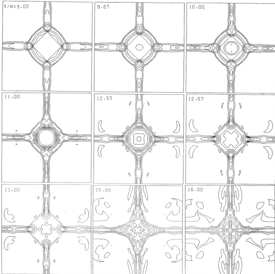
Fig. 9b Density contour in the cross sections at different location on the  $x$  axis for four orifices: downstream of the Mach disk.
