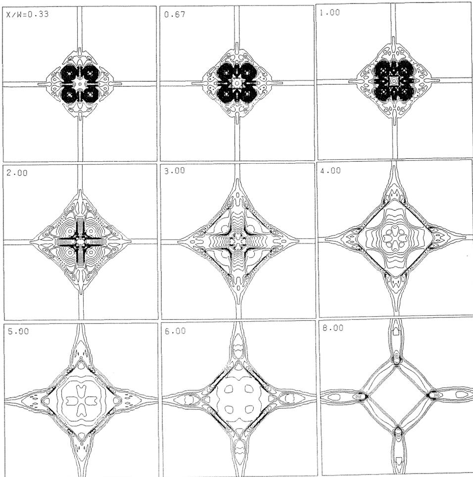
Fig. 9a Density contour in the cross sections at different location on the x axis for four orifices: upstream of the Mach disk.
