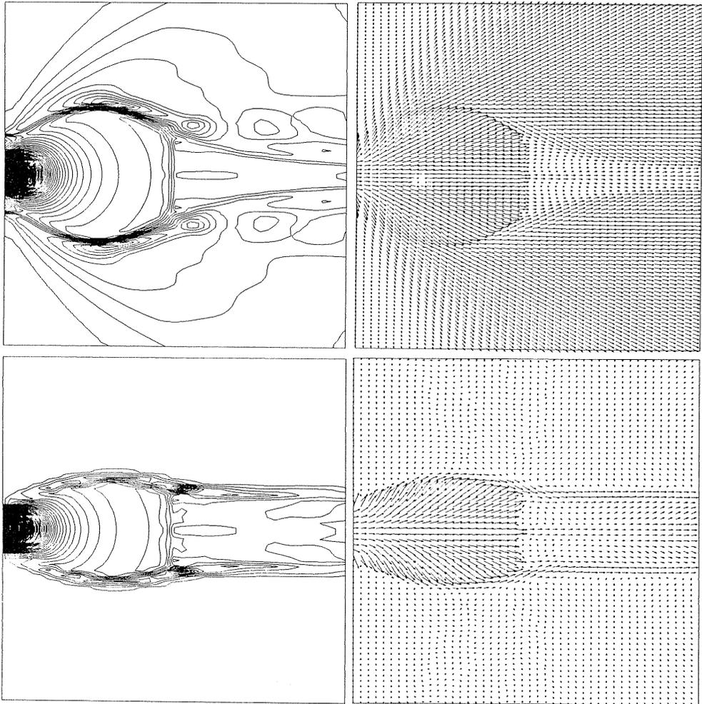
Fig. 2 Density contour (left) and velocity vectors (right) in the symmetric plane ( $z = 0$ ) (upper) and in the orthogonal plane ( $y = z$ ) (lower) for single orifice.
