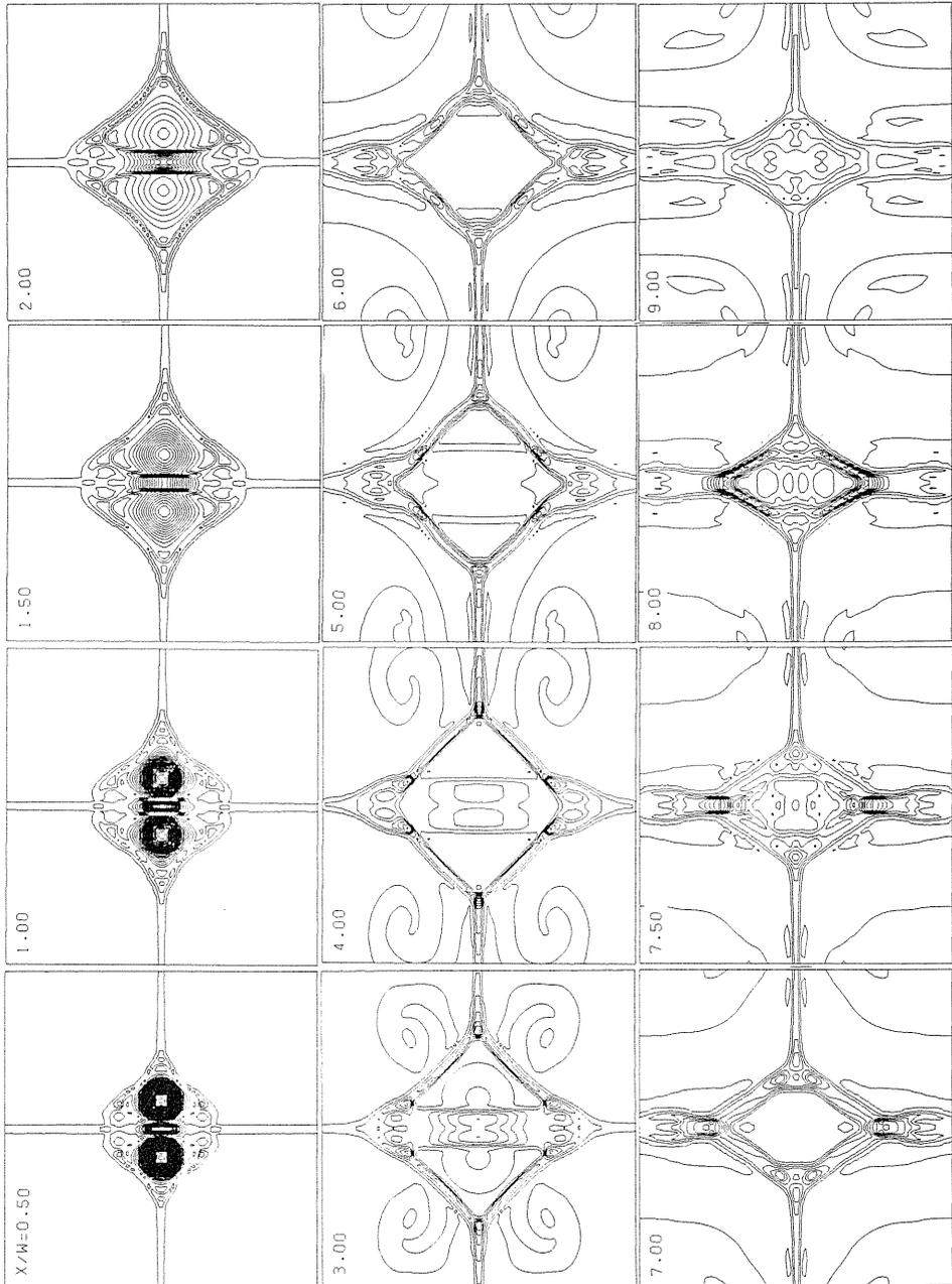
Fig. 6 Density contour in the cross sections at different location on the x axis for two orifices.
