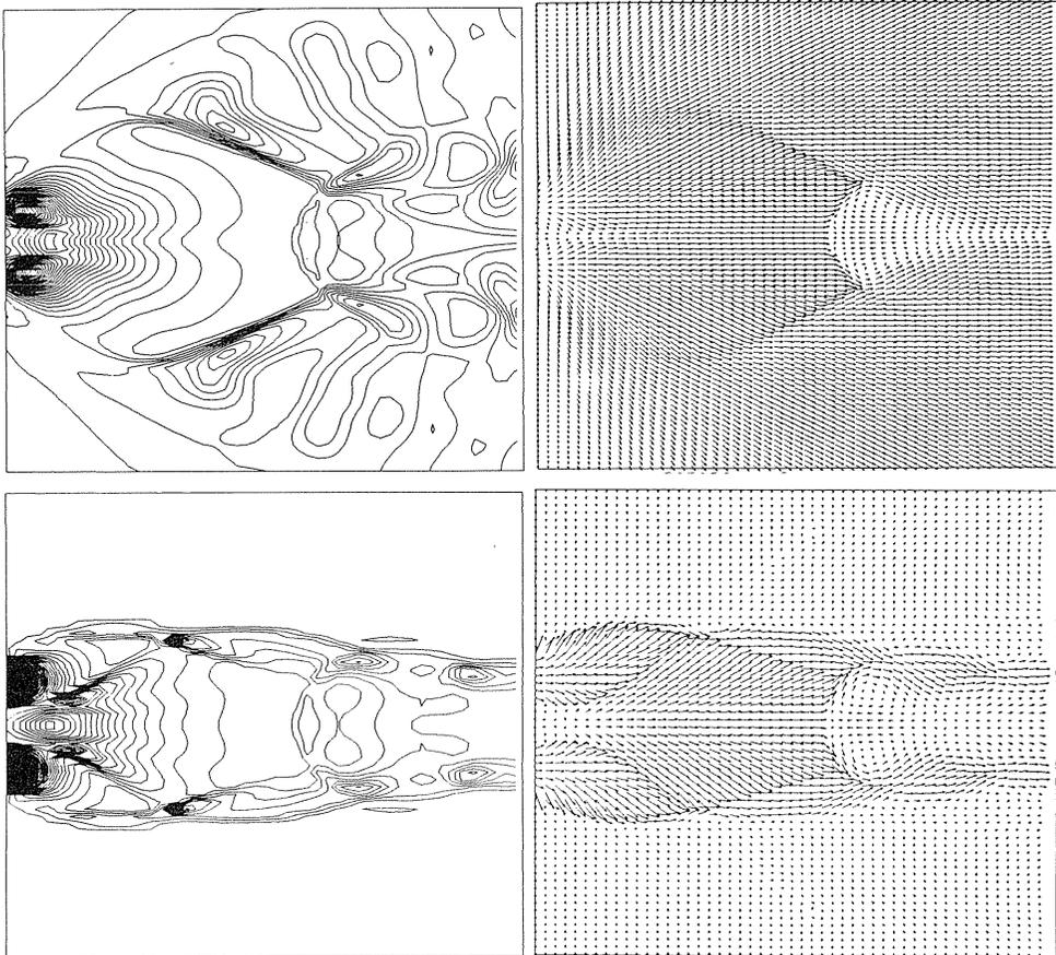
Fig. 8 Density contour (left) and velocity vectors (right) in the symmetric plane,  $z = 0$  (upper) and in the orthogonal plane  $y = z$  (lower) for four orifices.
