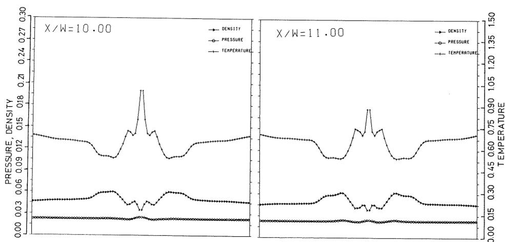
Fig. 4 Distributions of pressure, temperature, and density along the line in the cross section in Fig. 3 and  $y = 0$  for single orifices.
