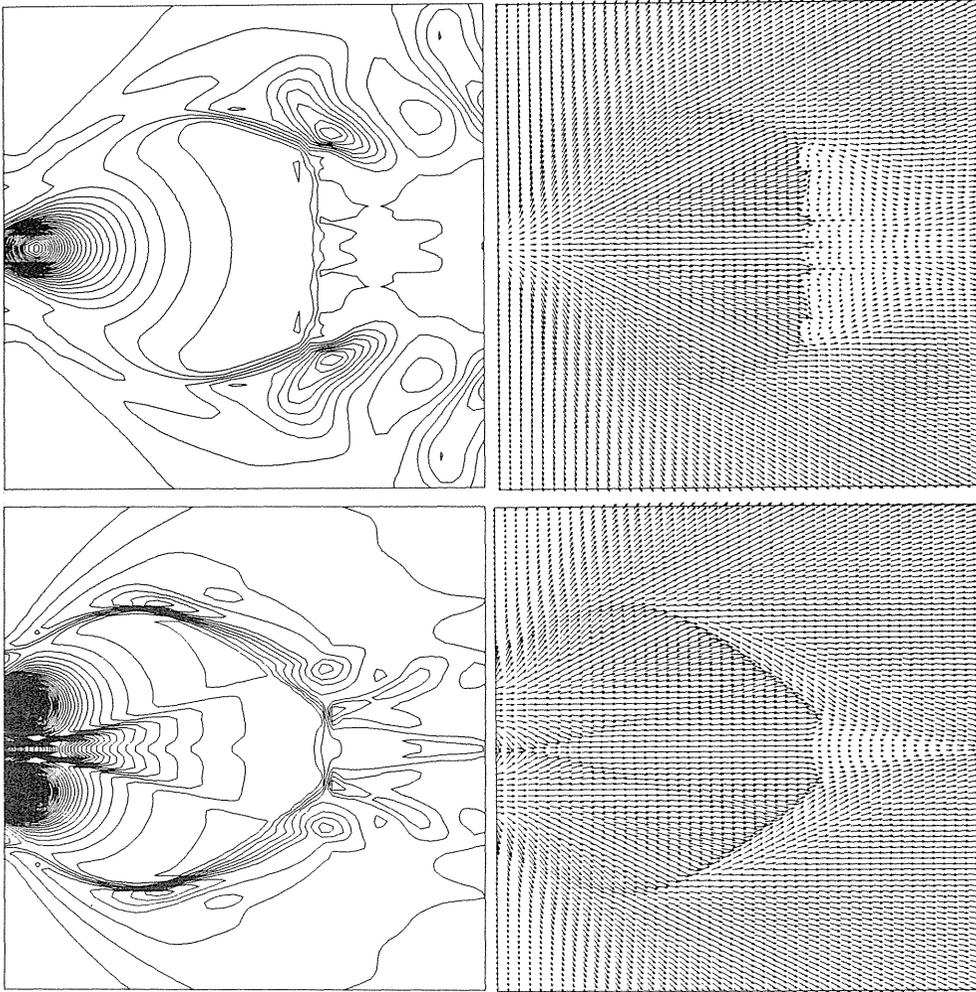
Fig. 5 Density contour (left) and velocity vectors (right) in the symmetric planes,  $z = 0$  (upper) and  $y = 0$  (lower) for two orifices.
