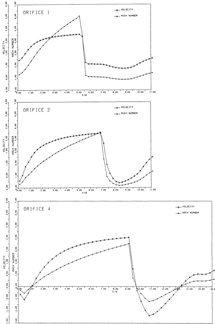
Fig. 10 Distributions of velocity and Mach number along the line symmetry ( $y = z = 0$ ).
