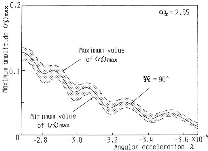
Fig. 5.5. Variations of the maximum amplitude with respect to the angular acceleration  $\lambda$  (deceleration)
