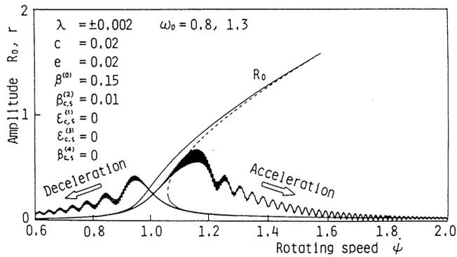
Fig. 3.9. Influence of the nonlinear component  $N(2)$  on the wave of the nonstationary oscillation
