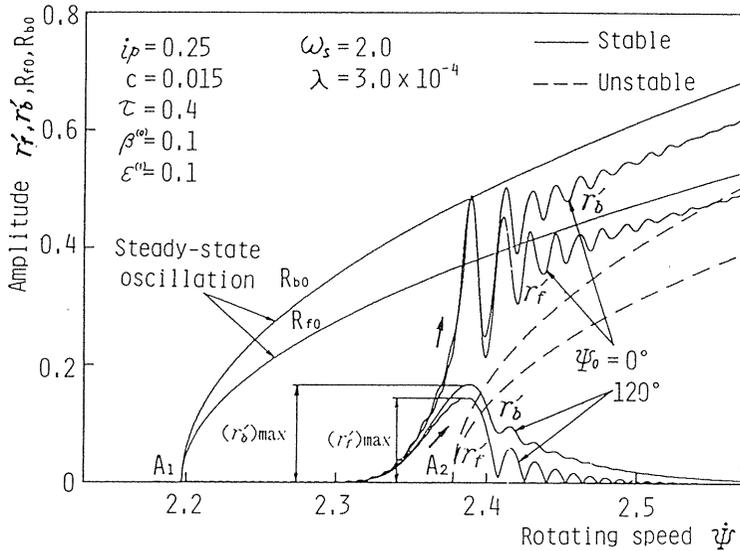
Fig. 5.3. Amplitude variations during acceleration through a critical speed for two different initial angular positions  $\Psi_0$  (acceleration)
