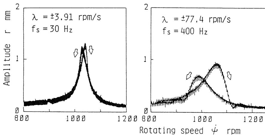
Fig. 3.15. Amplitude change during the passage through the major critical speed (a linear system)
