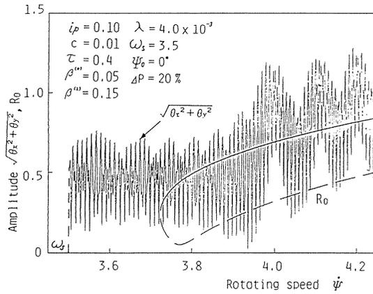
(a) Resonance curves and an amplitude variation curve in a nonstationary oscillation
