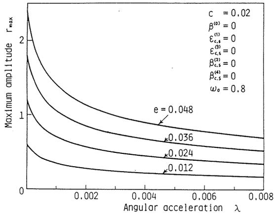
Fig. 3.7. Influence of the magnitude of the unbalance  $e$  on the  $r_{\max}$ - $\lambda$  curve (a linear system)
