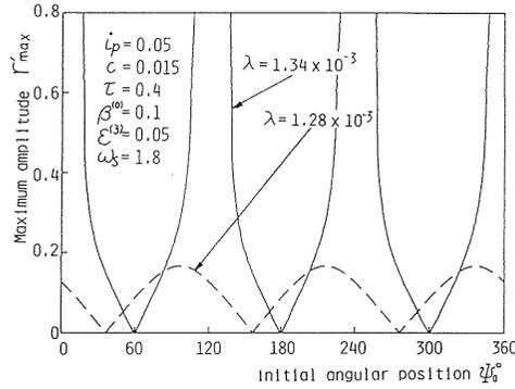
Fig. 6.6. Influence of the initial angular position  $\Psi_0$  on the maximum amplitude  $r'_{max}$  (A  $-1/2$  order subharmonic oscillation)
