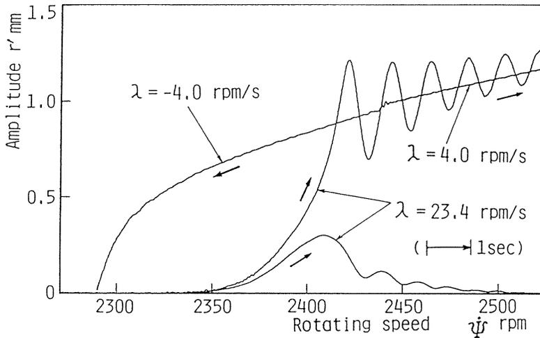
Fig. 4.12. Amplitude variations of subharmonic oscillation during acceleration in experiments
