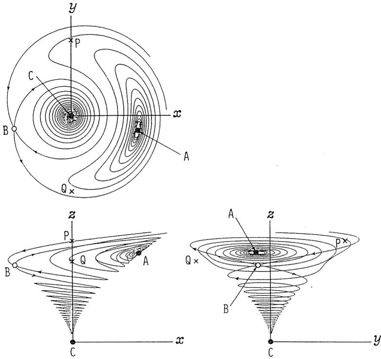
(a) Orthogonal projections of the trajectories passing through the saddle point B
