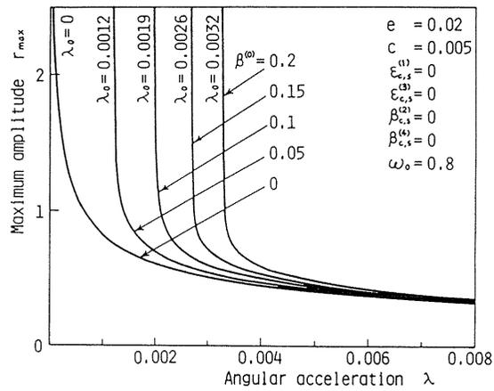
Fig. 3.8. Influence of the coefficient of nonlinear term  $\beta^{(0)}$  on the  $r_{\max}$ - $\lambda$  curve
