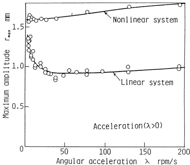
Fig. 3.13. Changes in the maximum amplitude  $r_{max}$  for angular acceleration  $\lambda$
