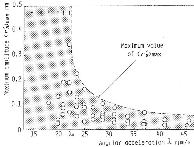
Fig. 5.10. Influence of the angular acceleration on the maximum amplitude (experimental results, acceleration)
