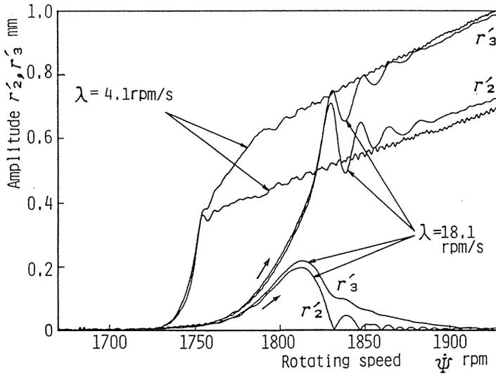
Fig. 5.9. Amplitude variations of the summed-and-differential harmonic oscillation during acceleration (experimental results): a case with a very slow acceleration and cases with the same acceleration but with different initial angular positions
