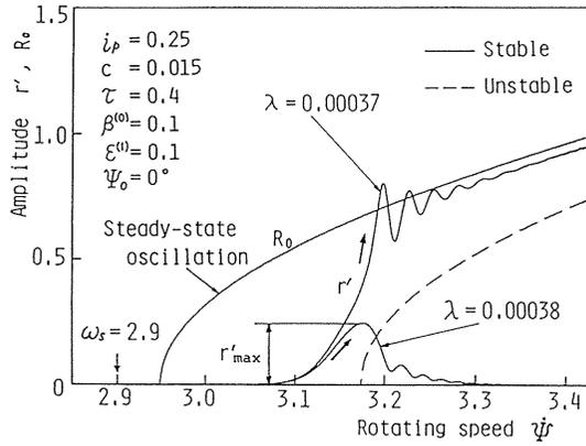
Fig. 4.4. Amplitude variation curve during acceleration through a critical speed
