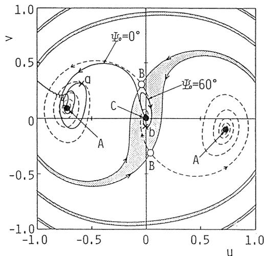
Fig. 4.7. Trajectories on the  $uv$ -plane and separatrices
