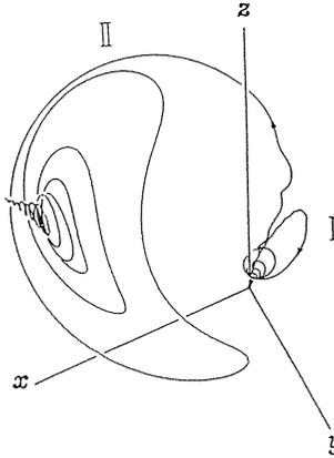
Fig. 5.7. Trajectories in the phase space corresponding to the nonstationary response during acceleration
