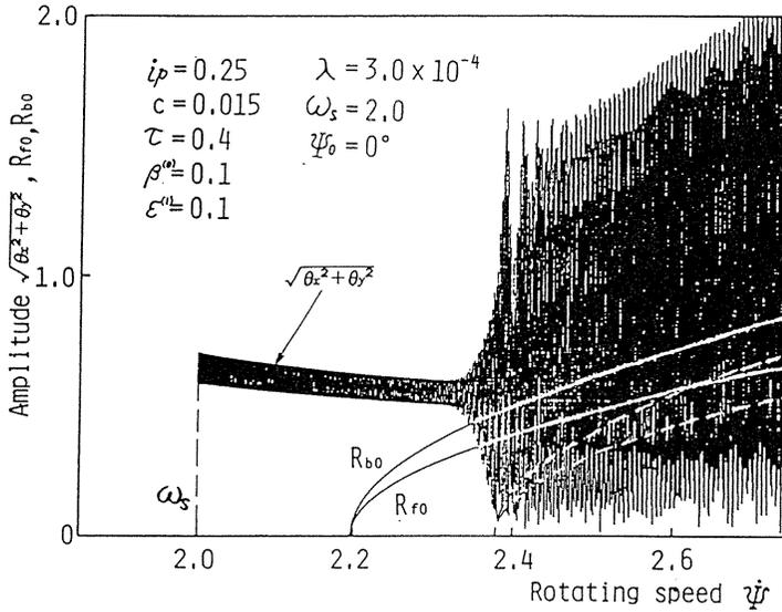
(a) Radius variation obtained by a numerical integration and the amplitudes of the steady-state resonance curve
