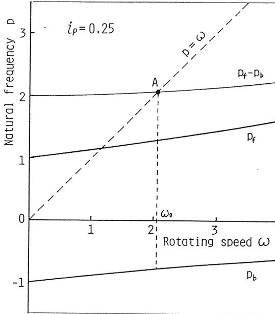
Fig. 5.1. Natural frequency  $p$  as a function of the rotating speed  $\omega$
