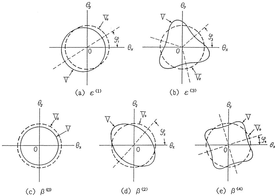
Fig. 2.3. Equipotential lines of each nonlinear component
