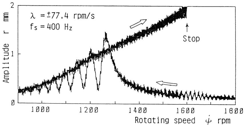
Fig. 3.14. Amplitude change during the passage through the major critical speed (comparatively large unbalance, nonlinear system)
