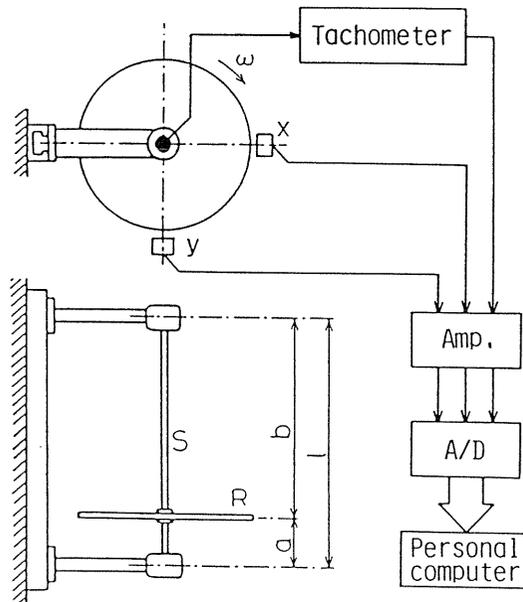
Fig. 4.9. Experimental apparatus and measurement system
