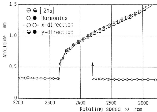
Fig. 4.10. Resonance curve of the subharmonic oscillation in an experiment
