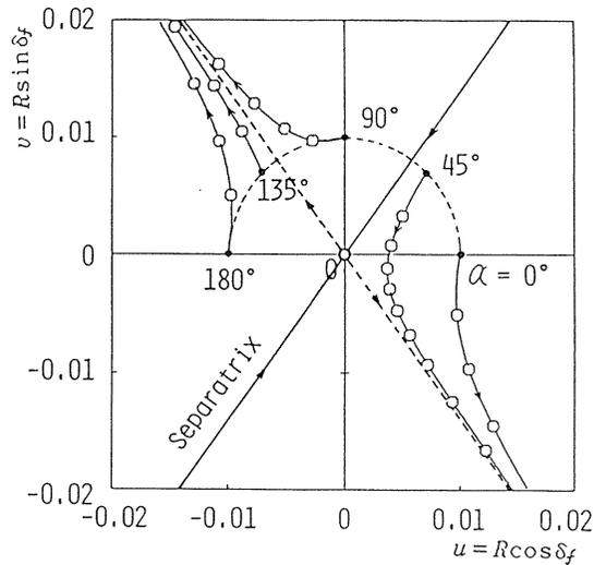
Fig. 4.8. Variation of trajectory due to initial position (a case of constant rotating speed)
