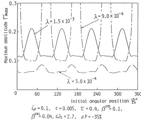
Fig. 6.7. Influence of the initial angular position  $\Psi_0$  on the maximum amplitude  $r'_{max}$  (A  $-1/3$  order subharmonic oscillation)
