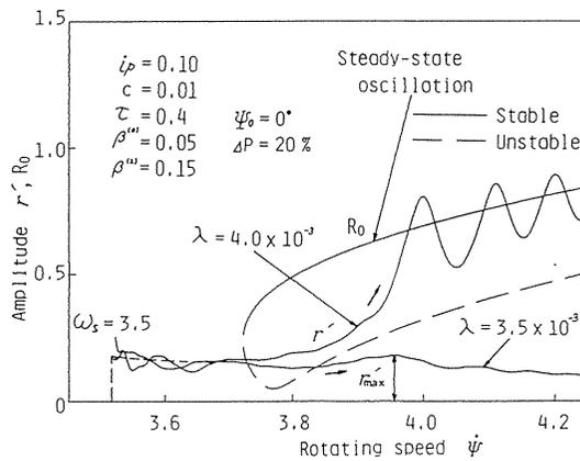
Fig. 6.3. Resonance curves and an amplitude variation curve in a nonstationary oscillation (after signal processing)
