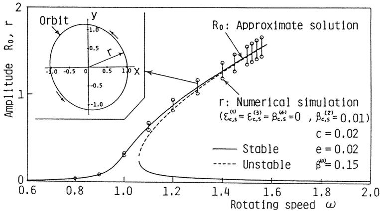
Fig. 3.3. Influence of component  $N(2)$  on the resonance curve
