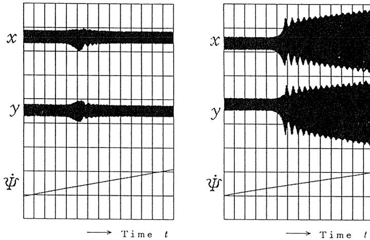
Fig. 4.11. Experimental results of time histories and of angular velocity  $\dot{\Psi}$
