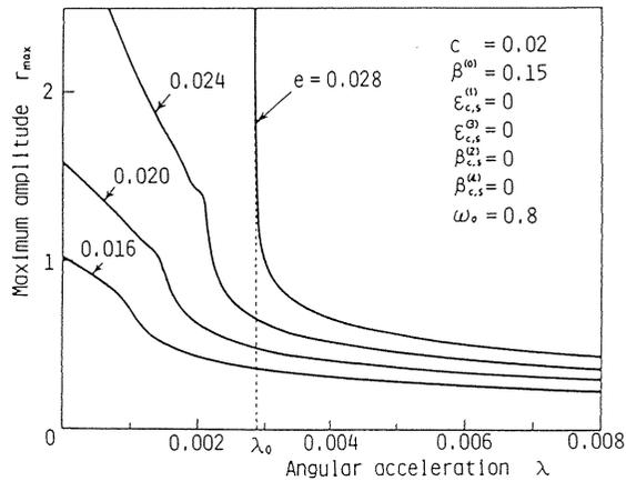
Fig. 3.6. Influence of the magnitude of the unbalance  $e$  on the  $r_{\max}$ - $\lambda$  curve (nonlinear system)
