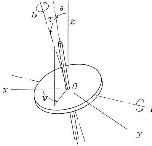
Fig. 4.1. A rotor model and coordinate systems
