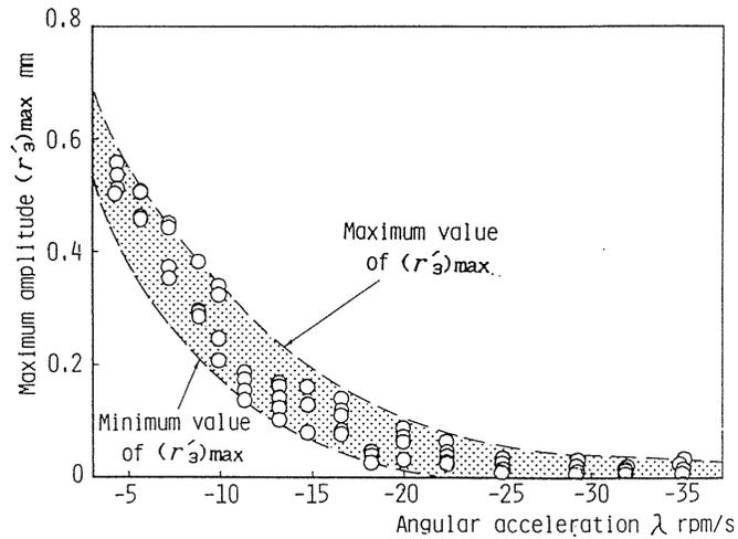
Fig. 5.11. Influence of the angular acceleration on the maximum amplitude (experimental results, deceleration)
