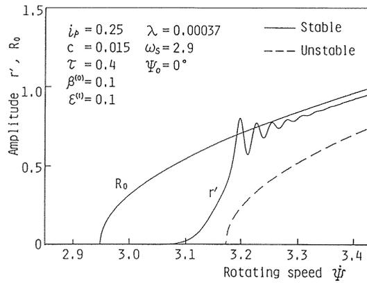
(c) Amplitude variation curve of subharmonic oscillation after data processing
