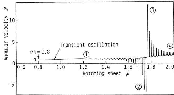
(b) Change in the angular velocity of whirling motion  $\dot{\psi}$
