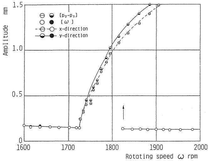
Fig. 5.8. Steady-state resonance curve of the summed-and-differential harmonic oscillation (experimental result)
