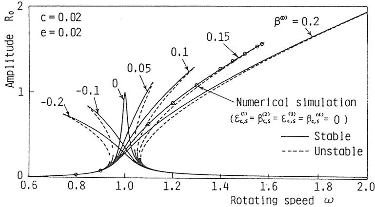
Fig. 3.2. Influence of component  $N(0)$  on the resonance curve
