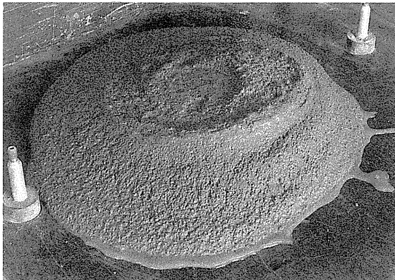
Photo. 1. Slump test of mortar.
