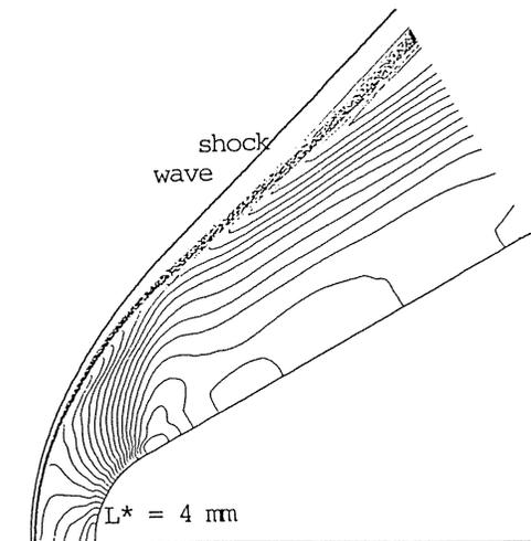
Fig. 3. Contours of  $H_2O$  density for  $L^* = 4.0$  mm,  $M_\infty = 6$  and  $\theta = 30$  degree.
