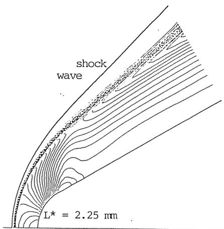
Fig. 2 (a) Contours of  $H_2O$  density for  $L^* = 2.25$  mm,  $M_\infty = 6$  and  $\theta = 30$  degree.
