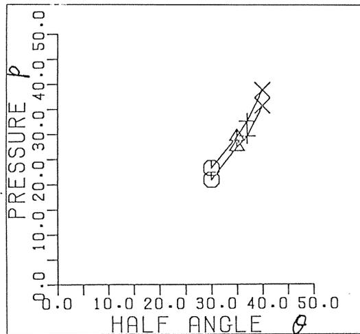
Fig. 5. A polar curve  $p$ - $\theta$  relation to SOD for  $M_\infty = 6$  and  $L^* = 3$  mm.
