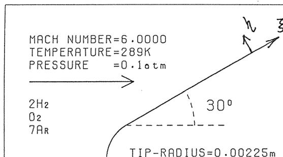
Fig. 1. Geometry of 2-D blunted wedge.
