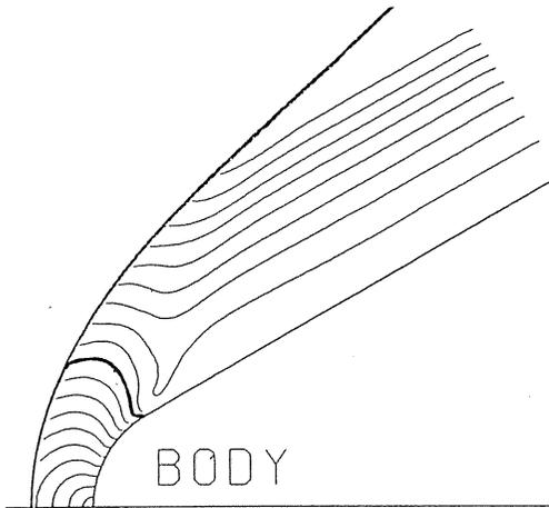
Fig. 4 (a) Sonic locus in shock layer for  $\theta = 30$  degrees.
