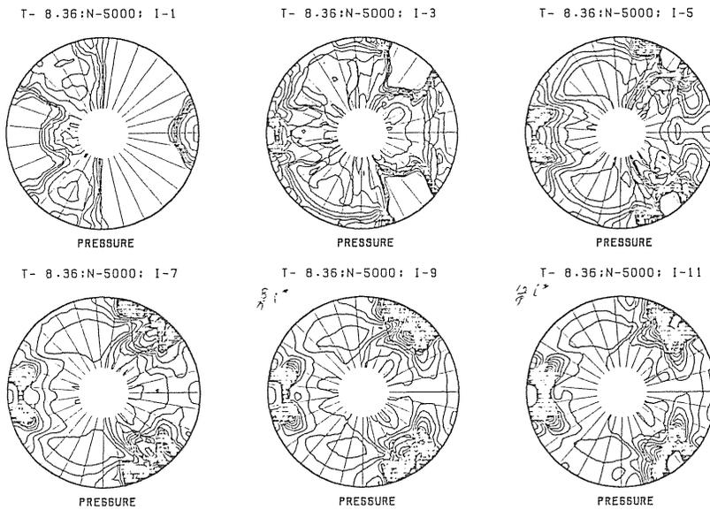
Fig. 4 (b) Pressure distributions in the cross sections of a tube of outer radius  $22L^*/9$  and inner radius  $4L^*/9$  at Time Step 5000;  $I = 1 - 11$ , corresponding to  $z = (I - 1)L^*/9$ .
