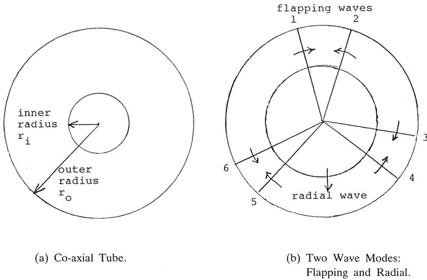
Fig. 1. Tube geometry and the concept of “flapping” and “radial” waves propagating in the azimuthal and radial directions of tube cross section.
