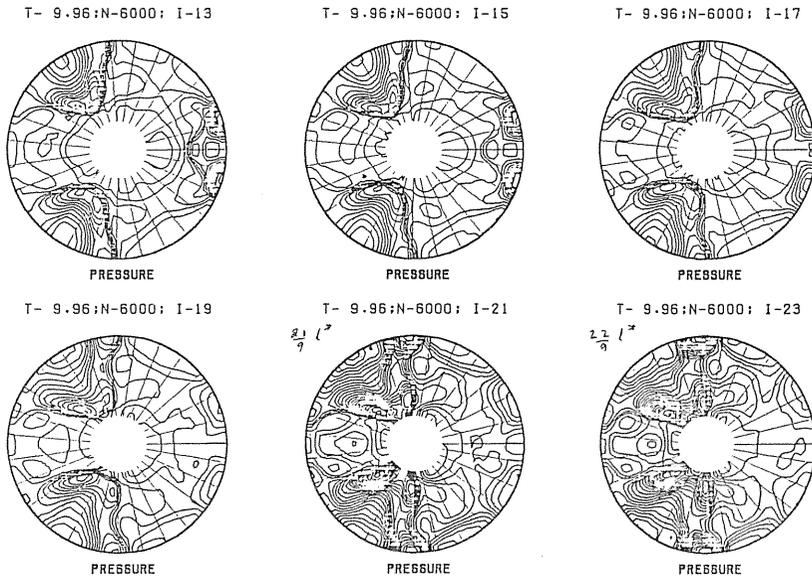
Fig. 5 (d) Pressure distributions in the cross sections of a tube of outer radius  $22L^*/9$  and inner radius  $4L^*/9$  at Time Step 6000; the cross sections  $I=13-23$ , corresponding to  $z=(I-1)L^*/9$ .
