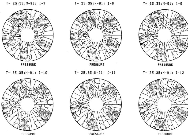
Fig. 6 (b) Pressure distributions in the cross sections  $I=7-12$  of a tube of outer radius  $46L^*/9$  and inner radius  $10L^*/9$  at Time Step 7000.
