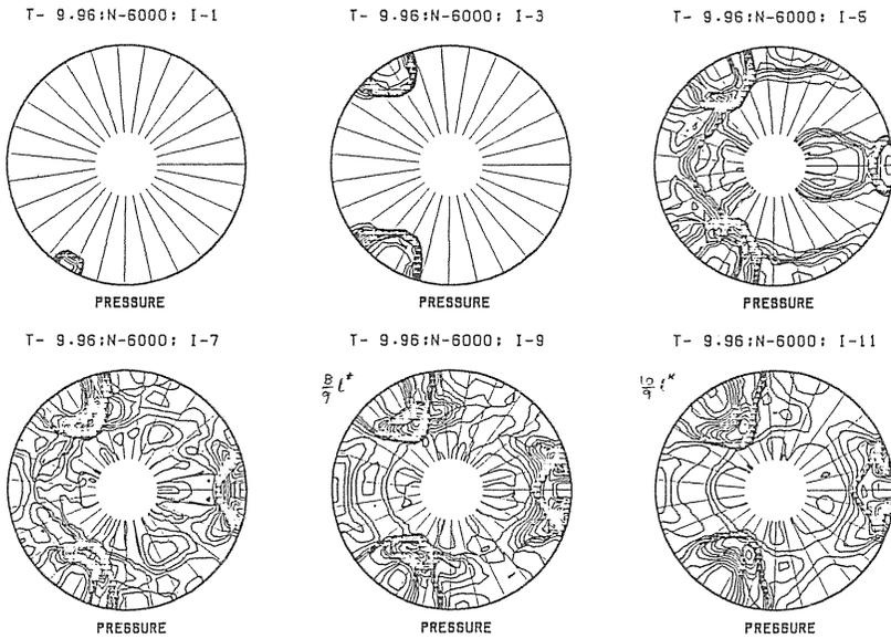
Fig. 5 (c) Pressure distributions in the cross sections of a tube of outer radius  $22L^*/9$  and inner radius  $4L^*/9$  at Time Step 6000; the cross sections  $I=1-11$ , corresponding to  $z=(I-1)L^*/9$ .
