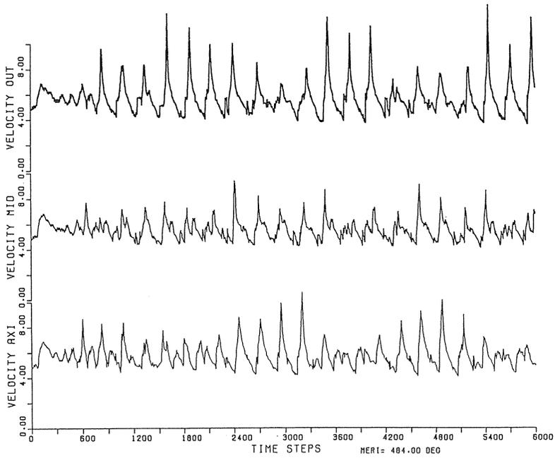
Fig. 3 (c) Propagation velocity of the detonation front at three different radii in the meridian plane  $\phi=235.51$  degree.
