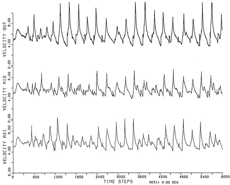
Fig. 3 (a) Propagation velocity of the detonation front at three different radii in the meridian plane  $\phi=0$  degree: A detonation in a tube of outer radius  $22L^*/9$  and inner radius  $4L^*/9$  at Time Step 5000. Total grids are  $450 \times 21 \times 110$ , based upon the uniform grid spacing  $L^*/9$ , giving the azimuthal angle interval 3.36 degrees.
