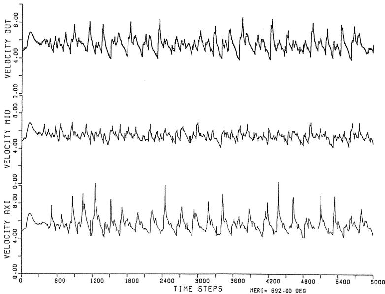
Fig. 3 (b) Propagation velocity of the detonation front at three different radii in the meridian plane  $\phi=33.64$  degree.
