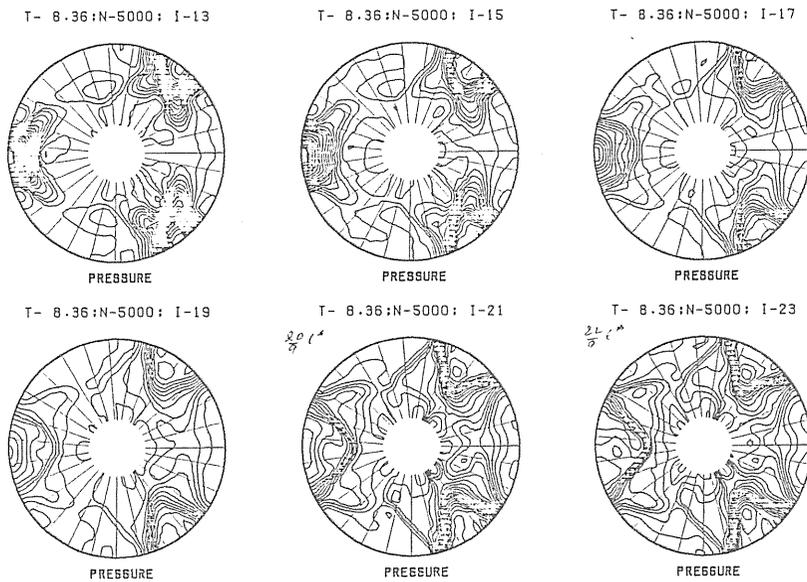
Fig. 4 (c) Pressure distributions in the cross sections of a tube of outer radius  $22L^*/9$  and inner radius  $4L^*/9$  at Time Step 5000;  $I = 13 - 23$ , corresponding to  $z = (I - 1)L^*/9$ .
