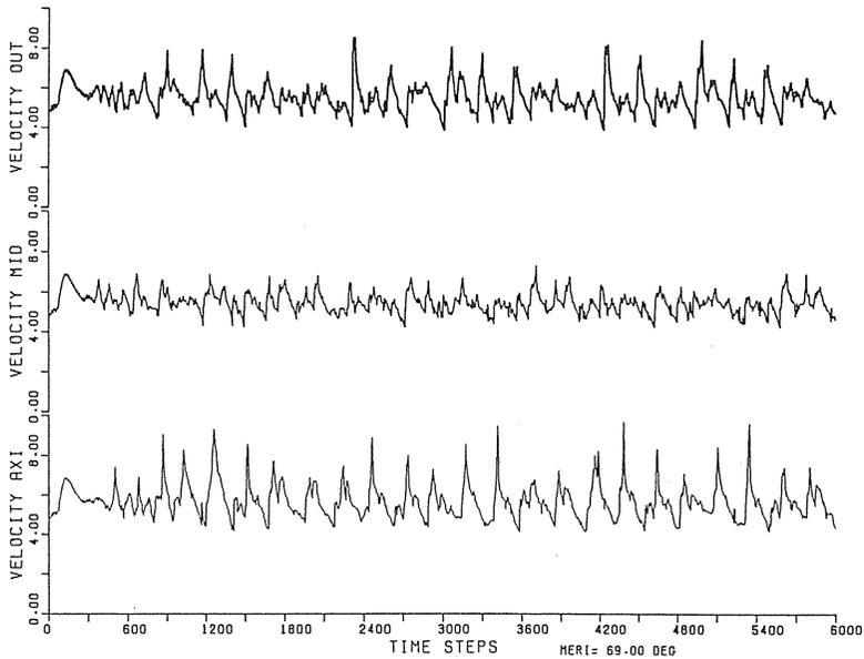
Fig. 3 (e) Propagation velocity of the detonation front at three different radii in the meridian plane  $\phi=336.45$  degree.
