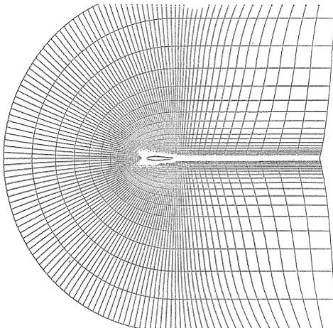
Fig. 1. Grid system used to analyze the NACA 0012 airfoil.
