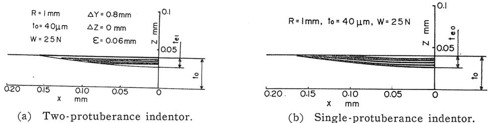
Fig. 38. Plastic flow lines (side view in case of  $W=25\text{N}$ ).
