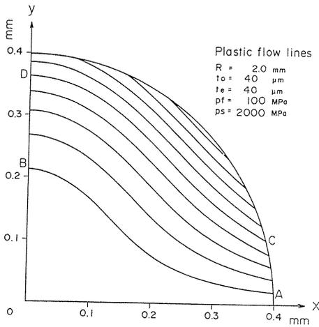
(a) x-y projection of plastic flow lines.
