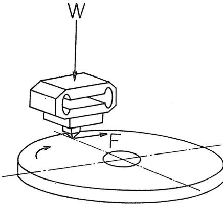
Fig. 2. Sketch of single protuberance slider on flat soft metal film.
