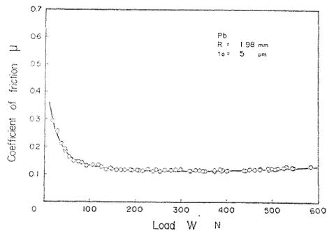
Fig. 5. Relation between coefficient of friction  $\mu$  and load  $W$  (Pb-electroplated film, sphere radius 1.98 mm).
