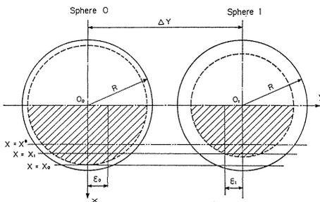
Fig. 28. Arrangement of two-protuberance indenter (top view).
