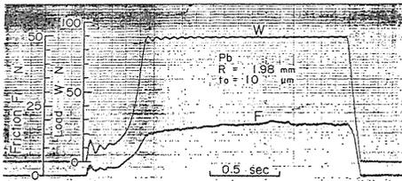
Fig. 4. Experimental record of applied load  $W$  and friction force  $F$ .
