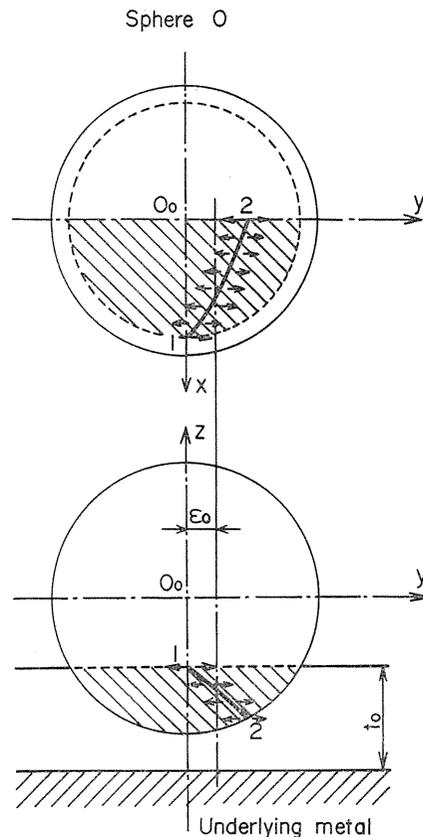
Fig. 30. Location of bifurcation in film flow direction.
