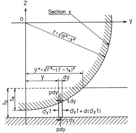
Fig. 16. Compression under plane strain.
