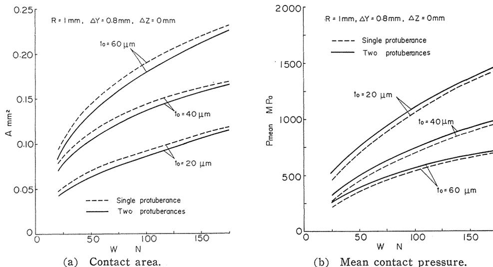
Fig. 44. Contacting state of indenter and soft metal film when film thickness  $t_0$  is varied.
