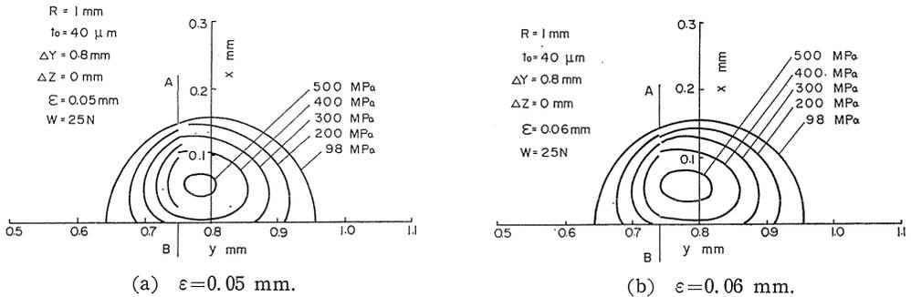
Fig. 34. Relation between bifurcation location and contact pressure distribution.
