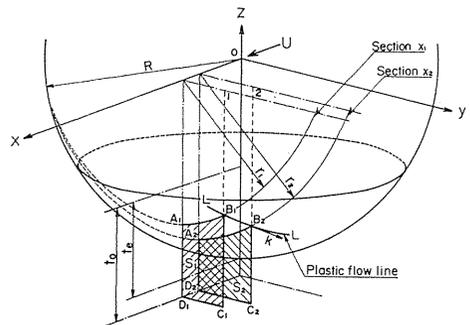
Fig. 27. Plastic flow of metal film between spherical protuberance and underlying metal.
