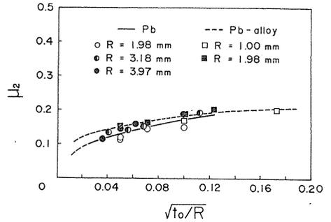
Fig. 10. Relation between minimum coefficient of friction  $\mu_2$  and  $\sqrt{t_0/R}$ .
