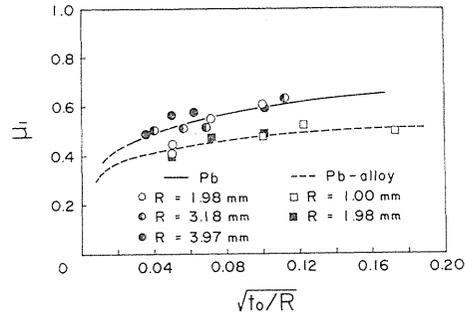
Fig. 12. Relation between coefficient of friction  $\mu_1$  when  $W=0$  and  $\sqrt{t_0/R}$ .
