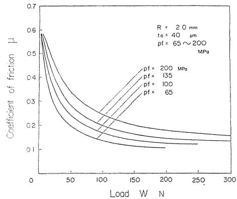
Fig. 22. Effect of deformation resistance  $p_f$  of film on coefficient of friction  $\mu$ .
