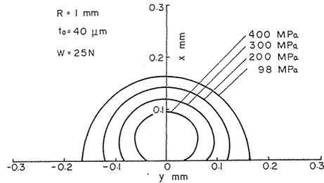
Fig. 39. Contact pressure distribution (single-protuberance indenter,  $W=25\text{ N}$ ).
