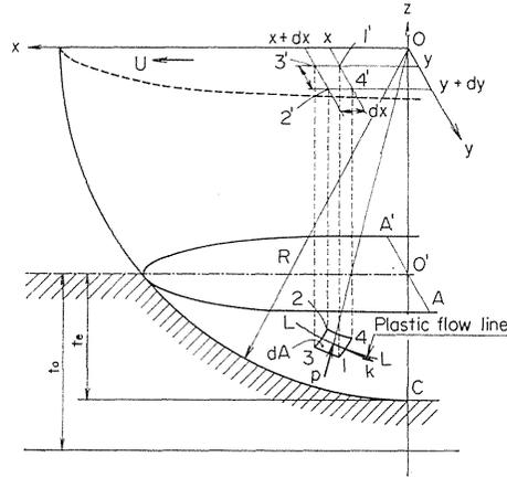
Fig. 17. Stress distribution on spherical protuberance.
