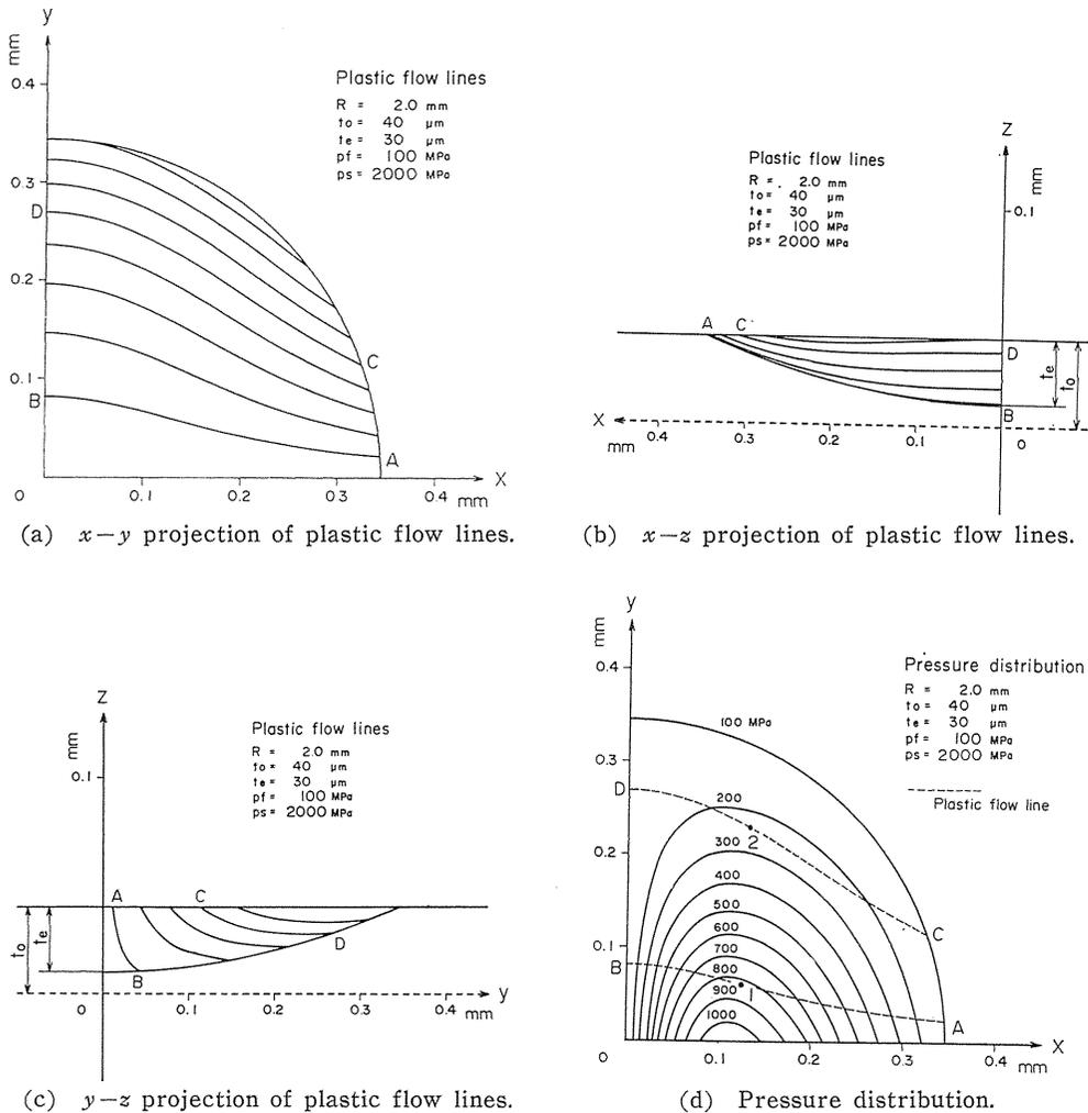
Fig. 18. Plastic flow lines and pressure distribution ( $t_e < t_0$ ).
