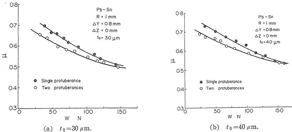
Fig. 26. Relation between coefficient of friction  $\mu$  and normal load  $W$ .
