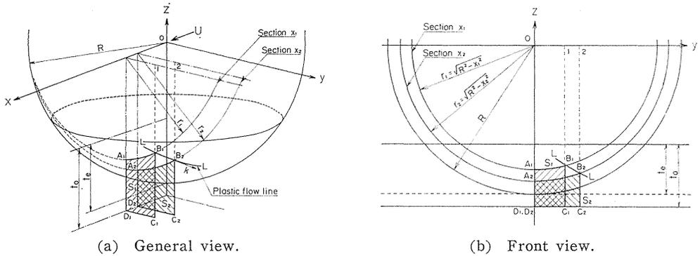
Fig. 15. Contact model of spherical protuberance and surface.
