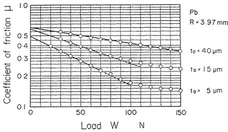
Fig. 11. Relation between coefficient of friction  $\mu$  and load  $W$  (semi-log plotting).
