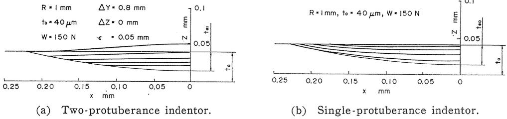
Fig. 41. Plastic flow lines (side view in case of  $W=150 \text{ N}$ ).
