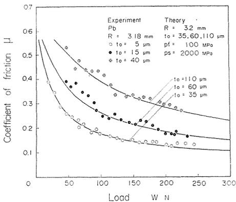
(b) Pb-electroplated film,  $R=3.18$  mm.
