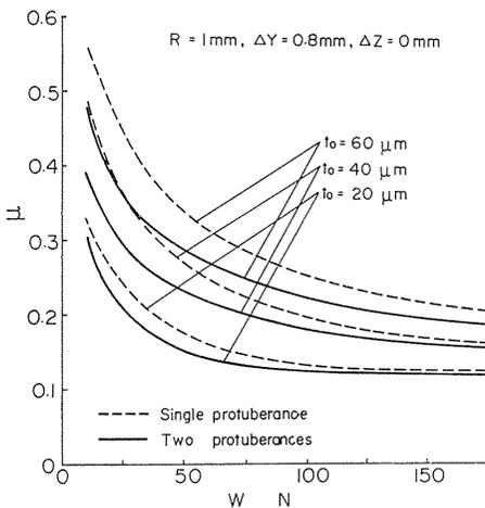
Fig. 43. Relation between coefficient of friction  $\mu$  and normal load  $W$  (calculational result when film thickness  $t_0$  is varied).
