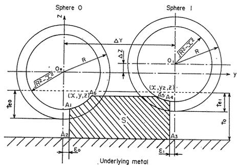
Fig. 29. Arrangement of two-protuberance indenter (front view) and deformation of soft metal film under interference effect.
