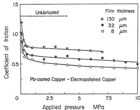
Fig. 1. Coefficient of friction vs. applied pressure for various lead film thickness [Tsuya and Takagi].
