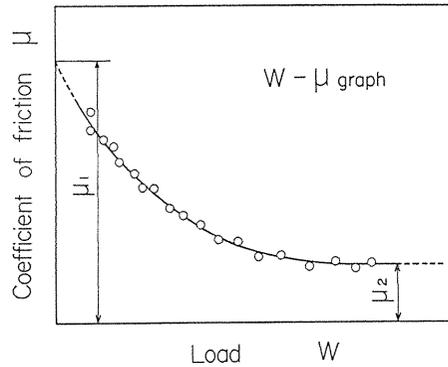
Fig. 8. Arrangement of experimental  $\mu$ - $W$  relation.
