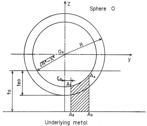
Fig. 31. Soft metal film deformation on non-interference effect side.
