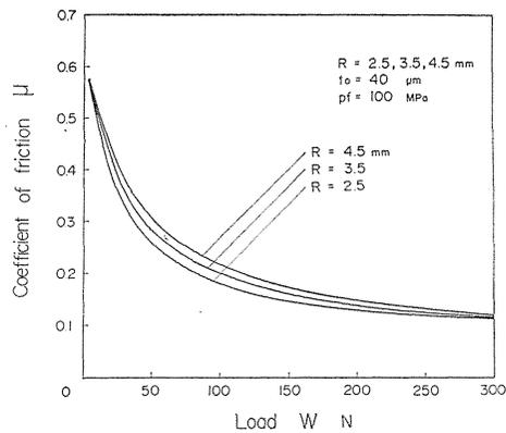
Fig. 20. Effect of radius of spherical protuberance  $R$  on coefficient of friction  $\mu$  ( $p_f=100$  MPa,  $k_f=p_f/\sqrt{3}$ ).
