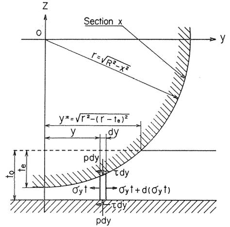
Fig. 32. Compression deformation under plane strain.
