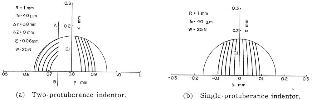
Fig. 37. Plastic flow lines (top view in case of  $W=25\text{N}$ ).
