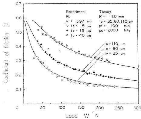
(c) Pb-electroplated film,  $R=3.97$  mm.
