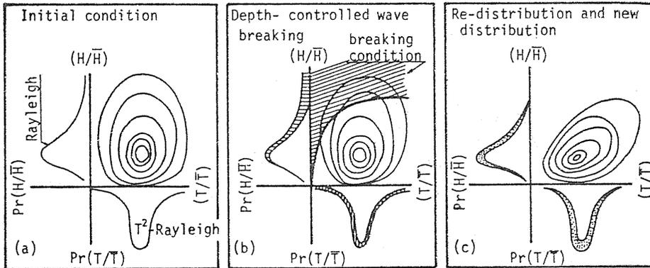
Fig. 36. Schematic illustration of variation of joint probability density of wave heights and periods due to wave breaking.
