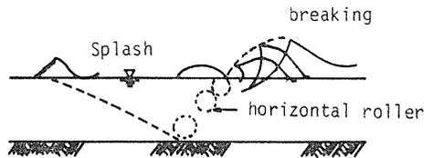
Fig. 14. Schematic illustration of plunging breaker.
