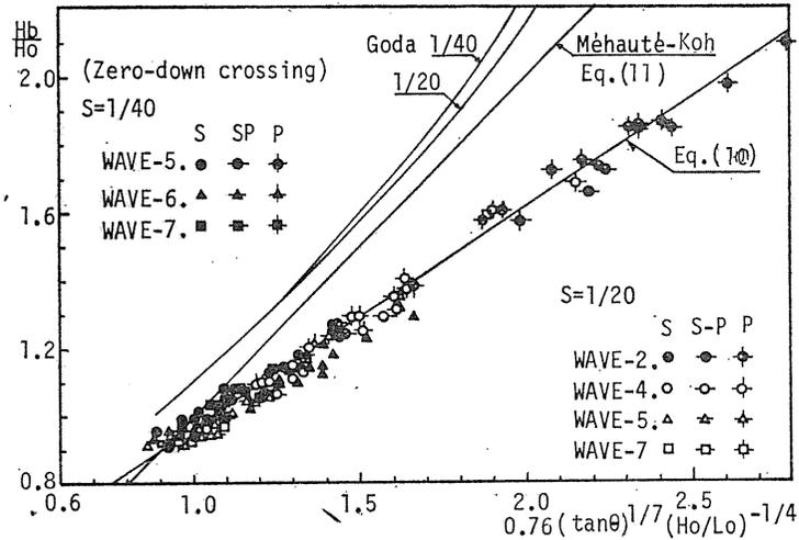
Fig. 13. Relative breaking wave height  $H_b/H_0$  (irregular wave).
