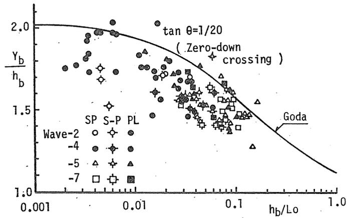
Fig. 10. Relative breaking wave crest height (irregular wave).
