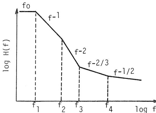
Fig. 27. Schematic illustration of equilibrium spectral slope.
