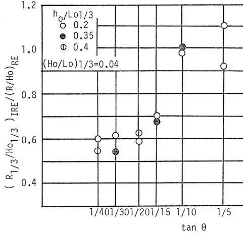
Fig. 42. Comparison between run-up heights of irregular wave and regular wave.
