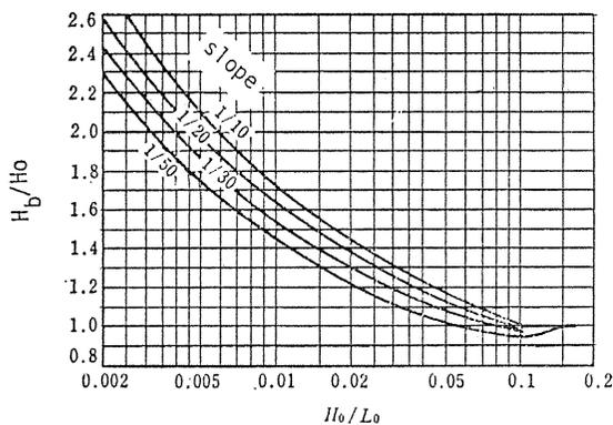
Fig. 5. Variation of breaking wave height (from Goda<sup>27)</sup>).
