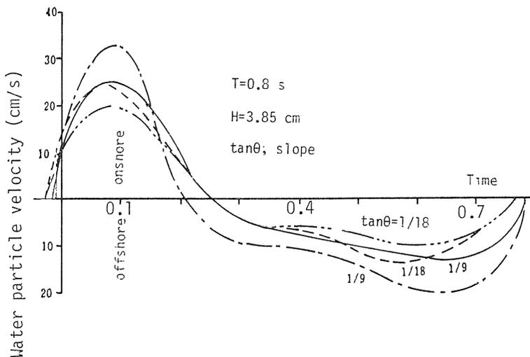
Fig. 7. Time profile of water particle velocity at breaking point (from Kemp<sup>28</sup>).
