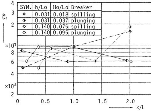
Fig. 23. Changes of coefficient  $\hat{C}_f$  with  $X/L$ .
