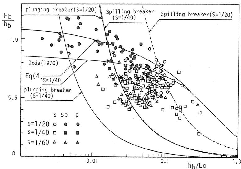
Fig. 9. Relative breaking wave height (irregular wave).
