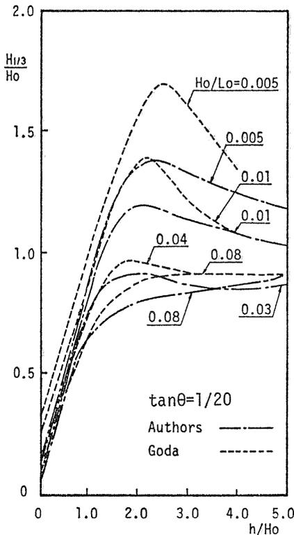
Fig. 37. Calculated values of significant wave height.
