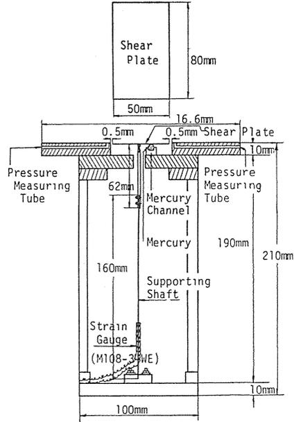
Fig. 20. Schematic view of shear meter.
