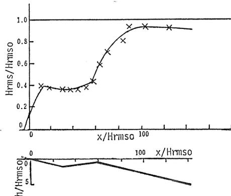
Fig. 35. Comparison between calculated values and experiments (from Battjes<sup>31)</sup>).
