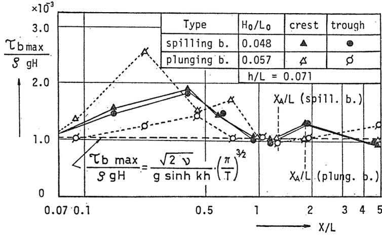
Fig. 22. Examples of relation between  $\tau_{b \max}/\rho g H$  and  $X/L$ .
