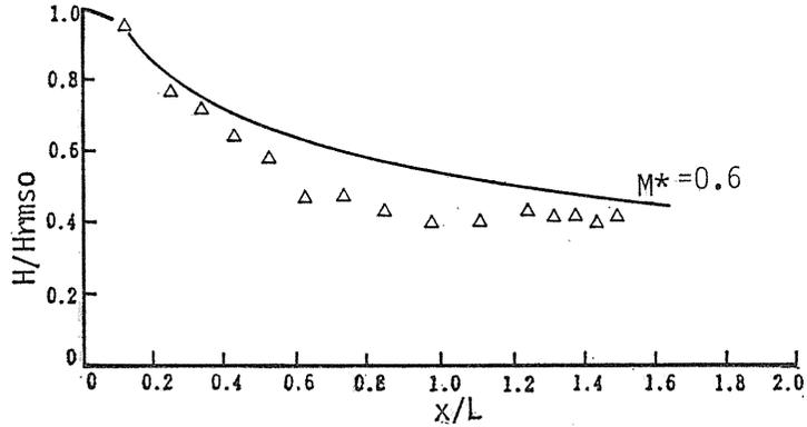
Fig. 33. Comparison between fields measurements and calculated values (from Suhayda<sup>53</sup>).
