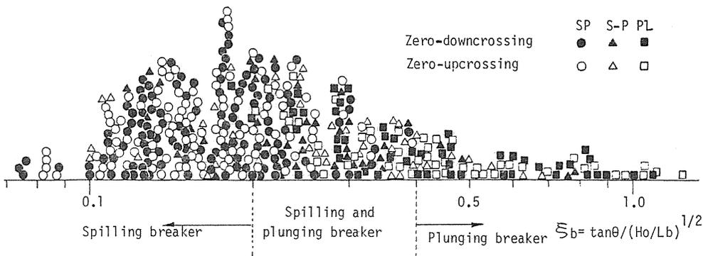
Fig. 3. Breaker type classification due to surf similarity parameter.
