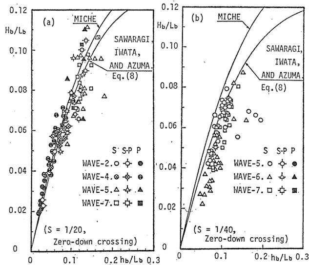
Fig. 11. Breaking wave steepness (irregular wave).
