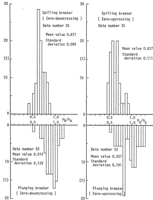
Fig. 8. Frequency of relative breaking wave height.
