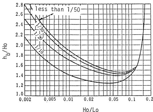
Fig. 4. Variation of breaking water depth (from Goda<sup>27)</sup>).
