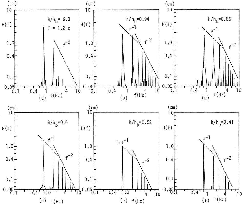
Fig. 28. Variation of wave height spectrum on sloping bed.
