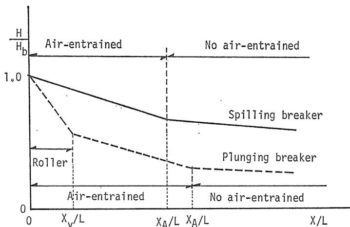
Fig. 15. Schematic illustration of wave height attenuation.
