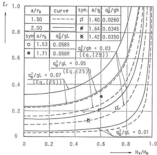
Fig. 19. Energy loss due to horizontal roller.
