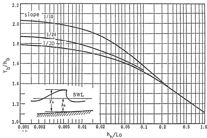
Fig. 6. Variation of breaking wave crest height (from Goda<sup>27</sup>).
