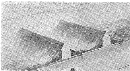
Fig. 7. Deformed Taylor-Görtler type vortices on the surface of the large crest model. R_\infty=1123 . The tow direction is from left to right.
