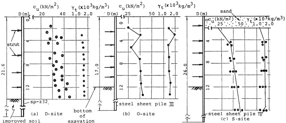
Fig. 4. 6. Ground conditions and location of struts of actual cases.
