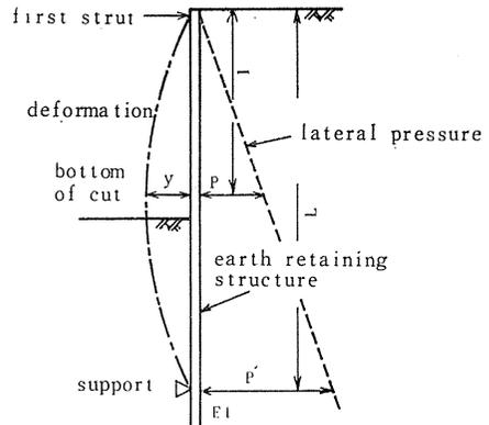
Fig. 4. 8. Deformation of earth retaining structure.
