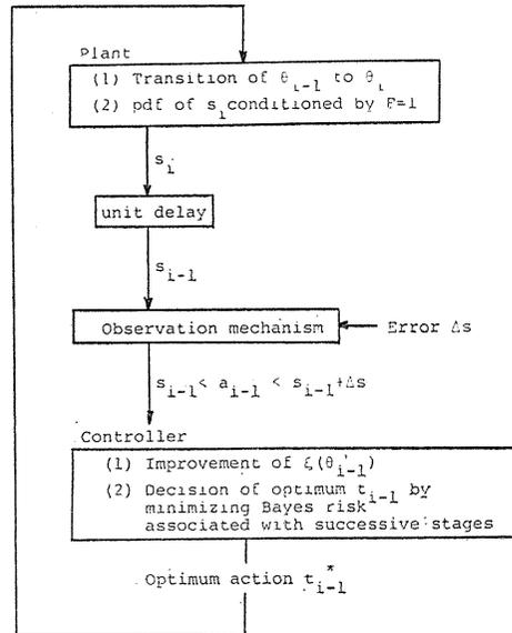
Fig. 3. 2. Optimization scheme of observational procedure.
