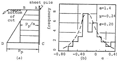
Fig. 4. 3. (a) Modified earth pressure below bottom of cut at open side.
