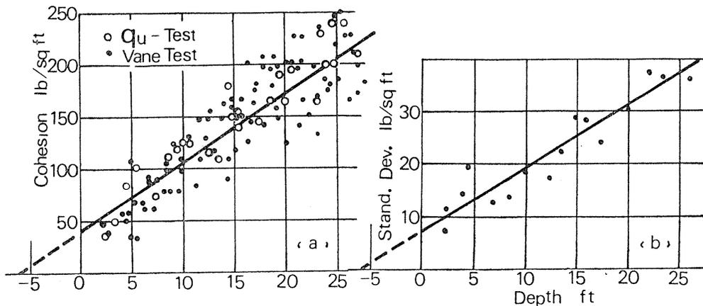
Fig. 2. 5. ( $c_u, \sigma_c \sim z$ ) Relations. (after Lumb)
