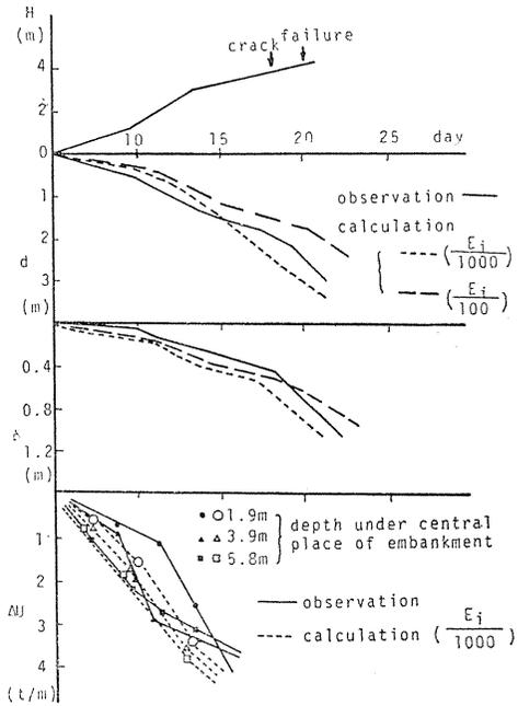
Fig. 3. 10. Progress of  $d$ ,  $\delta$  and  $\Delta u$  at Tsukisappu.
