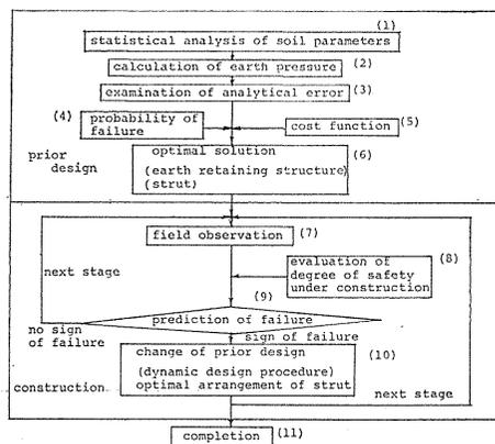
Fig. 4.1. Procedure of design.
