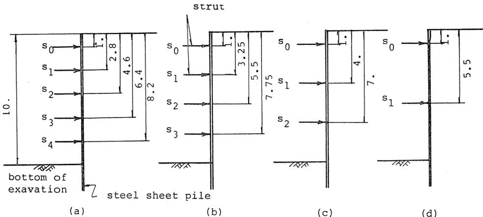
Fig. 4. 5. Arrangement of struts in model (A). (unit; m)
