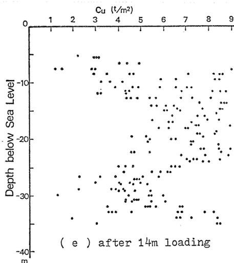
Fig. 2. 8. Relation between  $c_u$  and  $z$ .
