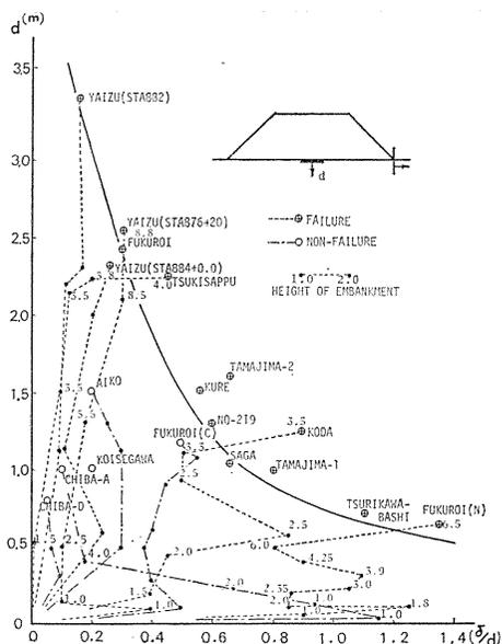
Fig. 3. 3.  $(\delta/d \sim d)$  diagram for prediction of failure.
