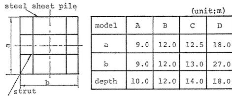
Fig. 4. 4. Excavation field models.
