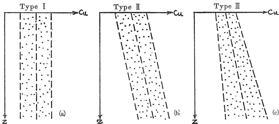
Fig. 2. 1. Typical Types of Distribution of  $c_u$ .
