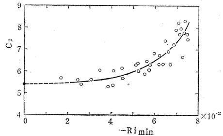
Fig. 4. 21. Change in the value of  $C_2$  in Eq. (4.23) in terms of the minimum value of Richardson number.
