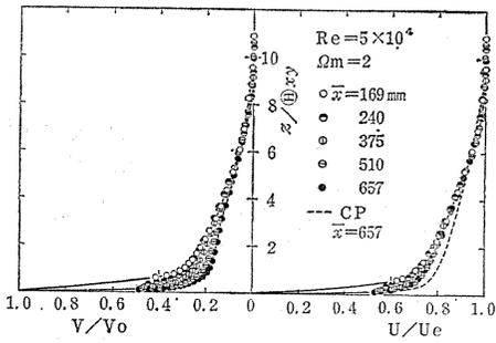
Fig. 4. 4. Velocity profiles in the turbulent boundary layer for AP(II) at  $\Omega_m=2$ .
