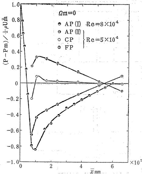
Fig. 4. 2. Static-pressure distribution.
