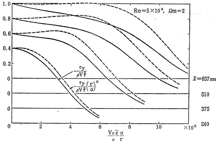
Fig. 4.10. Distribution of peripheral shear stresses in the turbulent boundary layer for CP.
