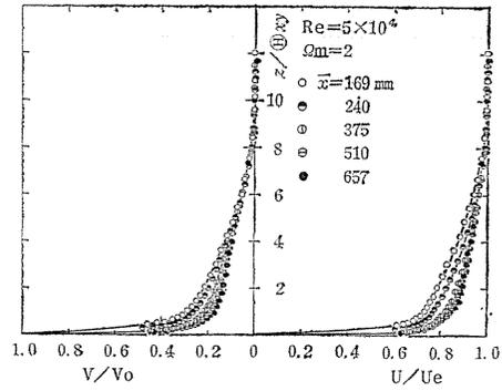
Fig. 4. 5. Velocity profiles in the turbulent boundary layer for FP at  $\Omega_m=2$ .
