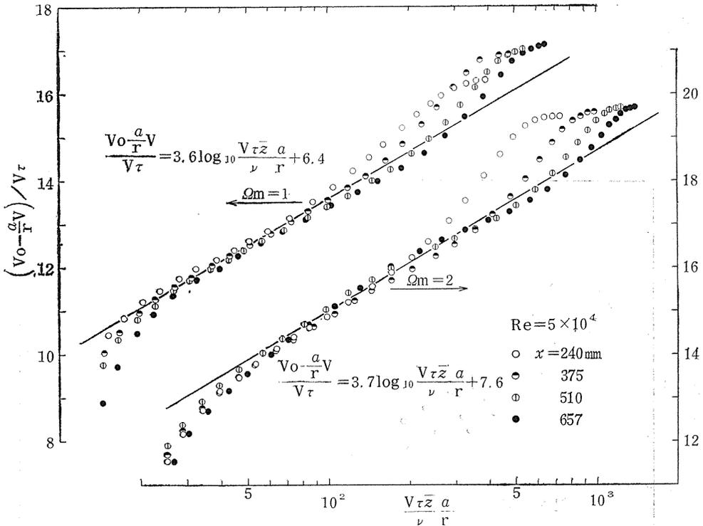
Fig. 4. 13. Logarithmic plots of peripheral velocity profiles for CP on the basis of Eq. (4. 23).
