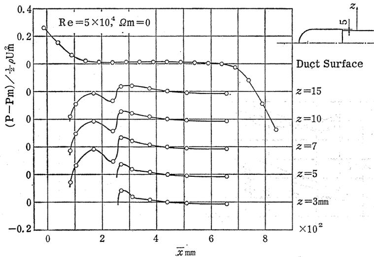
Fig. 3. 11. Pressure distribution in the case of Step.
