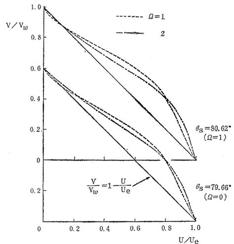
Fig. 2. 4. Variation of polar plots with  $\Omega$  at the each separation point of  $\Omega=0$  and  $\Omega=1$  respectively.
