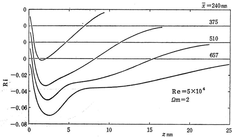
Fig. 4.18. Distribution of Richardson number in the turbulent boundary layer for CP.
