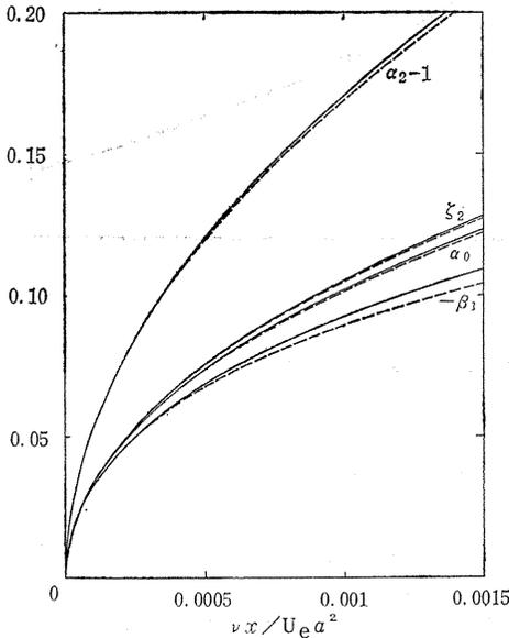
Fig. 2.10. Behavior of various parameters near the origin; solid line represents the numerical results, and dotted line shows the series solution near the origin.
