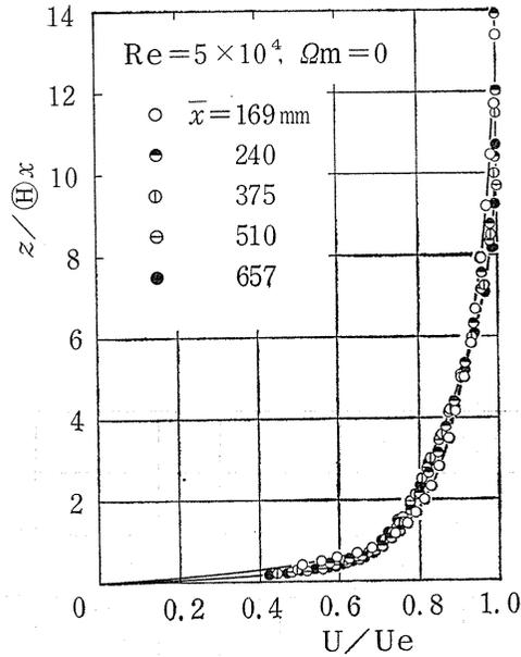
Fig. 3.3. Velocity profiles in the turbulent boundary layer for Cylinder at  $\Omega_m=0$ .
