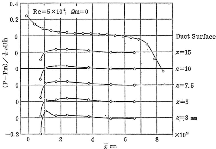
Fig. 3. 2. Pressure distribution in the case of Cylinder.
