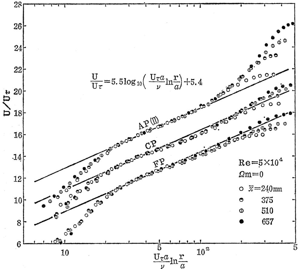
Fig. 4. 12. Logarithmic velocity distribution in the boundary layer with no rotation.
