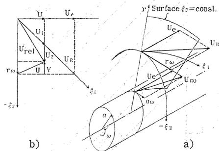
Fig. 3. 17. a) Rotating non-orthogonal frame. b) Relationship between various velocity components.
