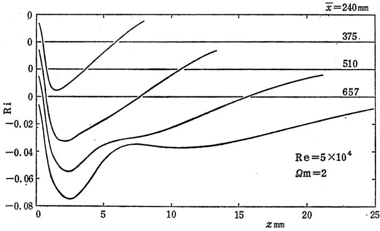
Fig. 4. 19. Distribution of Richardson number in the turbulent boundary layer for AP(II).
