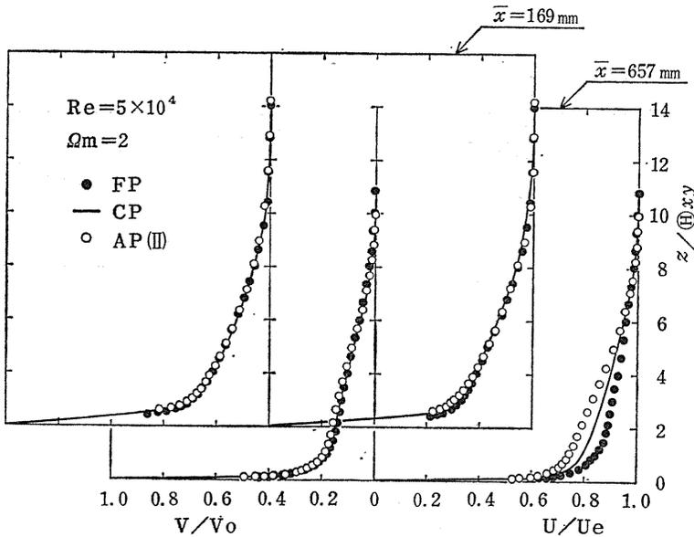
Fig. 4. 6. Comparison between velocity profiles for FP, CP and AP(II).
