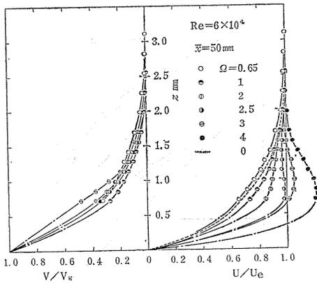
Fig. 2. 6. Velocity profiles on the hemispherical nose at high  $\Omega$  at  $\bar{x}=50\text{mm}$ .
