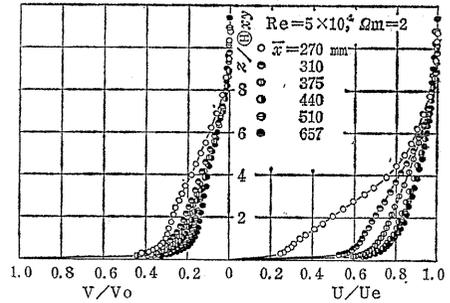
Fig. 3. 12. Velocity profiles for Step at  $\Omega_m=2$ .
