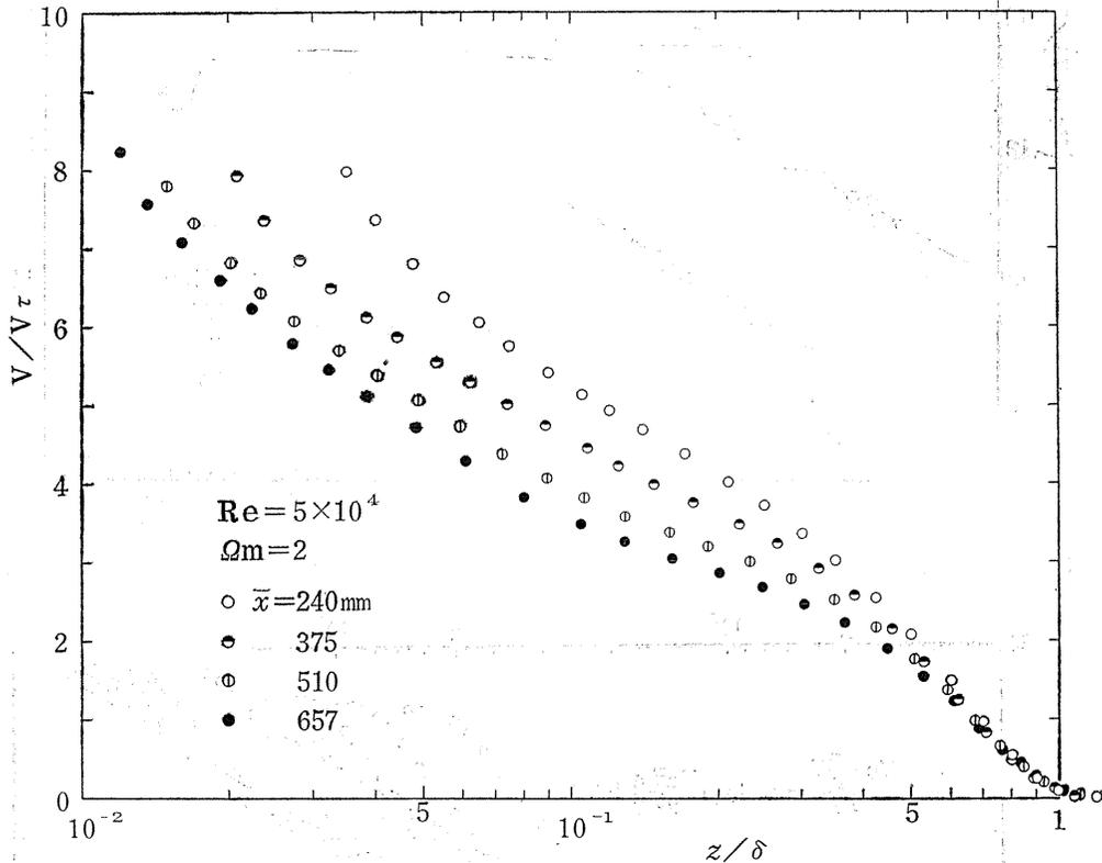
Fig. 4. 15. Logarithmic plots of peripheral velocity profiles for CP on the basis of the velocity-defect law in two-dimensional turbulent boundary layer.
