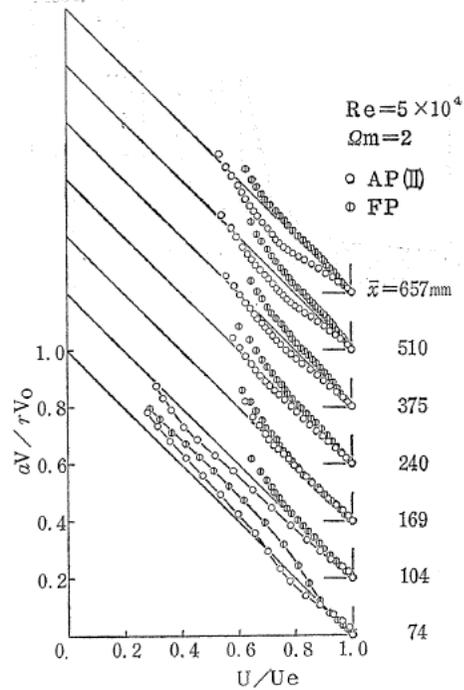
Fig. 4.7. Polar plots of velocity distribution for AP(II) and FP.
