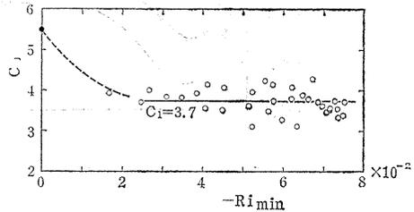
Fig. 4. 20. Change in the value of  $C_1$  in Eq. (4.23) in terms of the minimum value of Richardson number.
