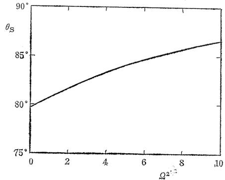
Fig. 2. 5. Shift of the separation point on a rotating sphere with increasing value of  $\Omega^2$ .
