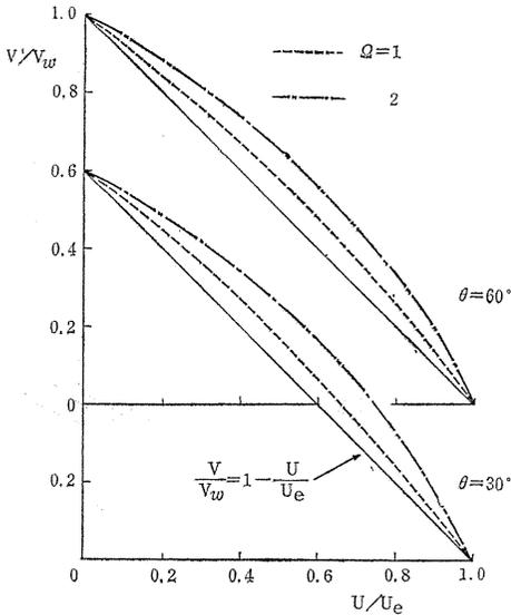
Fig. 2. 3. Polar plots, where  $V/V_w=1-U/U_e$  represents the quasi-collateral velocity distribution.
