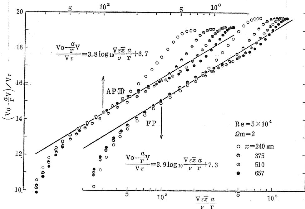
Fig. 4. 14. Logarithmic plots of peripheral velocity profiles for AP(II) and for FP on the basis of Eq. (4. 23).
