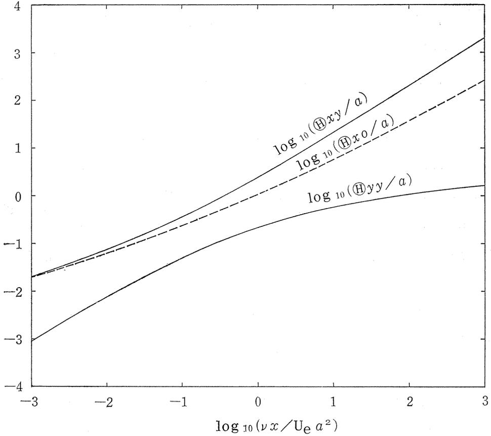
Fig. 2. 13. Non-dimensional momentum thickness  $\theta_{xy}$  and parameter  $\theta_{yy}$ .  $\theta_{x0}$  represents the value of  $\theta_x$  at  $\Omega=0$ .
