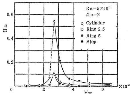
Fig. 3. 20. Variation of shape parameter  $H_{22}$  at  $\Omega_m=2$ .
