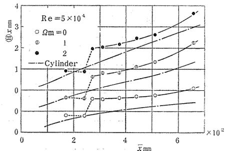
Fig. 3. 14. Developments of momentum thickness  $\theta_x$  for Ring 2.5.
