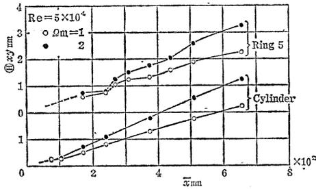
Fig. 3. 15. Developments of angular momentum thickness  $\theta_{xy}$  for Cylinder and Ring 5.
