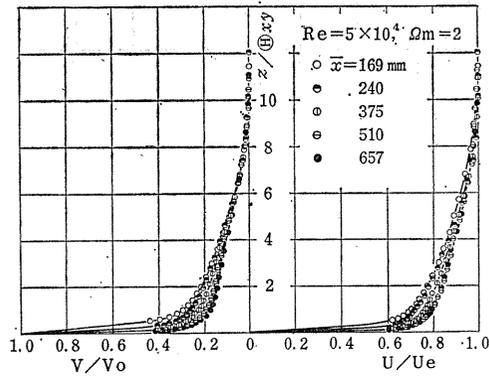
Fig. 3.4. Velocity profiles for Cylinder at  $\Omega_m=2$ .
