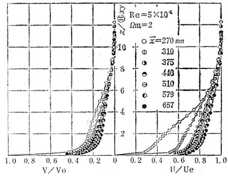
Fig. 3. 10. Velocity profiles for Ring 2.5 at  $\Omega_m=2$ .
