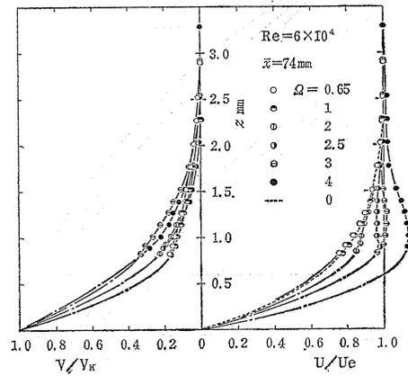
Fig. 2. 7. Velocity profiles on the hemispherical nose at high  $\Omega$  at  $\bar{x}=74\text{mm}$ .
