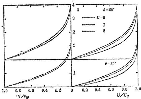
Fig. 2. 1. Velocity distribution on a rotating sphere using Fage's main flow.  $\theta$  is meridional angle measured from the forward stagnation point.  $U_e$ : main flow velocity,  $V_w$ : azimuthal velocity of the body surface.
