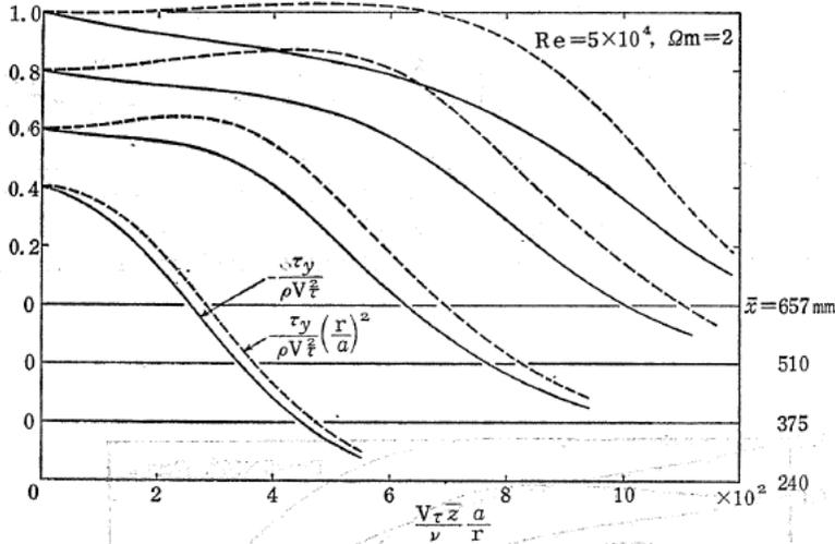
Fig. 4. 11. Distribution of peripheral shear stresses in the turbulent boundary layer for AP(II).
