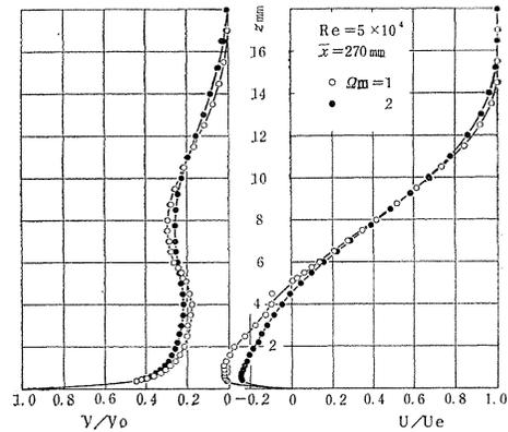
Fig. 3. 8. Velocity profiles at the station of  $\bar{x}=270$  mm for Ring 5.
