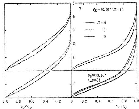
Fig. 2. 2. Velocity distribution at the separation point  $\theta_s$ .
