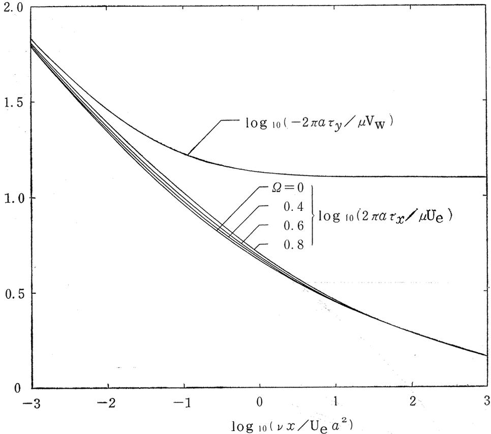
Fig. 2. 11. Non-dimensional wall shear-force components per unit length of the cylinder.
