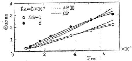
Fig. 4.9. Developments of angular momentum thickness  $\theta_{xy}$ . Experimental points represent the case of FP.
