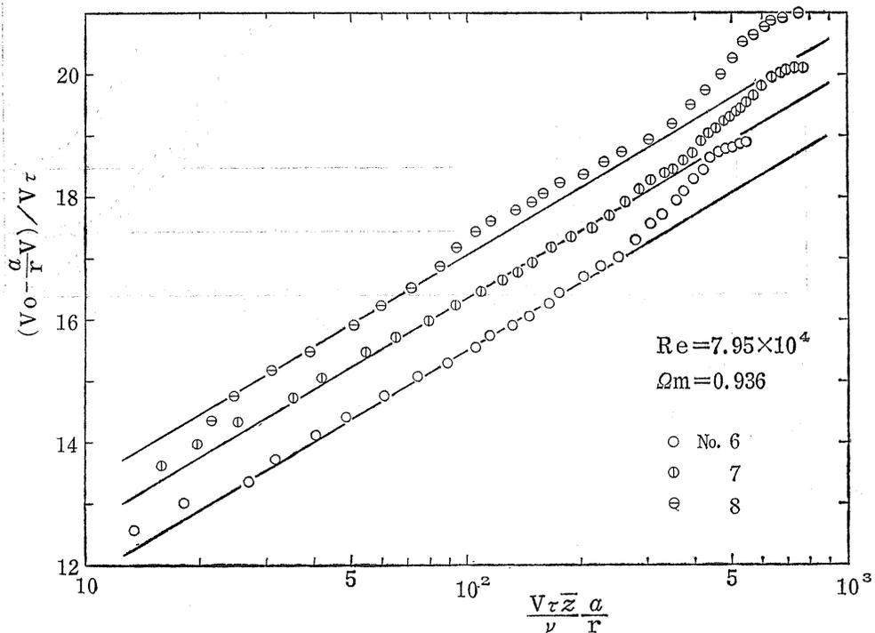
Fig. 4.17. Logarithmic plots of peripheral velocity profiles measured by Bissonnette & Mellor<sup>6)</sup> on the basis of Eq. (4.23): the value of  $C_1$  in Eq. (4.23) is 3.7.
