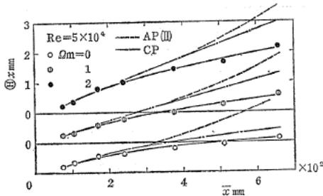
Fig. 4.8. Developments of momentum thickness  $\theta_x$ . Experimental points represent the case of FP.
