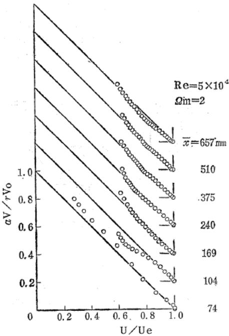
Fig. 3. 18. Polar plots of velocity distribution for Cylinder.
