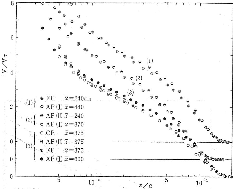
Fig. 4. 16. Logarithmic plots of peripheral velocity profiles in the turbulent boundary layers on the basis of the defect law (4. 16): (1)  $\Omega_m=2, \delta/a \doteq 0.156$ , (2)  $\Omega_m=2, \delta/a \doteq 0.124$ , (3)  $\Omega_m=1, \delta/a \doteq 0.165$ .
