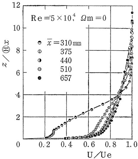
Fig. 3. 7. Velocity profiles of reattached flow for Ring 5 at  $\Omega_m=0$ .
