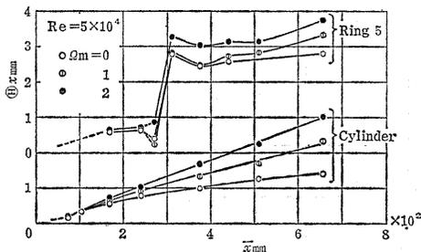
Fig. 3. 13. Developments of momentum thickness  $\theta_x$  for Cylinder and Ring 5.
