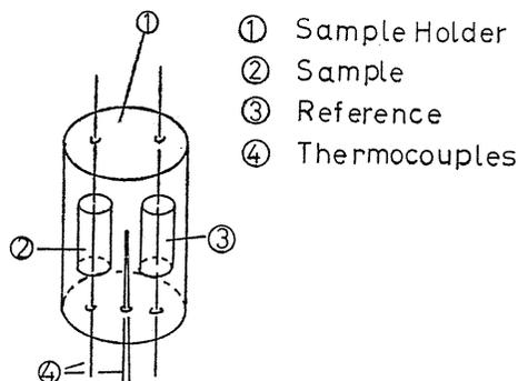
Fig. 9. Details of the sample holder.
