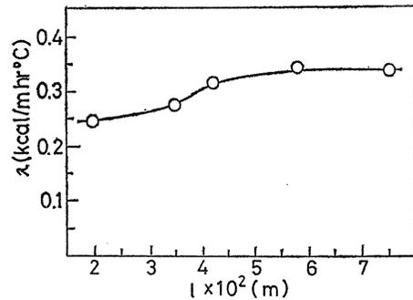
Fig. 5. An effect of the length of material on the measurement of a thermal conductivity.
