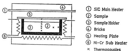
Fig. 15. (b) An experimental apparatus used for a slab sample.
