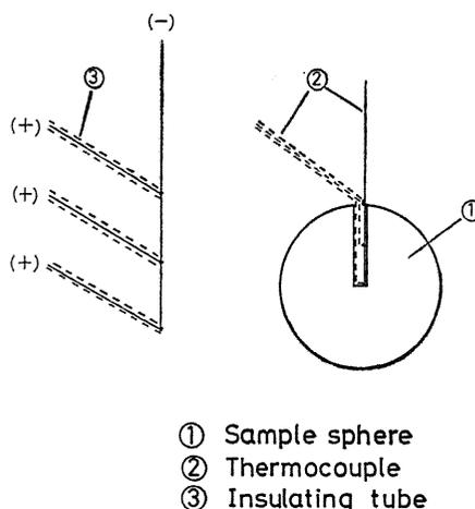
Fig. 15. (c) Details of the thermocouple connection employed for temperature measurement in a spherical sample.
