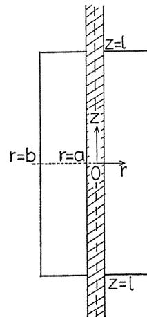
Fig. 2. A coordinate system of a hot wire method.
