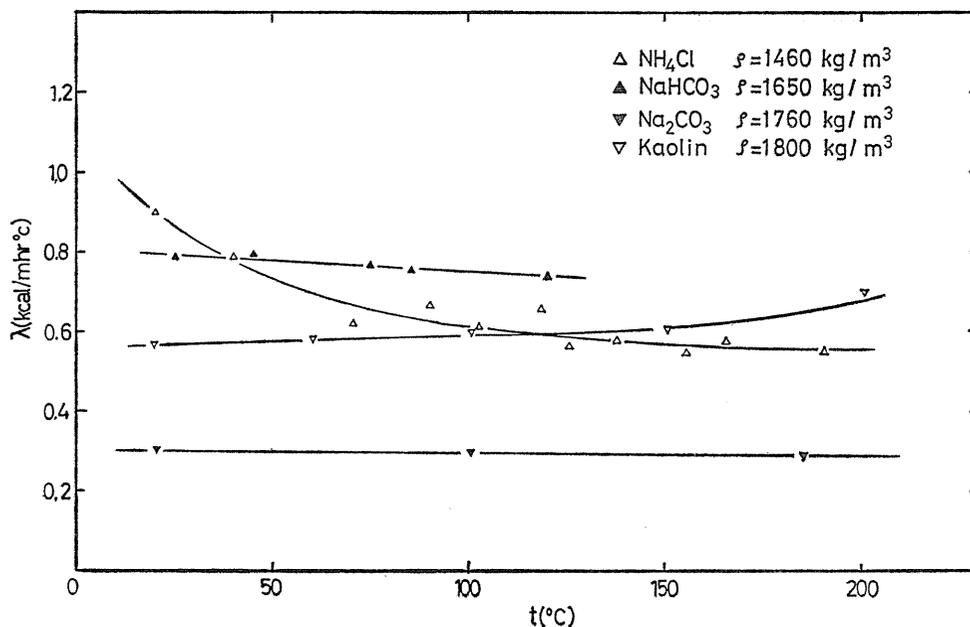
Fig. 6. Thermal conductivities in the non-reaction states measured by a hot wire method.
