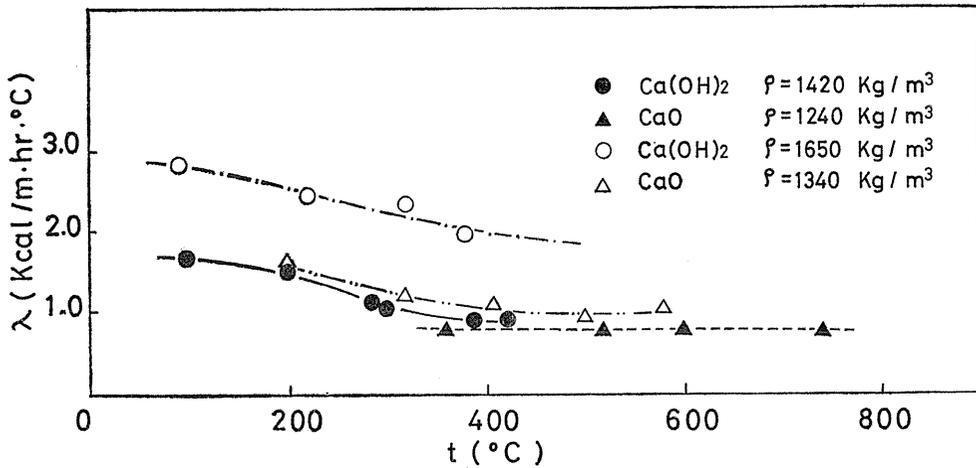
Fig. 16. Thermal conductivities of calcium hydroxide and calcium oxide measured by a hot wire method (non-reaction state).
