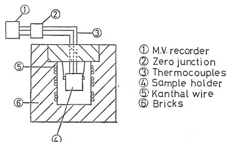
Fig. 8. A schematic drawing of the heating apparatus.
