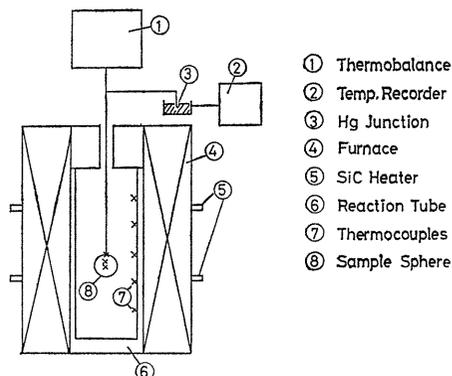
Fig. 15. (a) An experimental apparatus used for a spherical sample.
