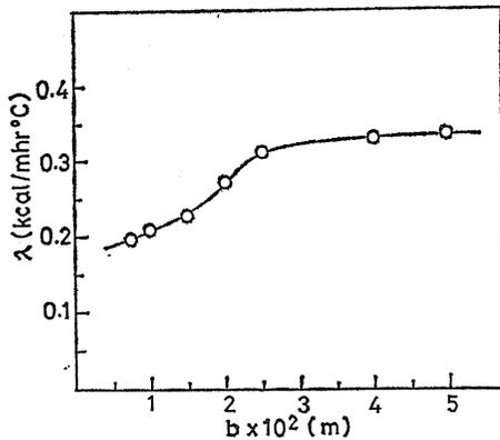
Fig. 4. An effect of the radius of material on the measurement of a thermal conductivity.
