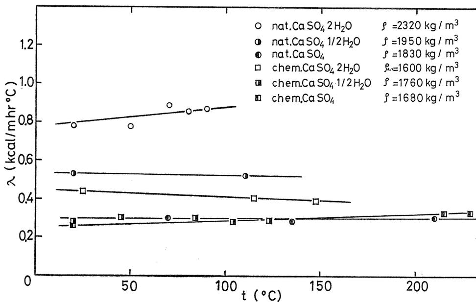
Fig. 7. Thermal conductivities in the non-reaction states measured by a hot wire method.
