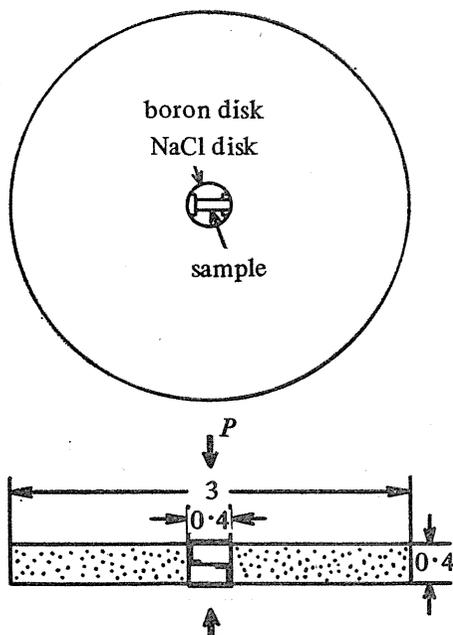
Fig. 2. Configuration of the sample cell for the pressure calibration.
