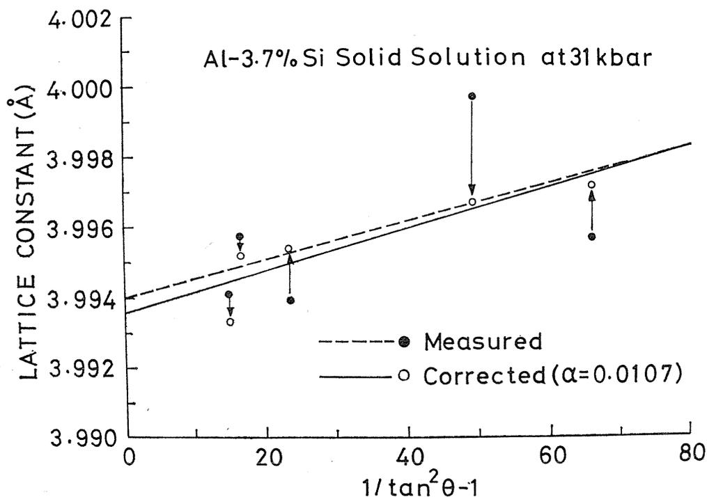
Fig. 27. Correction of peak shifts due to stacking faults.
