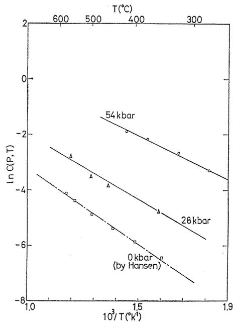
Fig. 15. Solute Si-concentration in Al as a function of the reciprocal temperature.
