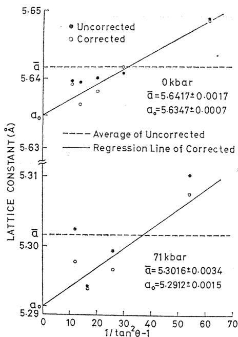
Fig. 26. Results of correction of the off-centering effect and extrapolation of the lattice constant of NaCl.
