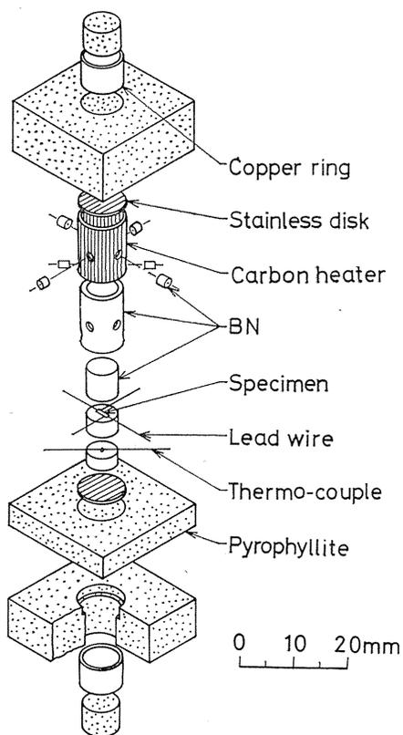
Fig. 4. Pressure cell assembly for measurements of electrical resistance used on the cubic anvil apparatus.
