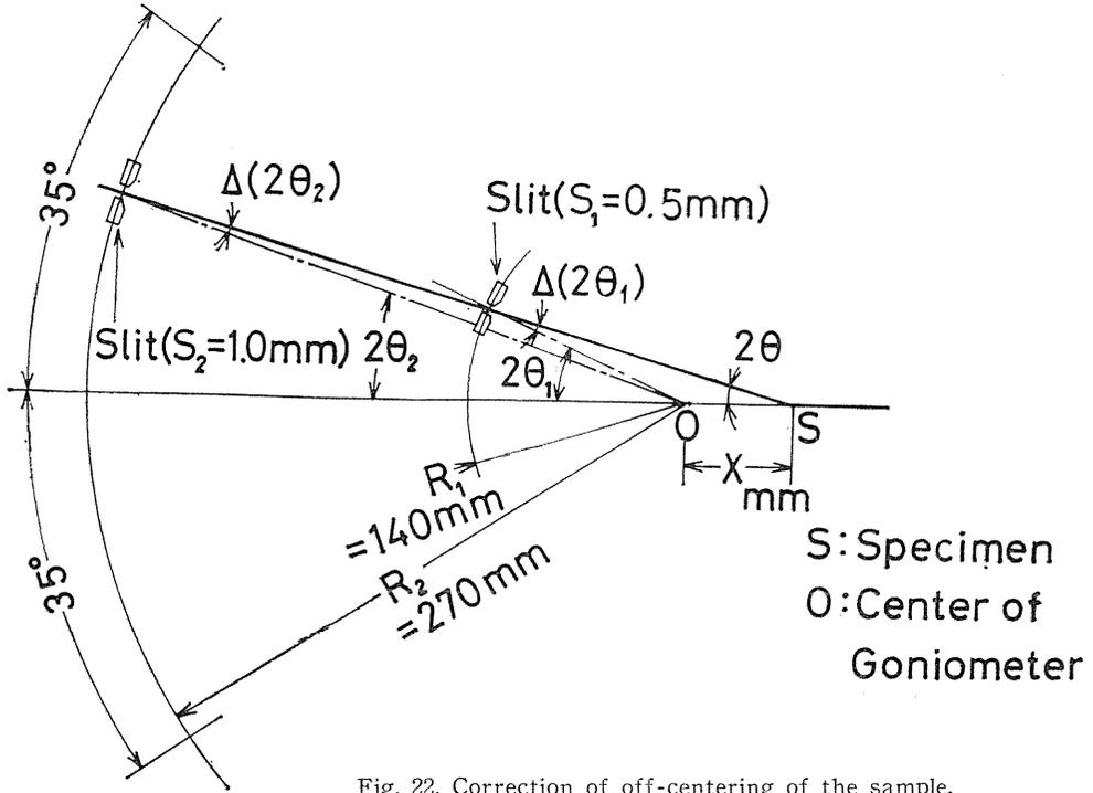
Fig. 22. Correction of off-centering of the sample.
