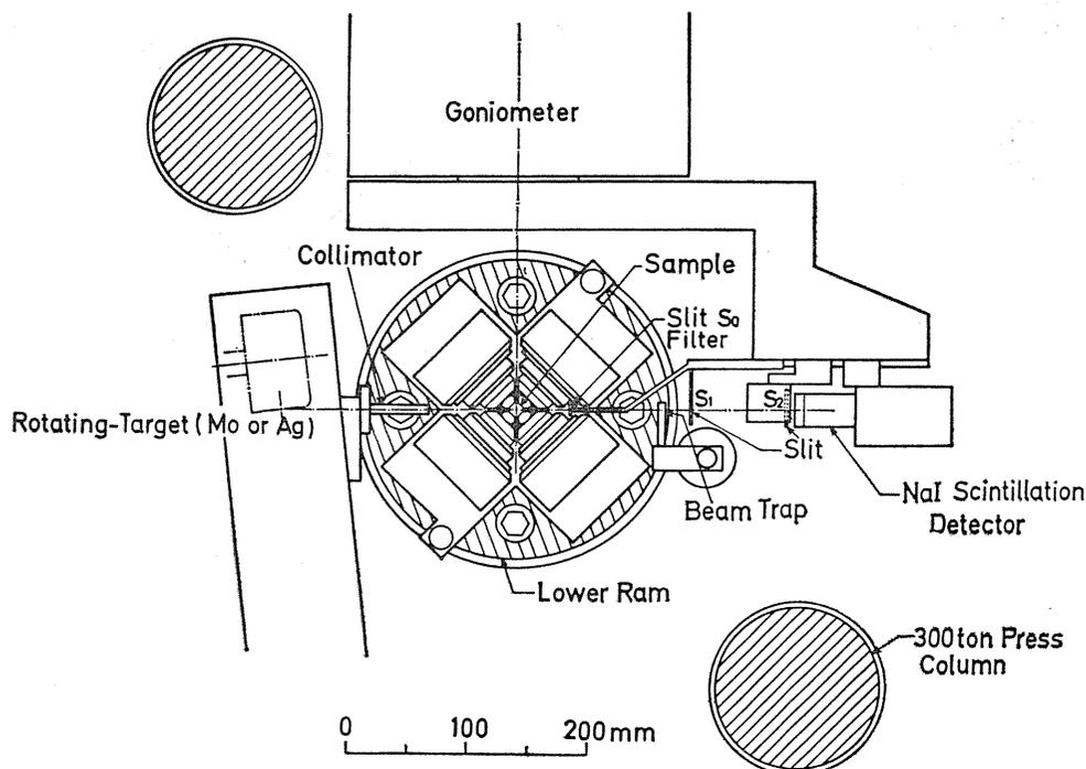
Fig. 19. Cubic anvil press equipped with high power X-ray source and goniometer.
