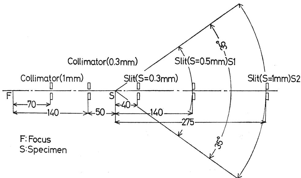
Fig. 20. Arrangement of collimator and slits in X-ray optical system.
