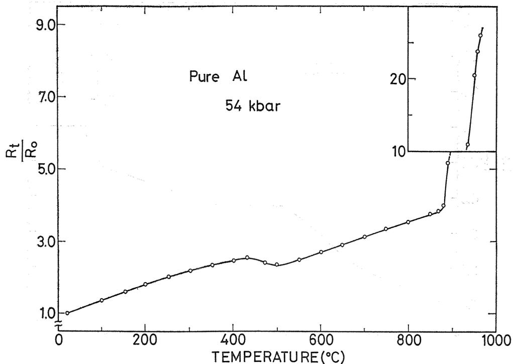
Fig. 6. Electric resistance vs. temperature relationship of pure Al at 54 kbar.
