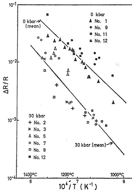
Fig. 18. Semilogarithmic plot of quenched-in resistivity vs. reciprocal of the absolute quenching temperature.
