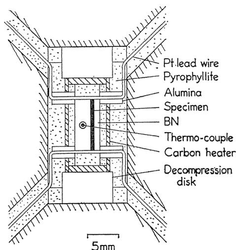
Fig. 5. Pressure cell assembly used on the girdle type apparatus.
