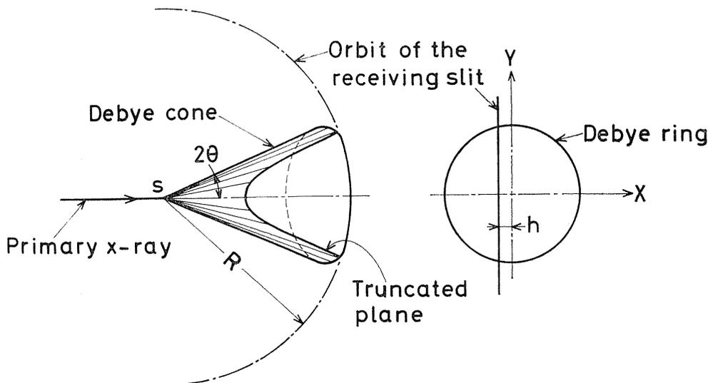
Fig. 23. Debye cone and orbit of receiving slit.
