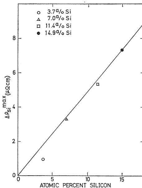
Fig. 11. Maximum of  $\Delta\rho_{\text{Si}}$  in Fig. 9,  $\Delta\rho_{\text{Si}}^{\text{max}}$ , as a function of Si-concentration.
