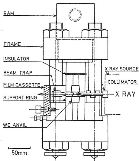
Fig. 1. Opposed anvil press equipped with an X-ray diffraction camera.
