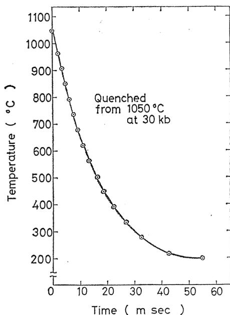
Fig. 17. Typical cooling curves of quenching in solid under high pressure.
