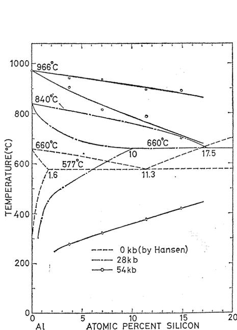
Fig. 14. Al-side phase diagram of Al-Si alloy at high pressure.
