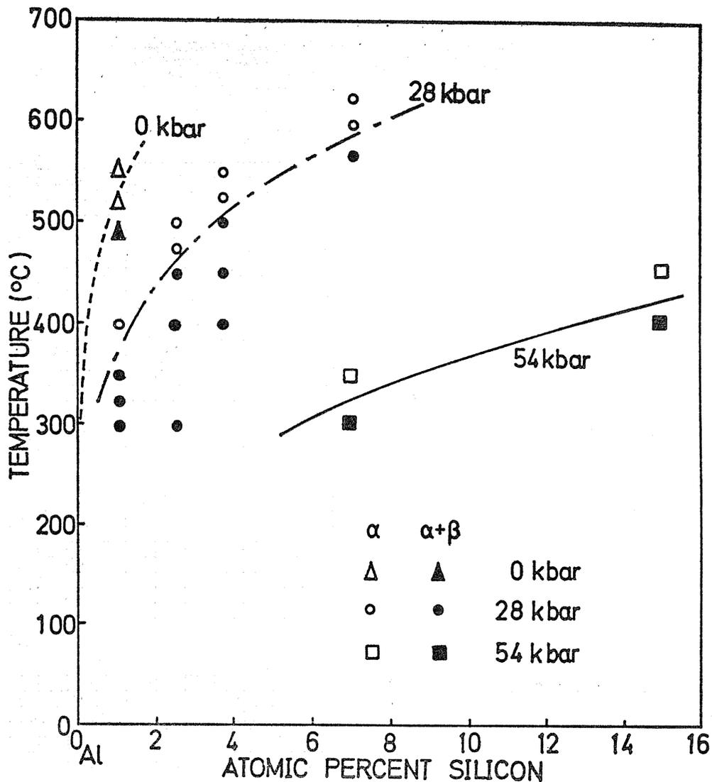
Fig. 13. Solubility limits of Si in Al under pressure of 28 and 54 kbar by means of the quenching method.
