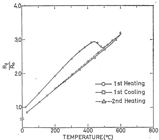
Fig. 7. Electric resistance change by alternate heating and cooling cycles on pure Al at 54 kbar.
