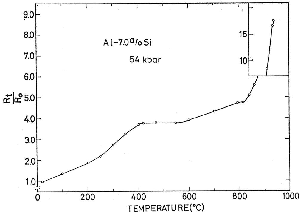
Fig. 8. Electric resistance vs. temperature relationship of Al-7.0% Si alloy at 54 kbar.
