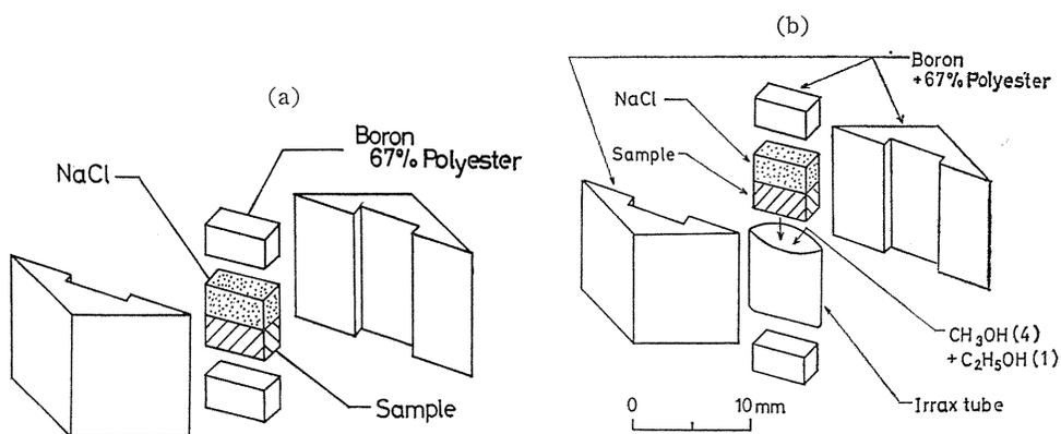
Fig. 21. Configuration of the sample cell for high pressure X-ray diffractometry. (a) Solid pressure-transmitting medium, (b) Liquid pressure-transmitting medium.
