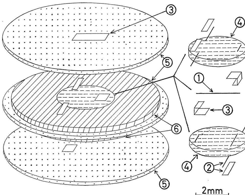
Fig. 16. Pressure cell assembly for vacancy study.
