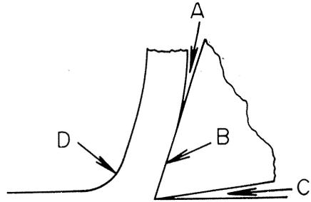
Fig. 1. Direction of cutting fluid entry.
