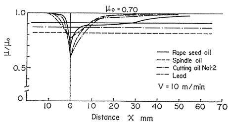
Fig. 10. Ratio of coefficient of friction with and without fluid.
