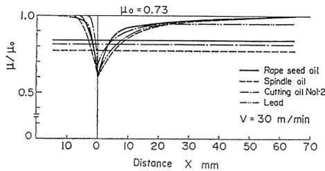
Fig. 9. Ratio of coefficient of friction with and without fluid.
