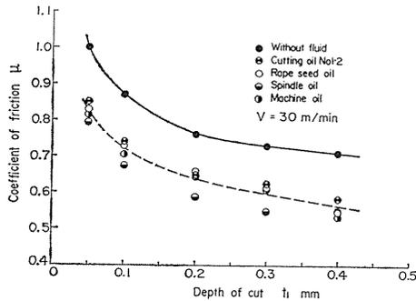
Fig. 5. Comparison of coefficients of frictions on cutting flooded and dry surfaces.
