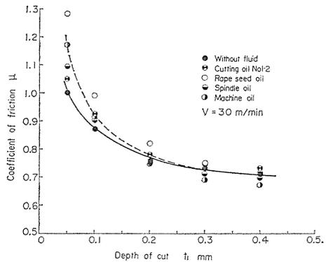
Fig. 4. Comparison of coefficients of frictions in cutting contaminated and clean surfaces.
