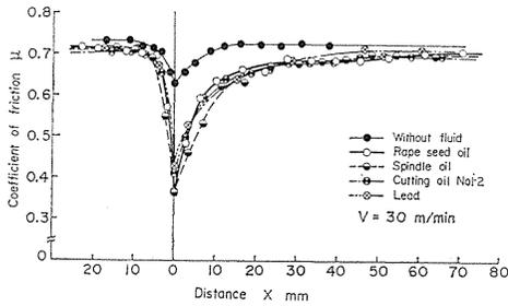
Fig. 8. Transitions of coefficients of frictions when tool penetrates hole with various fluid.
