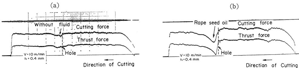
Fig. 7. Recorded charts in cutting workpieces having a hole with or without fluid.
