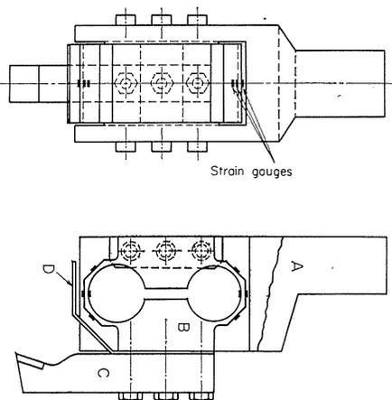
Fig. 2. Tool and dynamometer.
