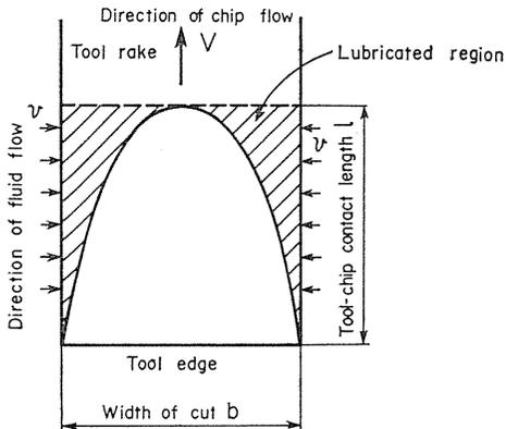
Fig. 13. Schematic view of the lubricated region.
