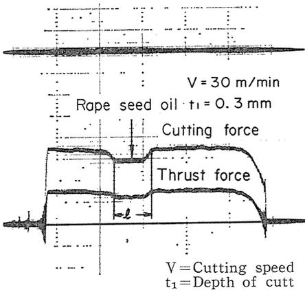
Fig. 3. An example of records of two components of cutting force.
