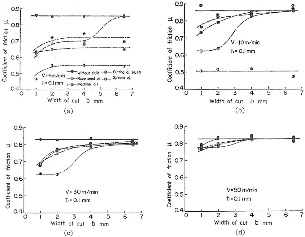
Fig. 12. Effect of cutting speed and width of cut on coefficient of friction.
