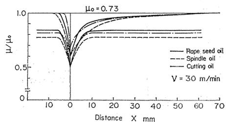
Fig. 11. Variation in coefficient of friction in cutting when hole is filled with fluid and a large quantity of fluid is simultaneously supplied from outside.
