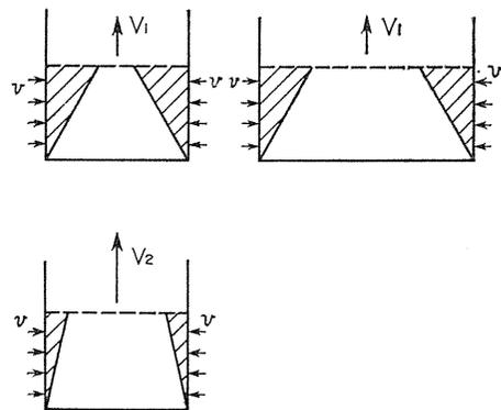
Fig. 14. Schematic view of contact region, assuming a constant speed of entry all over contact region.
