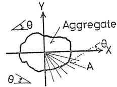
Fig. 2. 5. Method for measurement of inclination angle ( $\theta$ ) of bond crack.
