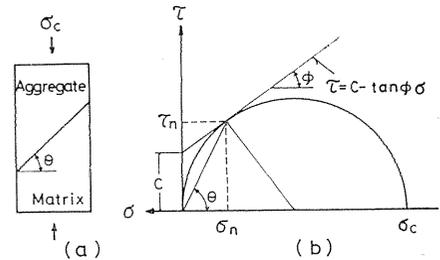
Fig. 2.7. Schematic bond failure criterion at the interface between coarse aggregate and mortar matrix.
