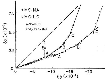
Fig. 3. 1. Relation between circumferential strain ( $\epsilon_x$ ) and longitudinal strain ( $\epsilon_y$ ).
