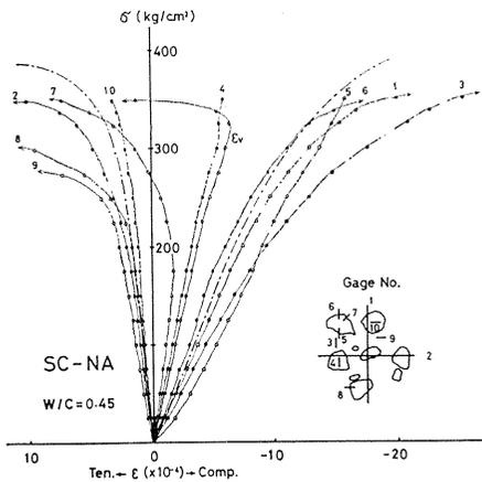
Fig. 2. 8. 1. Normal concrete ( $W/C=0.45$ )
