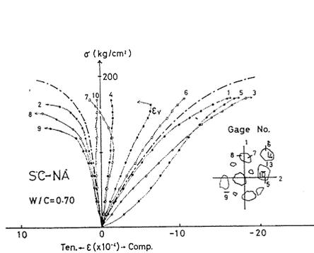
Fig. 2. 8. 3. Normal concrete ( $W/C=0.70$ )
