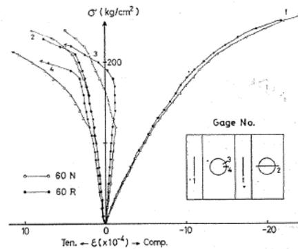
Fig. 4. 5. Stress ( $\sigma$ ) - strain ( $\epsilon$ ) relation of model concrete (Effect of surface condition of aggregate (Exp.-IV. 2. 1)).
