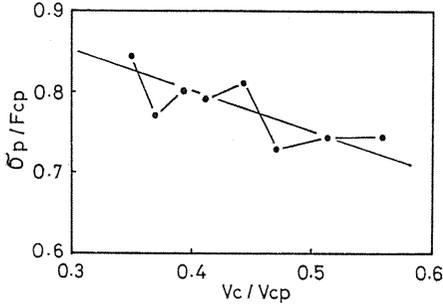
Fig. 3. 4. Relation between relative proportional limit ( $\sigma_p/F_{cp}$ ) and volume fraction of cement ( $V_c/V_{cp}$ ) of cement paste.
