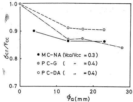
Fig. 3. 17. Effect of size of aggregate ( $\phi_a$ ) on relative critical stress ( $\sigma_{cr}/F_{cc}$ ).
