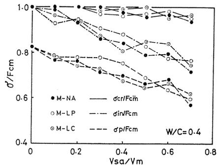
Fig. 3. 5. Relation between relative characteristic stresses ( $\sigma/F_{cm}$ ) and volume fraction of fine aggregate ( $V_{sa}/V_m$ ) of mortar.
