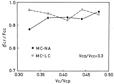
Fig. 3. 12. Relation between relative critical stress ( $\sigma_{cr}/F_{cc}$ ) and volume fraction of cement ( $V_c/V_{cp}$ ) of MC-series concrete.
