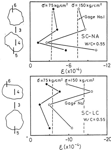
Fig. 2. 9. Strain distribution of plate specimen in longitudinal direction.
