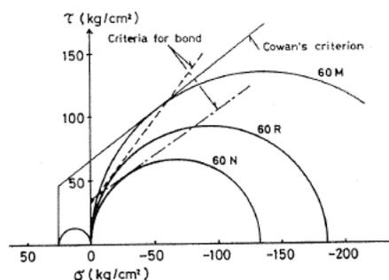
Fig. 4. 8. Schematic failure criteria of mortar matrix and bond at the interface.
