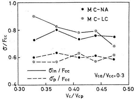
Fig. 3. 11. Relation between relative characteristic stresses ( $\sigma/F_{cc}$ ) and volume fraction of cement ( $V_c/V_{cp}$ ) of MC-series concrete.
