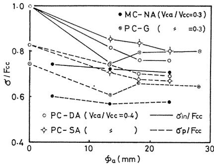
Fig. 3. 16. Effect of size of aggregate ( $\phi_a$ ) on relative proportional limit ( $\sigma_p/F_{cc}$ ) and relative initiation stress ( $\sigma_{in}/F_{cc}$ ).
