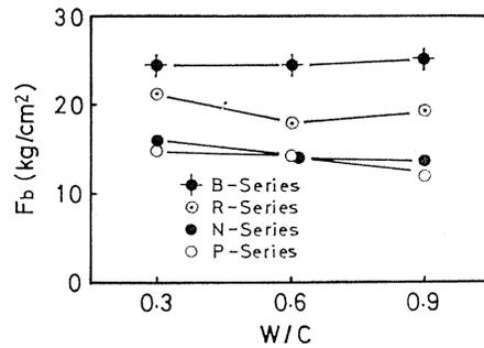
Fig. 4. 2. Relation between flexural bond strength ( $F_b$ ) and water-cement ratio of mortar aggregate ( $W/C$ ).
