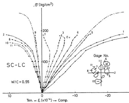
Fig. 2. 8. 4. Lightweight aggregate concrete ( $W/C=0.55$ )
