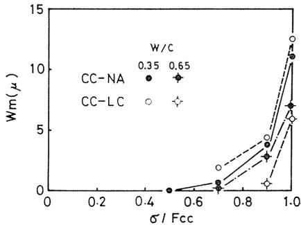
Fig. 2. 4. Relation between maximum width of mortar crack ( $W_m$ ) and relative amount of stress ( $\sigma/F_{cc}$ ).
