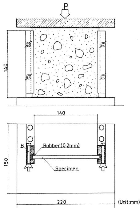
Fig. 2. 1. Loading device used in Exp. - II . 2.
