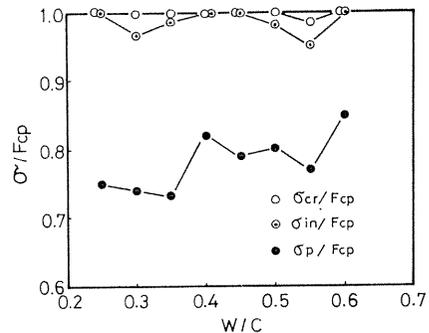
Fig. 3. 3. Relation between relative characteristic stresses ( $\sigma/F_{cp}$ ) and water-cement ratio ( $W/C$ ) of cement paste.
