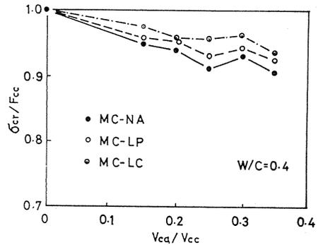
Fig. 3. 10. Relation between relative critical stress ( $\sigma_{cr}/F_{cc}$ ) and volume fraction of coarse aggregate ( $V_{ca}/V_{cc}$ ) of MC-series concrete.
