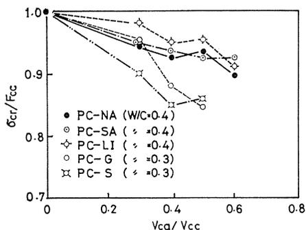
Fig. 3. 15. Effect of type of coarse aggregate on relative critical stress ( $\sigma_{cr}/F_{cc}$ ) of PC-series concrete.
