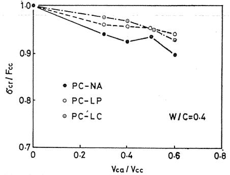
Fig. 3. 8. Relation between relative critical stress ( $\sigma_{cr}/F_{cc}$ ) and volume fraction of coarse aggregate ( $V_{ca}/V_{cc}$ ) of PC-series concrete.
