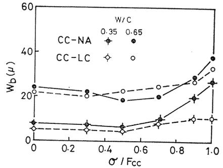
Fig. 2. 3. Relation between maximum width of bond crack ( $W_b$ ) and relative amount of stress ( $\sigma/F_{cc}$ ).
