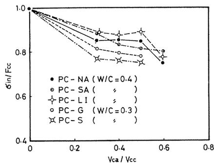
Fig. 3. 14. Effect of type of coarse aggregate on relative initiation stress ( $\sigma_{in}/F_{cc}$ ) of PC-series concrete.
