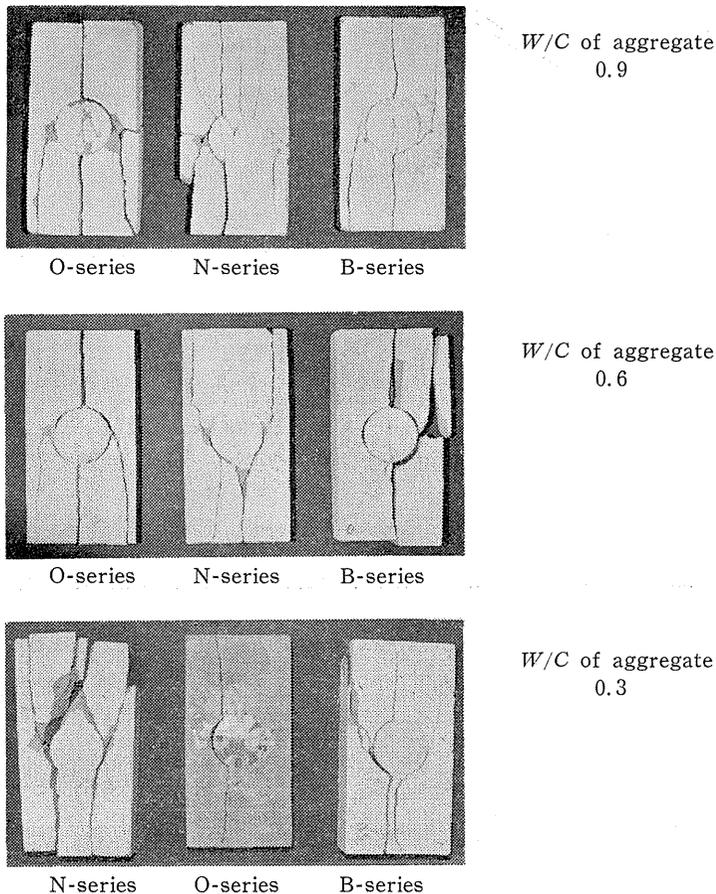
Photo. 4. 1. Typical failure mode of model concrete (Exp.-IV. 2. 2).
