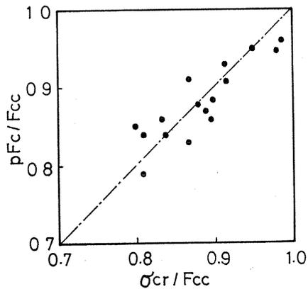
Fig. 3. 19. Relation between relative compressive strength ( ${}_pF_c/F_{cc}$ ) of PA-series specimen and relative critical stress ( $\sigma_{cr}/F_{cc}$ ) of NO-series specimen.
