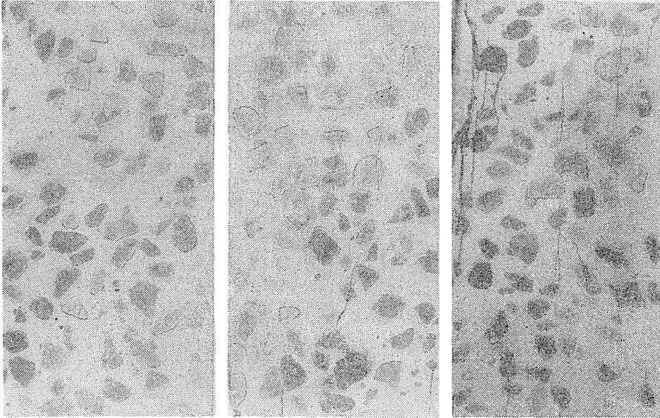
Photo. 2. 2. 1.  $\sigma/F_{cc}=0$ Photo. 2. 2. 2.  $\sigma/F_{cc}=0.7$ Photo. 2. 2. 3.  $\sigma/F_{cc}=1.0$
