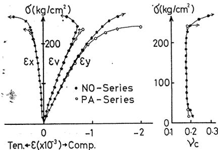
Fig. 3. 18. Effect of end condition of specimen on stress ( $\sigma$ ) - strain ( $\epsilon$ ) and stress ( $\sigma$ ) - Poisson's ratio ( $\nu_c$ ) relations.
