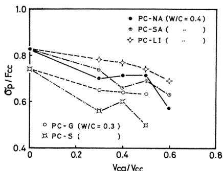
Fig. 3. 13. Effect of type of coarse aggregate on relative proportional limit ( $\sigma_p/F_{cc}$ ) of PC-series concrete.
