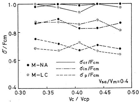
Fig. 3. 6. Relation between relative characteristic stresses ( $\sigma/F_{cm}$ ) and volume fraction of cement ( $V_c/V_{cp}$ ) of mortar.
