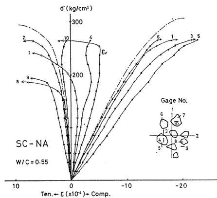
Fig. 2. 8. 2. Normal concrete ( $W/C=0.55$ )
