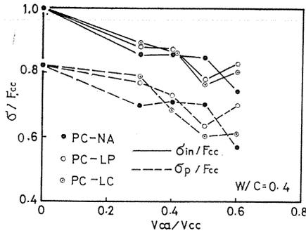
Fig. 3. 7. Relation between relative characteristic stresses ( $\sigma/F_{cc}$ ) and volume fraction of coarse aggregate ( $V_{ca}/V_{cc}$ ) of PC-series concrete.
