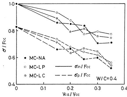
Fig. 3. 9. Relation between relative characteristic stresses ( $\sigma/F_{cc}$ ) and volume fraction of coarse aggregate ( $V_{ca}/V_{cc}$ ) of MC-series concrete.
