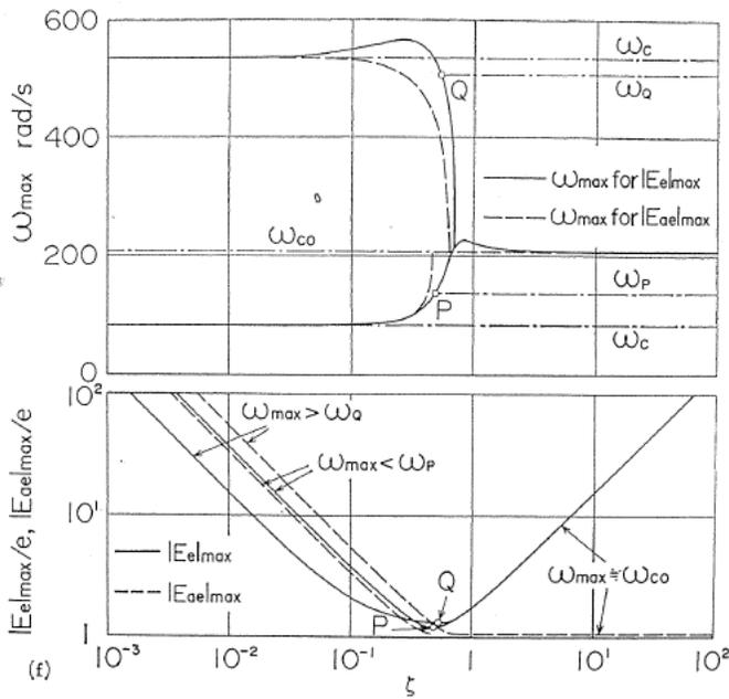
Fig. 2. Rotor response  $|E_e|, |F_e|, |E_\tau|, |F_\tau|$  and pedestal response  $|E_{ae}|, |E_{a\tau}|$  versus rotating speed  $\omega$  for various amounts of damping; system shown in Fig. 1, Fig. 7 (a) and Fig. 8.
