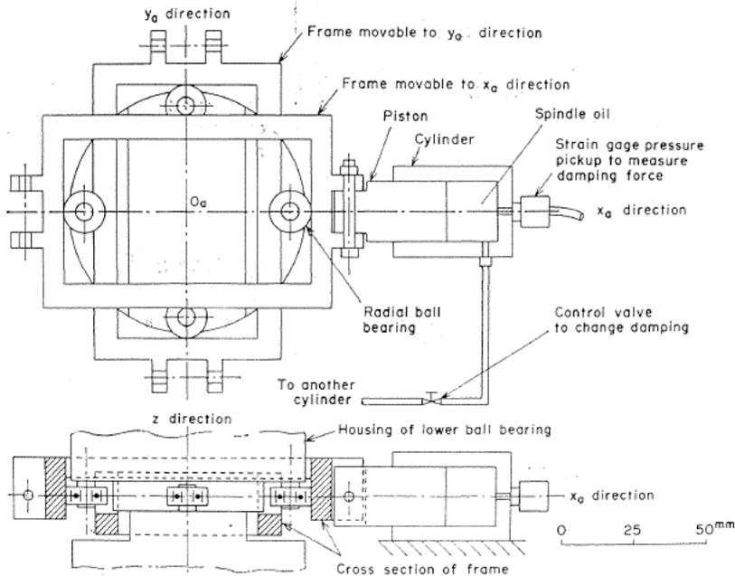
Fig. 9. Pressure-pickup type dashpot.
