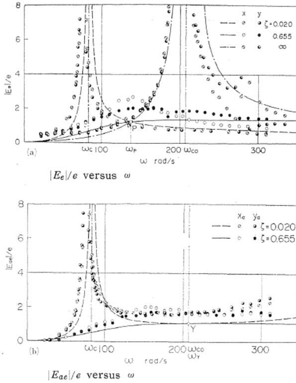
Fig. 10. Response curves with nearly equal damping in two directions  $x_a, y_a$ . ( $m_a/m=0.309, k_a/\alpha=0.1115$ )
