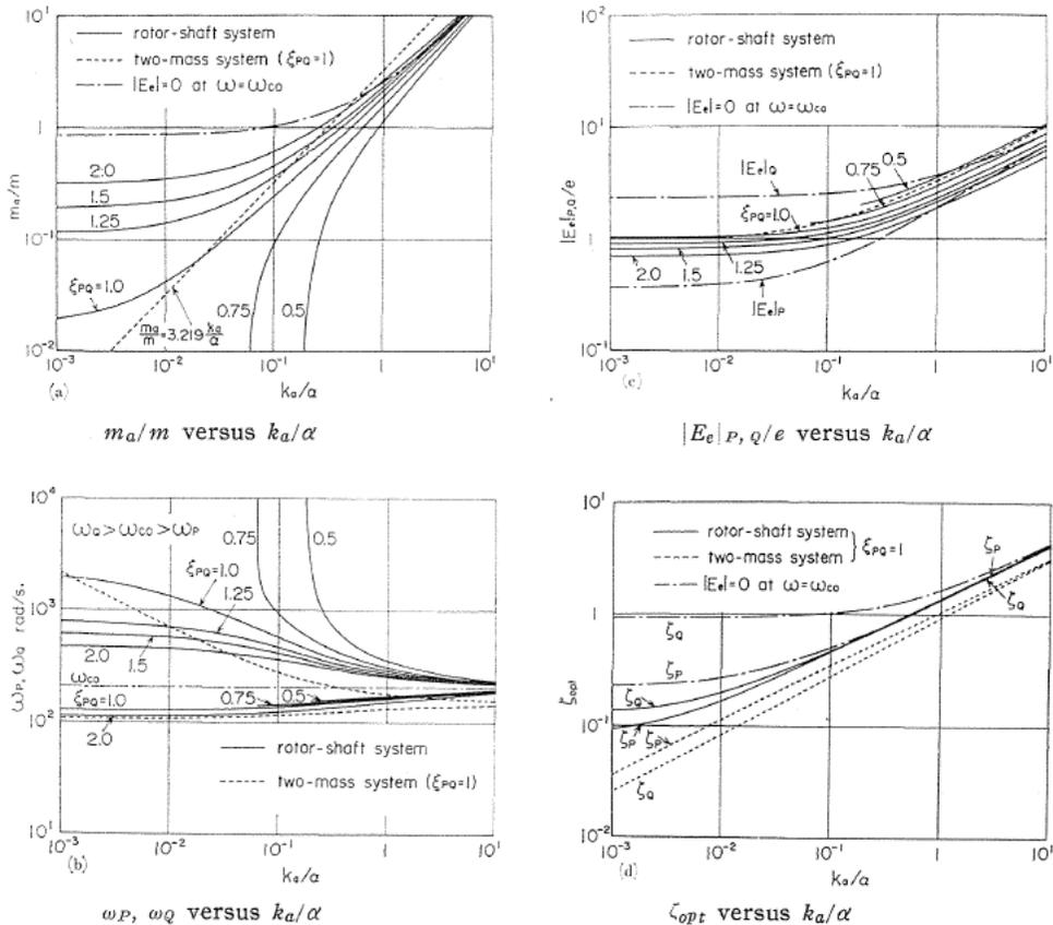
Fig. 4. The most favorable choice of  $m_a/m$ ,  $k_a/\alpha$ , and optimum damping  $\zeta_{opt}$  as regards rotor response  $|E_e|$  due to static unbalance  $e$ .
