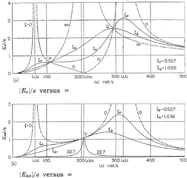
Fig. 3. Response curves  $|E_e| - \omega$ , and  $|E_{ae}| - \omega$  for a favorable case derived by letting amplitude  $E_e = 0$  at  $\omega = \omega_{c0} = 207.1$  rad/s. ( $m_a/m = 1.062$ ,  $k_a/\alpha = 0.1115$ ,  $\xi_{PQ} = 3.94$ ,  $\zeta_P = 0.527$ ,  $\zeta_Q = 1.036$ )
