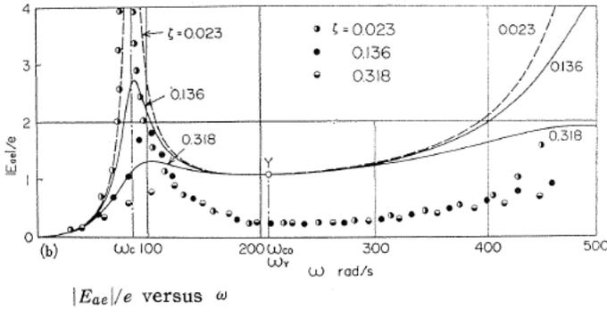
Fig. 11. Response curves with nearly equal damping in two directions  $x_a, y_a$ . ( $m_a/m=0.340, k_a/\alpha=0.1265$ )
