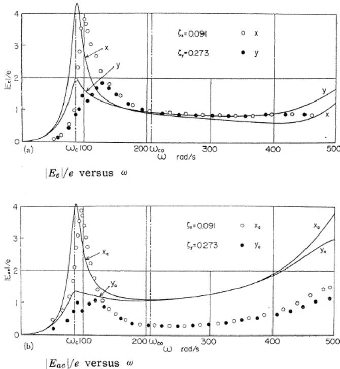
Fig. 12. Response curves with unequal damping in two directions  $x_a, y_a$ . ( $m_a/m=0.340, k_a/\alpha=0.1265, \zeta_y/\zeta_x=3$ )
