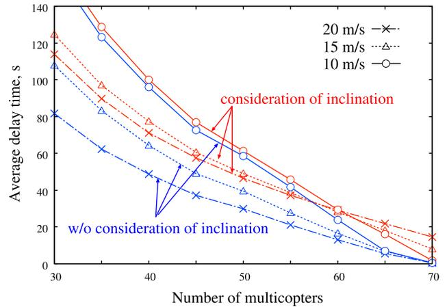
**Fig. 12** Average delay time considering inclination of multicopters.
