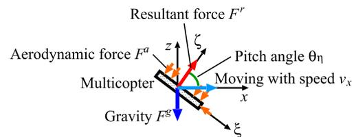
Fig. 9 Dynamic model of a flying multicopter.
