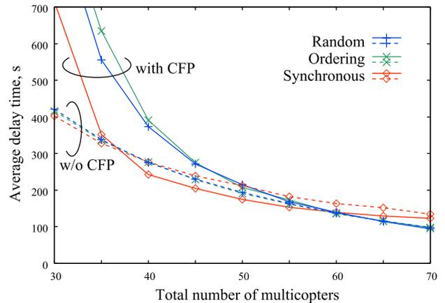
Fig. 8 Average delay time of the random, ordering, and synchronous drop timings for the rebounding flight scheme.
