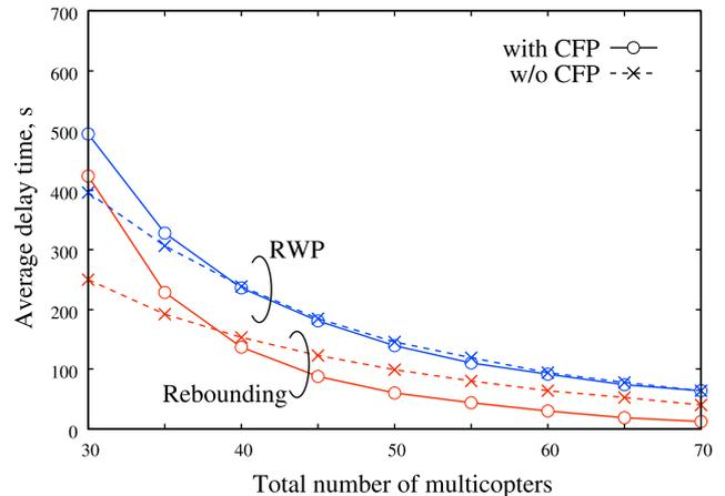
Fig. 4 Average delay time of RWP and rebounding flight schemes with and without CFP.
