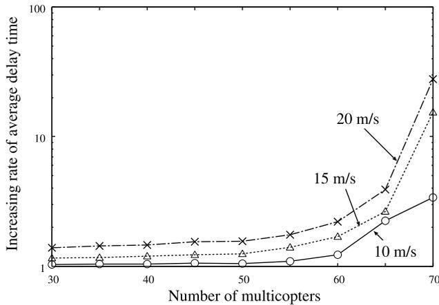
**Fig. 13** Increasing rate of average delay time considering the inclination of multicopters.
