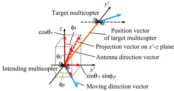
**Fig. 11** A model of intending and target multicopters to calculate gain of polarization plane deviation.
