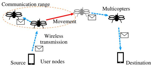
**Fig. 1** An aerial wireless relay network.
