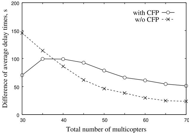
**Fig. 5** The difference of the average delay times between RWP and rebounding flight schemes.
