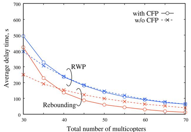
Fig. 4 Average delay time of RWP and rebounding flight schemes with and without CFP.
