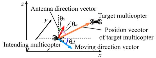
**Fig. 10** A model of intending and target multicopters to calculate relative antenna gain.
