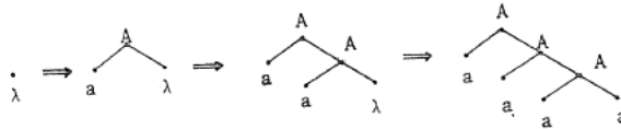
FIG. 3.2. A topological representation of the generation process of a tree t(\mu(t) = (Aa)^3a) in T(S) .
