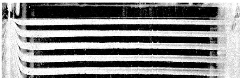
FIG. 5. Visualized transverse velocity profile. The flow direction is from top to bottom, where the wire is placed normal to the flow and parallel to the bottom wall at y = 70 mm.
