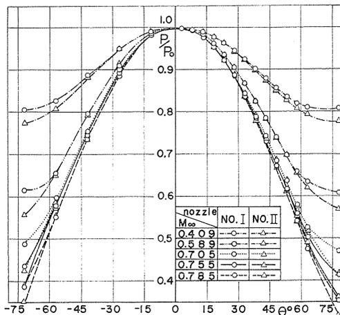
FIG. 9. Comparison between pressure distribution around a cylinder in Nozzle I and Nozzle II,
