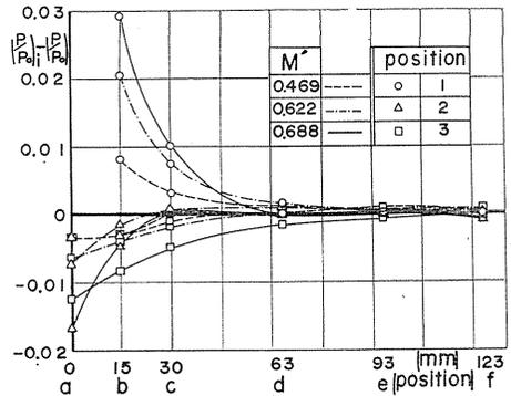
FIG. 7. Effect of cylinder on static pressure along the wall.
