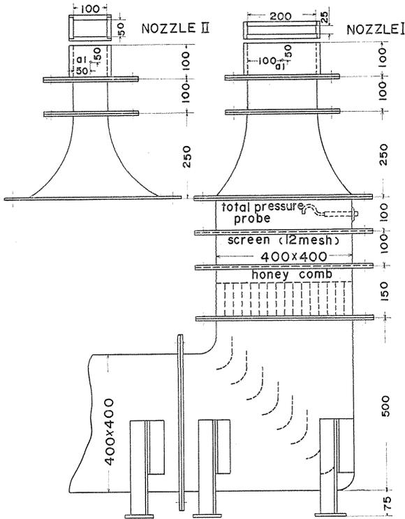
FIG. 2. Wind tunnel.
