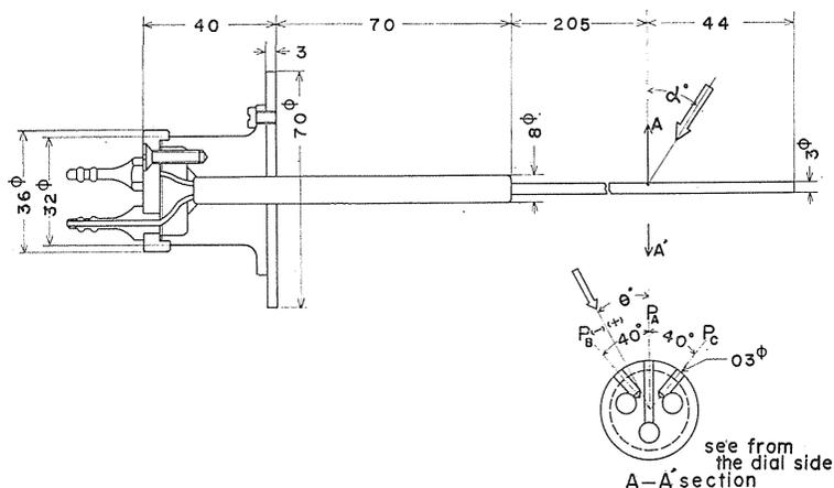
FIG. 4. Three-holes cylindrical probe.
