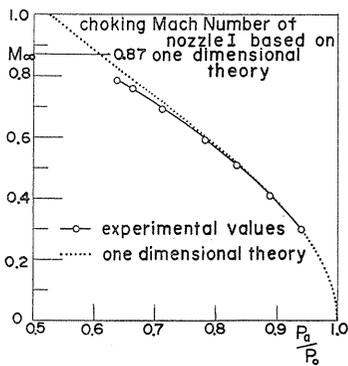
FIG. 8. Mach number variation versus tunnel total pressure,
