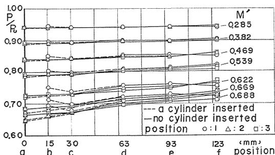
FIG. 6. Pressure distribution along the wall of Nozzle I.
