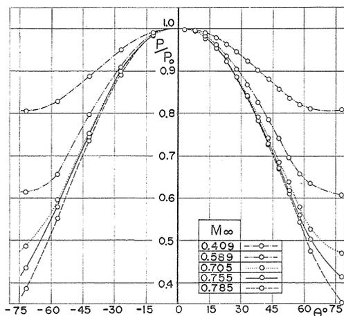
FIG. 5. Pressure distribution around a cylinder in Nozzle I.
