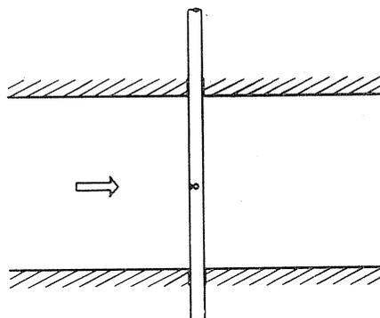
FIG. 1. Cylindrical probe in the flow passage.
