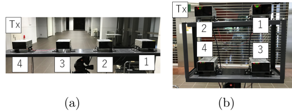
Fig. 5. Position of optical modulators in the array for two different arrangements:(a) Linear arrangement (b) Square arrangement
