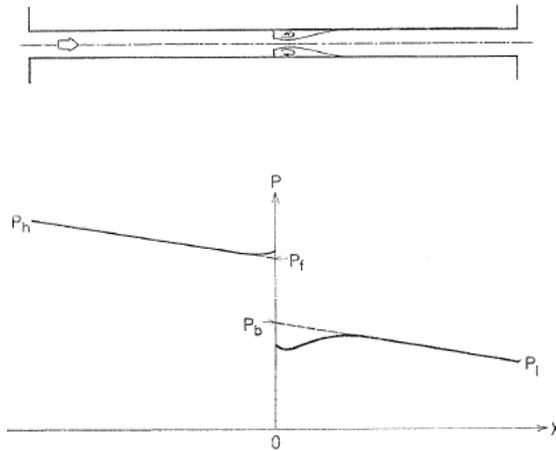
FIG. 4. Pressure distribution in a pipe orifice.
