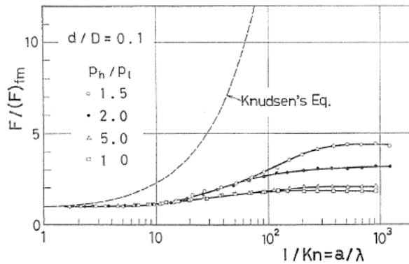
FIG. 5-c. Overall conductance of the pipe orifice ( $d/D=0.1$ ).
