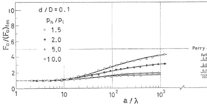
FIG. 9-c. Pure conductance of the orifice ( $d/D=0.1$ ).
