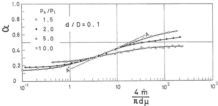
FIG. 10-c. Discharge coefficient ( $d/D=0.1$ ).
