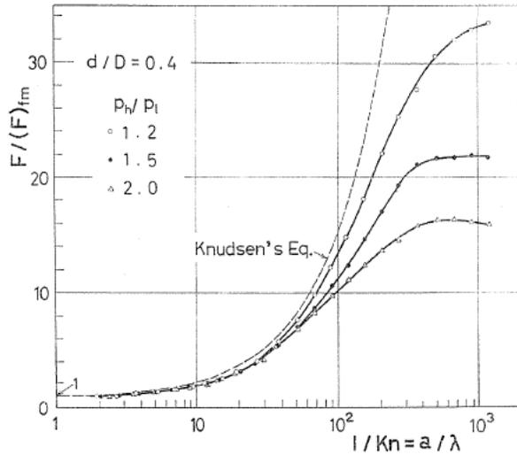
FIG. 5-b. Overall conductance of the pipe orifice ( $d/D=0.4$ ).
