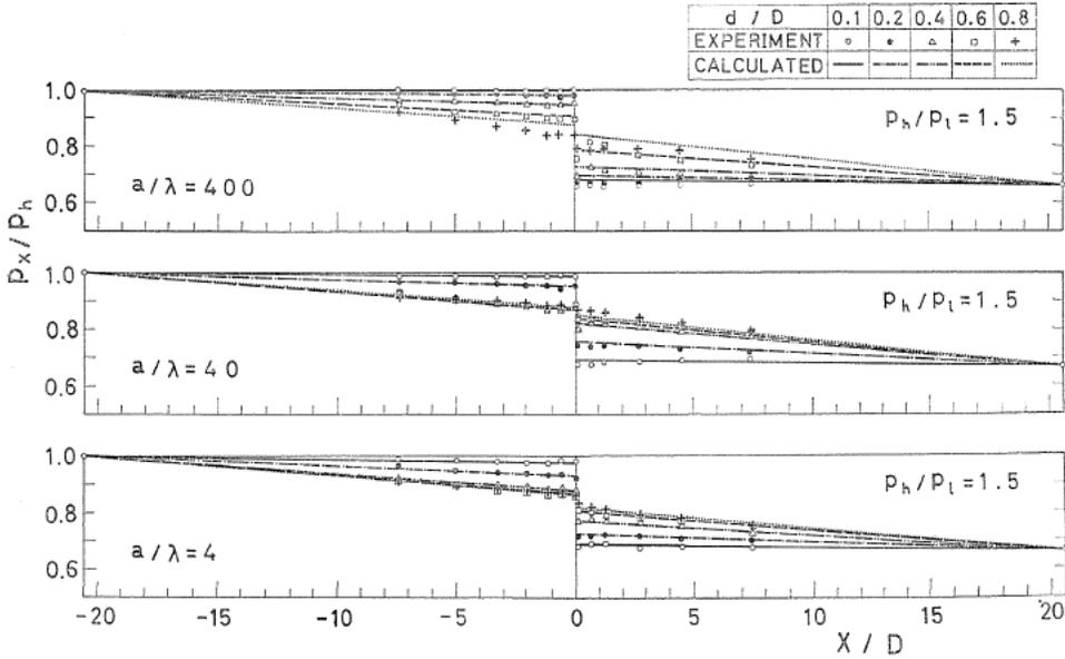
FIG. 8. Pressure distributions in the pipe orifice.
