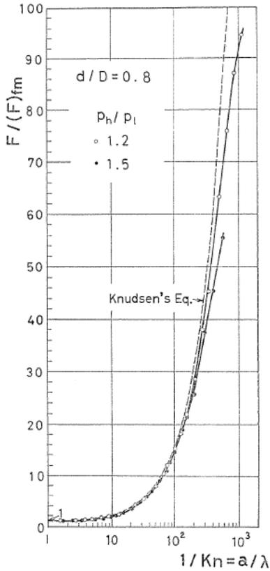
FIG. 5-a. Overall conductance of the pipe orifice ( $d/D=0.8$ ).
