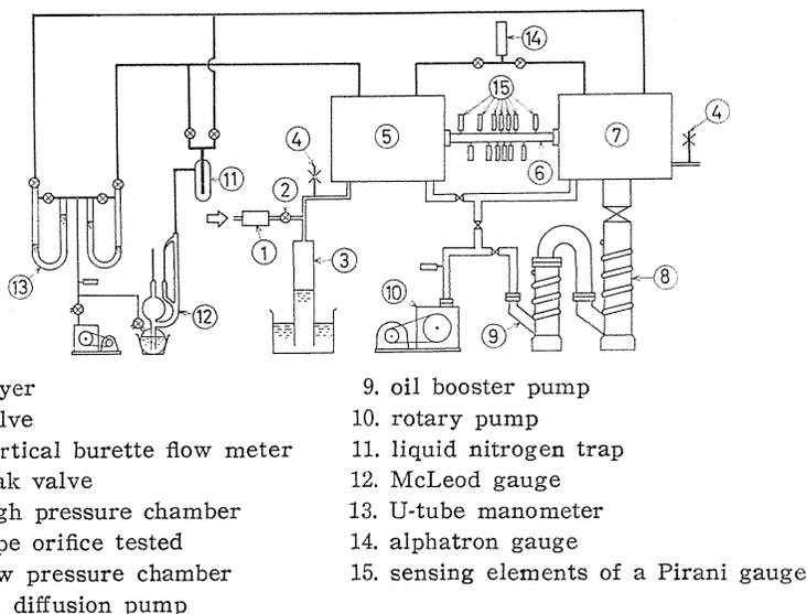
FIG. 1. Experimental arrangement for conductance measurements of pipe orifices.
