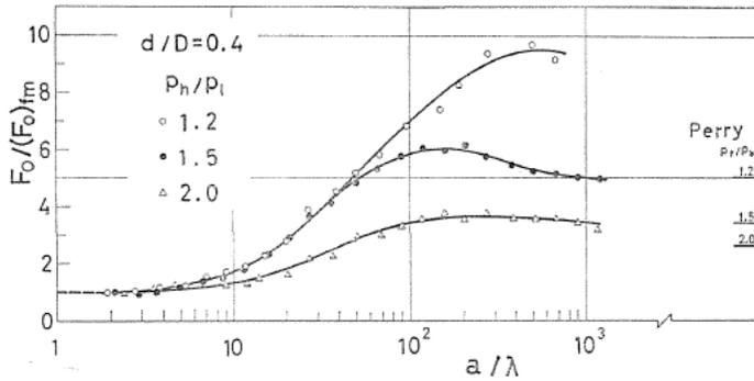
FIG. 9-a. Pure conductance of the orifice ( $d/D=0.4$ ).
