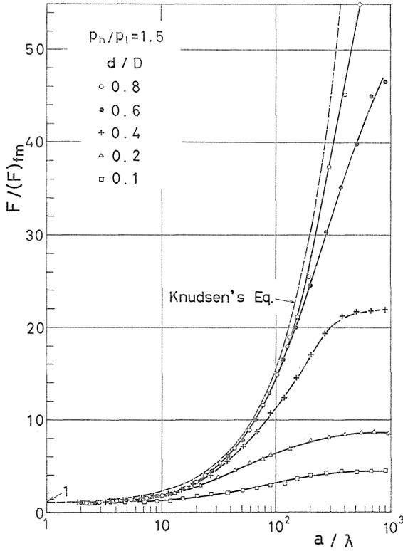
FIG. 6. Overall conductance of the pipe orifice ( $p_h/p_l=1.5$ ).
