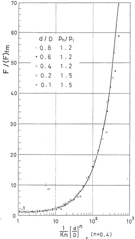
FIG. 7. Comparison of the measured conductance with the empirical equation (9) when the pressure ratio is very close to unity.
