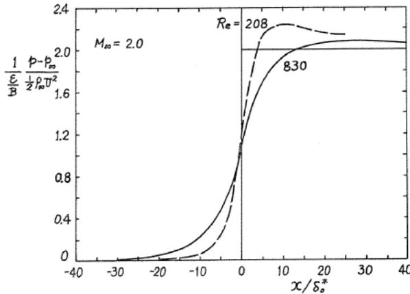
FIG. 5. Pressure distribution along the wall.
