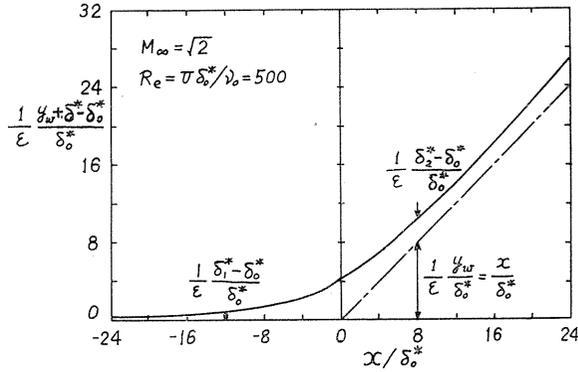
FIG. 6. Distribution of displacement thickness.
