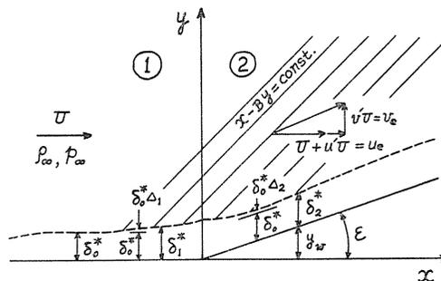
FIG. 1. Flow pattern of the boundary layer around a wedge slope.
