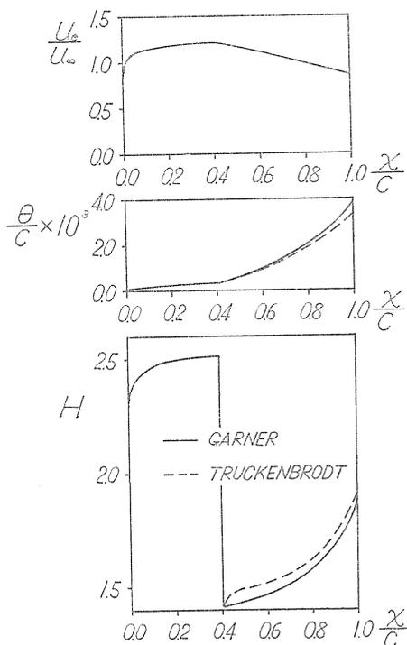
FIG. 1. The velocity distribution and the variations of momentum thickness, shape factor. NACA 642-015  $Re=10^5$ ,  $\alpha=0^\circ$ .
