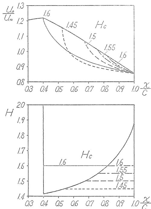
FIG. 2. The velocity distribution and the variations of shape factor.
