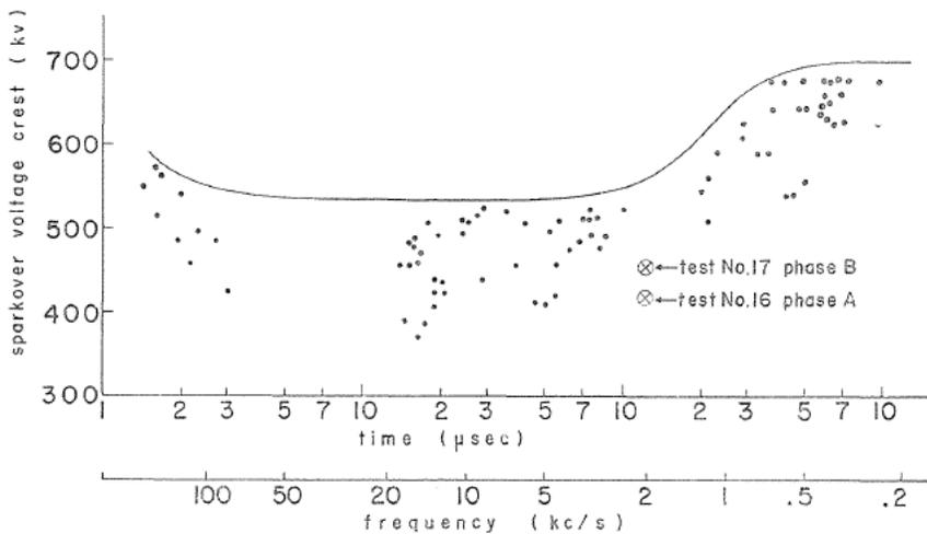
FIG. 6. 260 kv arrester  $V-t$  characteristics associated with the results obtained in this field test
