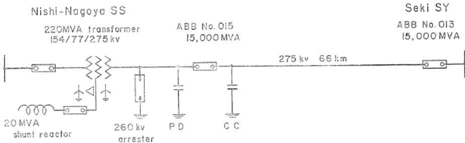
FIG. 2. Single-line schematic diagram of test line and terminal equipments
