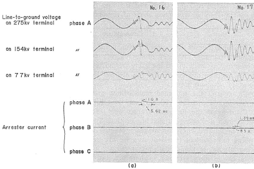
FIG. 5. Cathode-ray oscillograms of switching surges recorded on 220 mva transformer terminals and arrester currents
