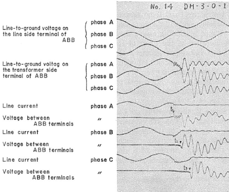
FIG. 3. Cathode-ray oscillograms of test No. 14
