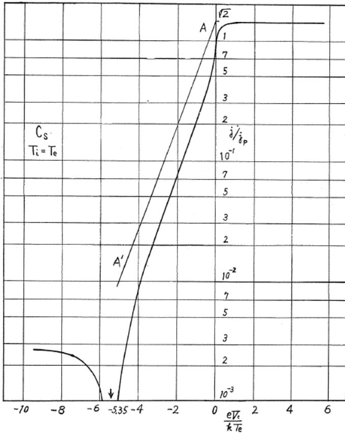
FIG. 9. The ideal Langmuir probe curve, in which the conditions  $r^2=1$  and  $E_0=0$  are imposed, for  $C_s$  assuming  $T_i=T_e$ . In the figure, the straight line  $A-A'$  shows the relation  $j/j_{es} = \exp(eV_c/kT_e)$ .
