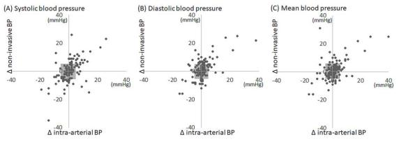
Black points show the change of each paired blood pressure within two minutes (∆ intraarterial BP: tracks the change of intra-arterial blood pressure; ∆ non-invasive BP: tracks the change of non-invasive blood pressure). The exclusion zone is ≤5 mmHg. (A) Systolic, (B) diastolic, and (C) mean blood pressure. BP, blood pressure.
