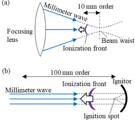
FIG. 2. Schematic images of the experiment conducted in the over-critical condition (a) [1,2] and the under-critical condition (b) [3,4].
