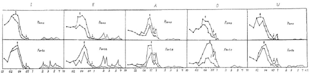
FIG. 7. Variation of timbre patterns of five vowels for subject F, caused by difference of vocal intensity: *piano* and *forte*.
