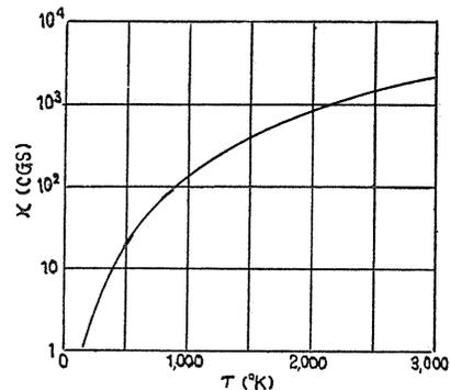
FIG. 2. The dependence of thermal conductivity on temperature.
