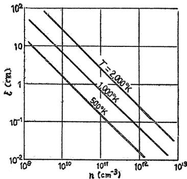
FIG. 1. Mean free path,  $l$ , versus number density,  $n$ , for various temperature.
