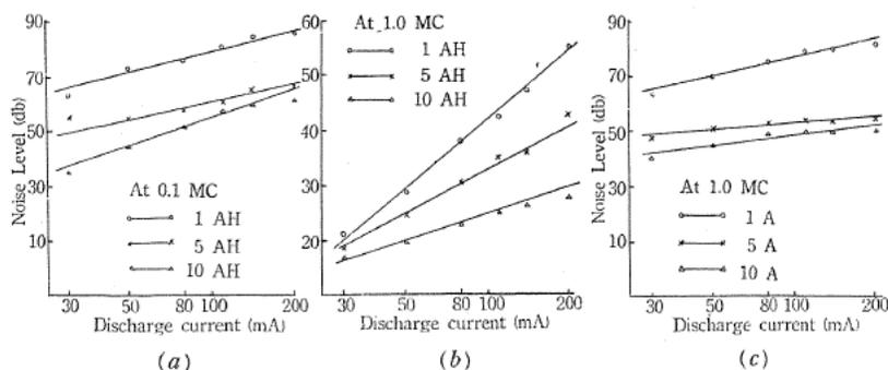
FIG. 3. Effect of discharge current on noise.
