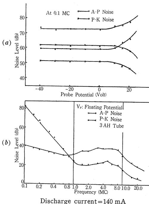
FIG. 4. (a) Effect of probe potential on noise. (b) Noise spectra measured between probe and anode, and between probe and cathode.
