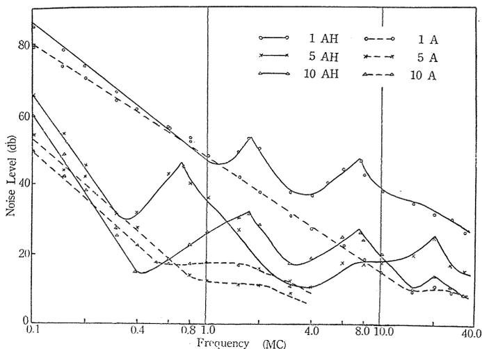
FIG. 2. Typical noise spectra of discharge tubes measured.
