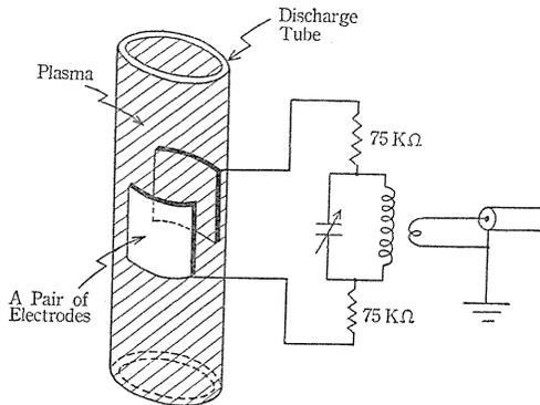
FIG. 1. A noise measuring circuit by a pair of small electrodes.
