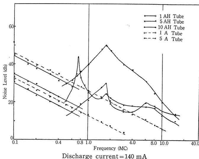
FIG. 5. Noise spectra measured by a pair of small electrodes located 10 cm apart from anode.
