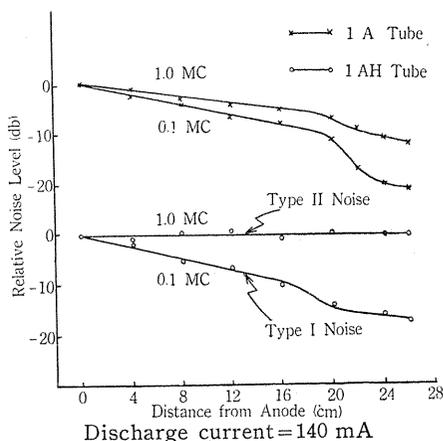
FIG. 6. Distribution of noise along axis of tube.
