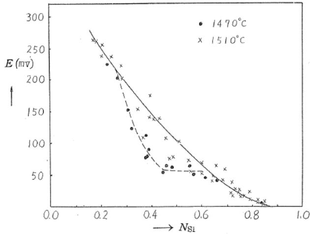
FIG. 1. e.m.f. -  $N_{Si}$  relations for Ni-Si alloys.
