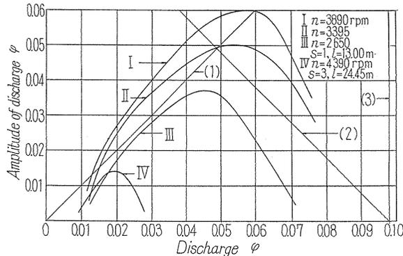
FIG. 3.13. Relation between working discharge of blower and amplitude of discharge variation.
