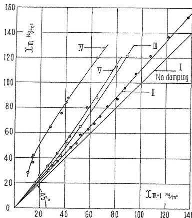
FIG. 2.11. Relation between position of small opening and damping of vibration,
