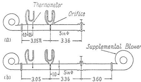
FIG. 2.1. Pipe-line systems for measurement of characteristic curve of blower.
