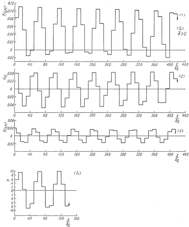
FIG. 1.14. Wave forms of surging in a pipe-line with a discontinuous cross section ( $\xi=0.5$ , areal ratio=1:2 and valve is closed).
