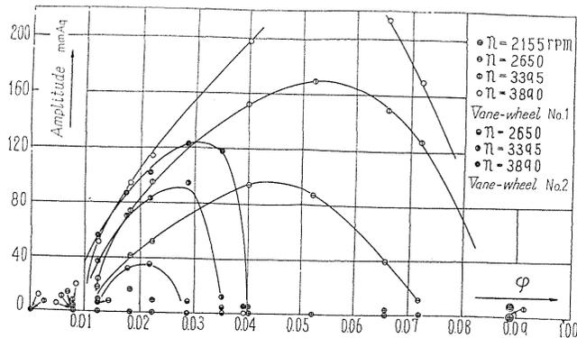
FIG. 3.7. Effects of rotating speed and working discharge of blower on surging.
