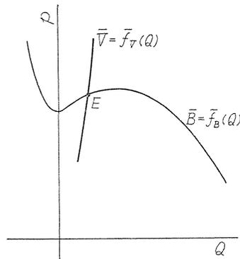
FIG. 1.2. Characteristics of blower and valve.
