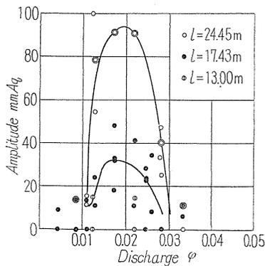
FIG. 3.11. Relation between pipe length and pressure amplitude of surging (orifice position *F* and type of surging  $s=3$ ).
