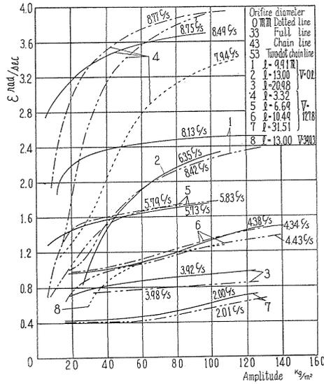
FIG. 2. 15. Equivalent damping coefficients for various pipe-lines.
