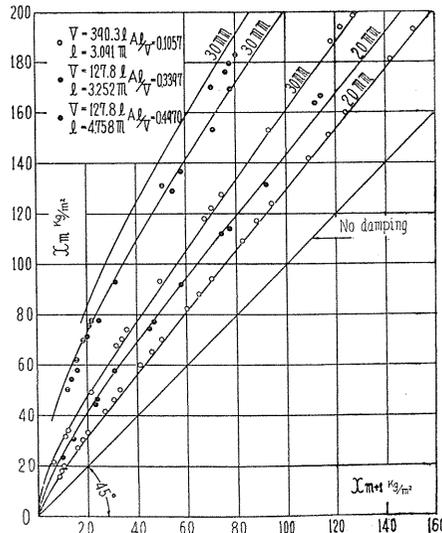
FIG. 2.10. Damping of vibration of fundamental mode (comparison between theoretical values and measured ones).
