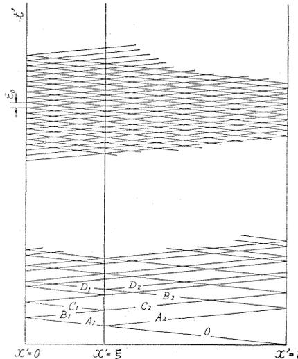
FIG. 1.5. Loci of propagating disturbance.
