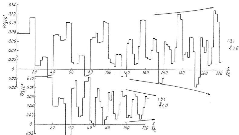
FIG. 1.10. Graphical solutions of transient pressure waves ( $\xi=0.3$  and valve is closed)
