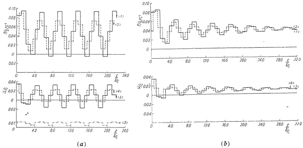
FIG. 1.13. Graphical solutions of surging ( $\xi=0.5$  and valve is slightly open). Working point of blower is unstable in (a) and stable in (b).
