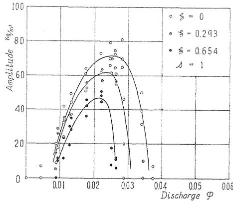
FIG. 4.2. Relation between pressure amplitude of surging and blower position in pipe-line (pipe-line I).
