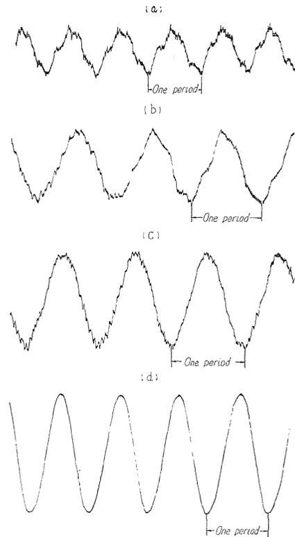
FIG. 3.5. Variation of wave form of surging along pipe-line.
