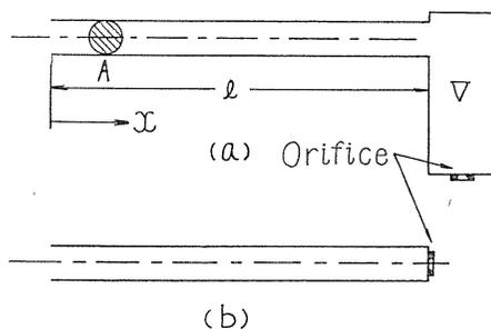
FIG. 2.3. Pipe-lines for measurement of free vibration of air column.
