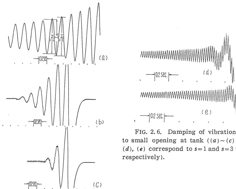
FIG. 2.6. Damping of vibration due to small opening at tank ((a)~(c) and (d), (e) correspond to  $s=1$  and  $s=3$  type respectively).
