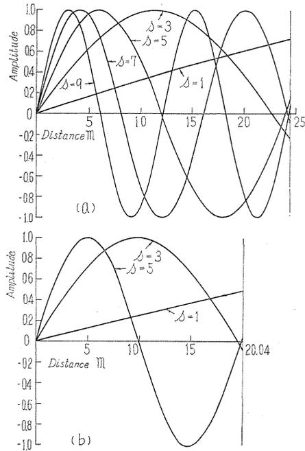
FIG. 4.1. Variation of pressure amplitude along pipe-line for various normal modes.
