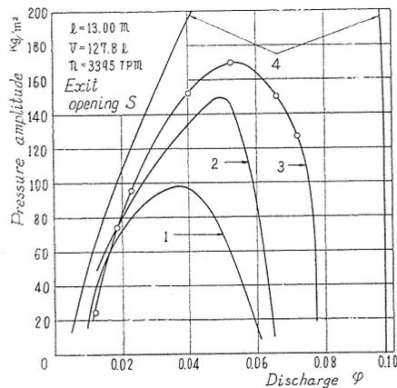
FIG. 5.3. Quantitative comparison between evaluated values of pressure amplitude and experimental values.
