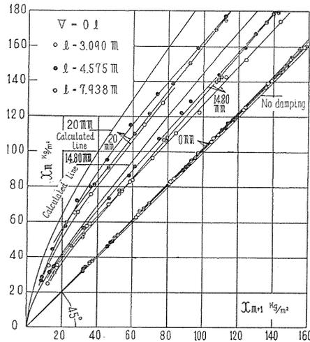
FIG. 2.9. Damping of vibration of fundamental mode ( $V=0 l$ ).
