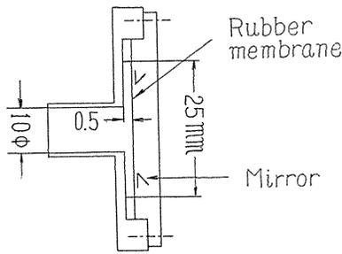
FIG. 2.4. Pressure indicator for measurement of free vibration.
