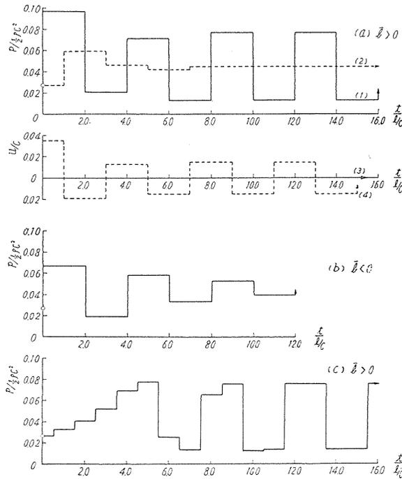
FIG. 1.9. Graphical solutions of surging ( $\xi=0$  and valve is closed).
