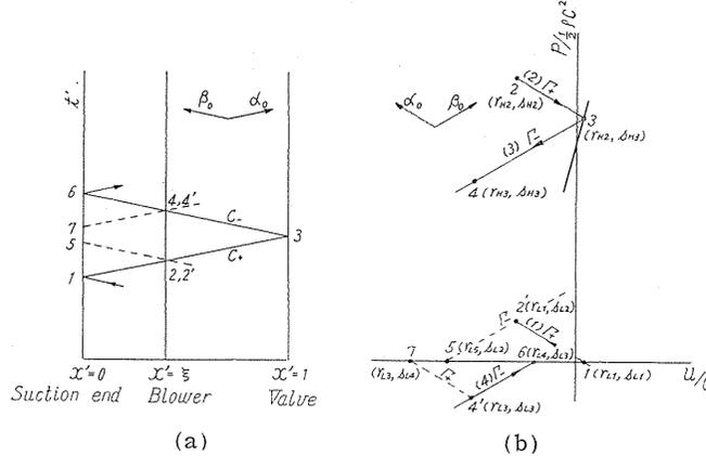
FIG. 1.7. Correspondence between the points on  $x', t'$  plane and those on  $p/(1/2)\rho c^2, u/c$  plane.
