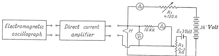
FIG. 3.3. Electric circuit for measurement of velocity variation.
