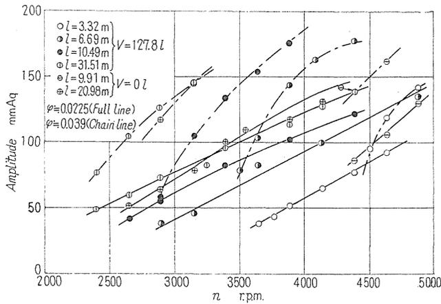
FIG. 3.8. Relation between rotating speed of blower and pressure amplitude of surging.
