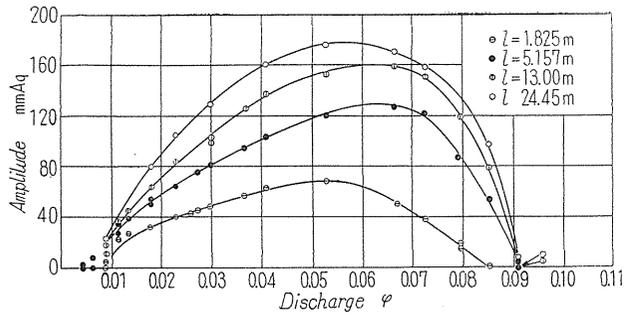
FIG. 3.9. Relation between pipe length and pressure amplitude of surging (orifice position *S* and type of surging  $s=1$ ).
