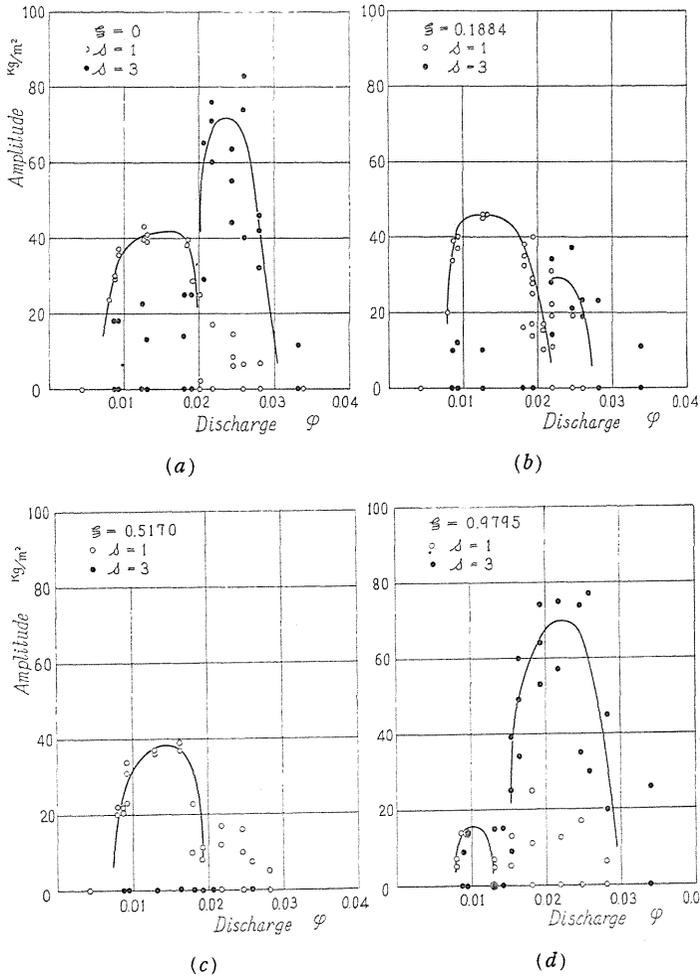
FIG. 4.7. Relation between pressure amplitude of surging and blower position in pipe-line; and change of type of surging.
