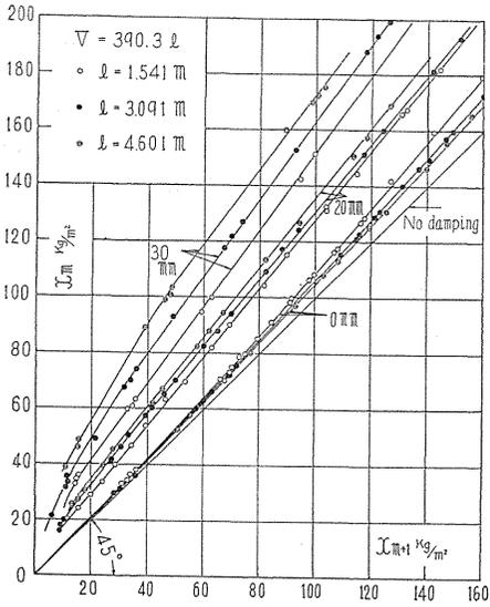
FIG. 2.7. Damping of vibration of fundamental mode ( $V=390.3 l$ ).
