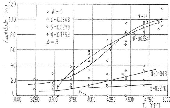
FIG. 4.4. Effect of rotating speed of blower on relation between pressure amplitude and blower position in pipe-line (pipe-line II).
