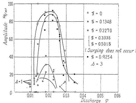
FIG. 4.3. Relation between pressure amplitude of surging and blower position in pipe-line (pipe-line II).
