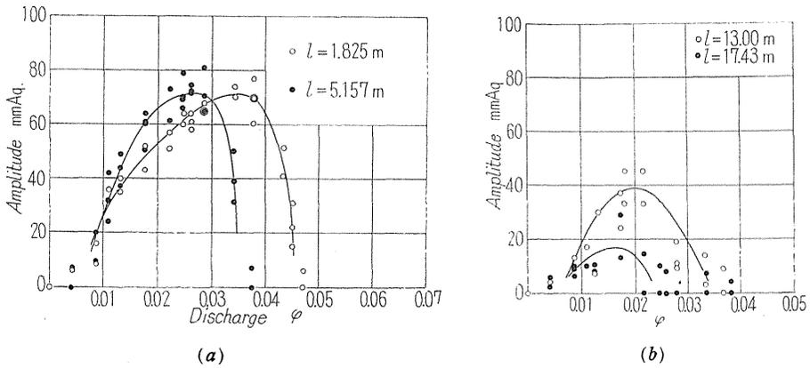
FIG. 3.10. Relation between pipe length and pressure amplitude of surging (orifice position *F* and type of surging  $s=1$ ).
