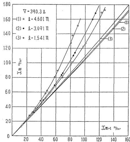
FIG. 2.14. Damping effect of blower on vibrating air column.
