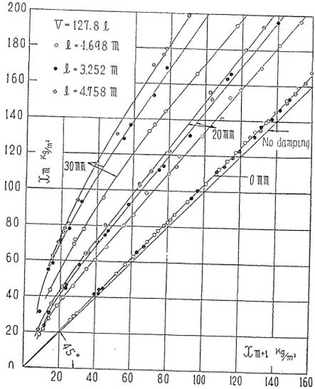
FIG. 2.8. Damping of vibration of fundamental mode ( $V=127.8 l$ ).
