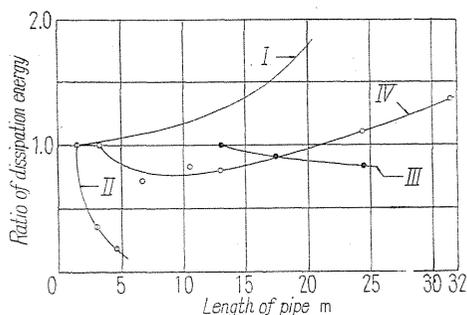
FIG. 3.14. Relation between energy dissipation and pipe length.
