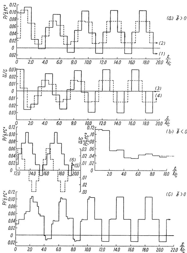
FIG. 1.11. Graphical solutions of surging ( $\xi=0.5$  and valve is closed).
