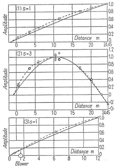
FIG. 3.4. Variation of pressure amplitude of surging along pipe-line.
