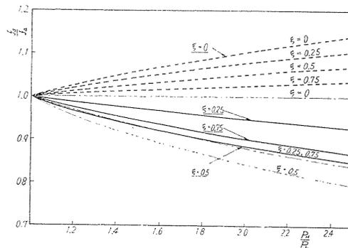
FIG. 1.15. Effect of compression ratio of blower on frequency of surging.
