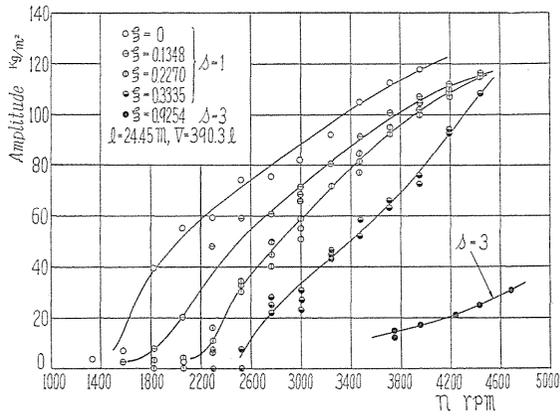
FIG. 4.6. Effect of rotating speed of blower on relation between pressure amplitude and blower position (pipe-line III).
