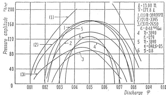
FIG. 5.2. Qualitative comparison between evaluated values of pressure amplitude of surging by approximation theory and experimental values.
