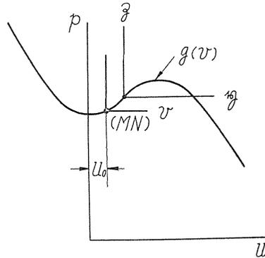
FIG. 5.1. Approximate representation of characteristic curve of blower by a cubic.
