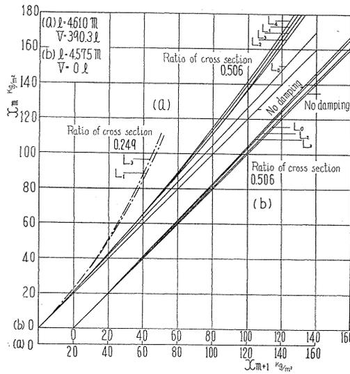
FIG. 2.12. Damping of vibration due to throttle valve inserted at a point of pipe-line.
