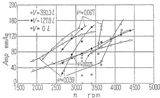
FIG. 3.12. Relation between tank volume and pressure amplitude of surging.
