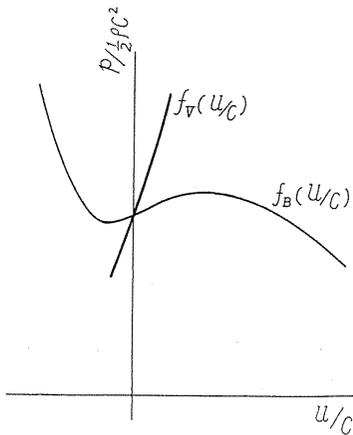
FIG. 1.4. Characteristics of blower and valve on  $p/(1/2)\rho c^2, u/c$  plane.
