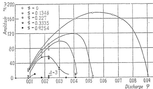
FIG. 4.5. Relation between pressure amplitude of surging and blower position in pipe-line (pipe-line III).
