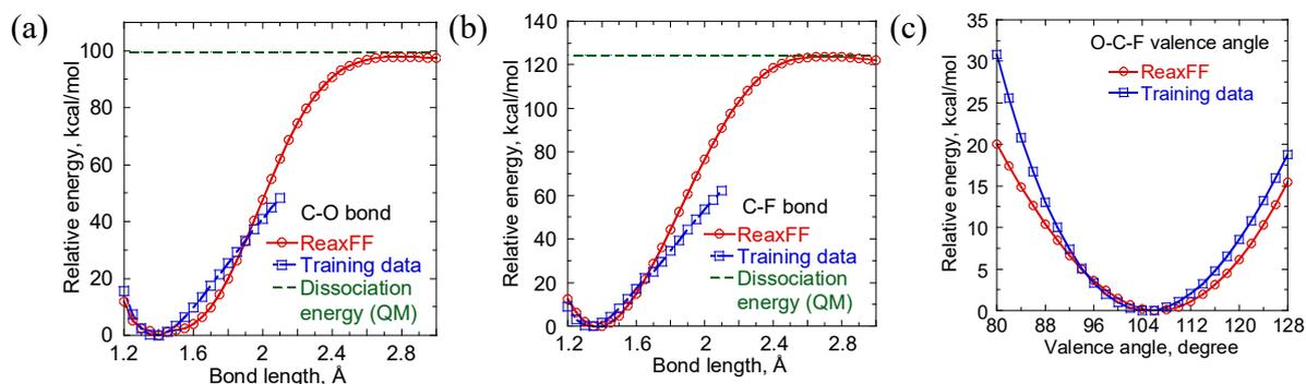
**Figure 3.** Comparison between results of the developed PFPE ReaxFF and training data from QM calculation: (a) C–O bond energy, (b) C–F bond energy, and (c) O–C–F valence angle energy. The bond dissociation energies (broken lines) in (a) and (b) were obtained by QM calculation.
