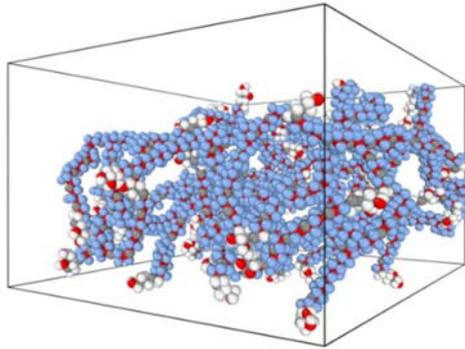
**Figure 1.** One initial configuration of the heating simulations. The system consisted of 36 D-4OH molecules. The gray, white, blue, and red represent carbon, hydrogen, fluorine, and oxygen atoms, respectively.
