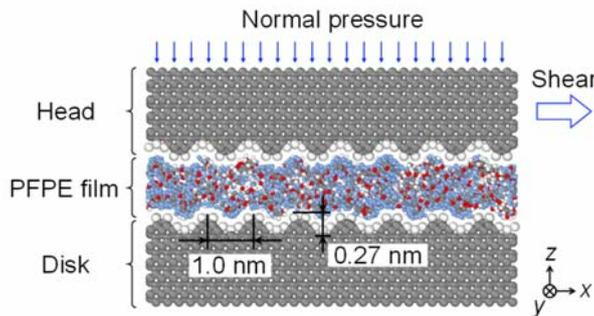
**Figure 2.** One initial configuration of the shearing simulations. Surface roughness with a peak-to-valley height of 0.27 nm and a period of 1.0 nm was introduced to suppress interfacial slip. The  $x$  and  $y$  dimensions of the simulation box were both set to 8.04624 nm, and periodic boundary conditions were applied in the two directions. The gray, white, blue, and red represent carbon, hydrogen, fluorine, and oxygen atoms, respectively.
