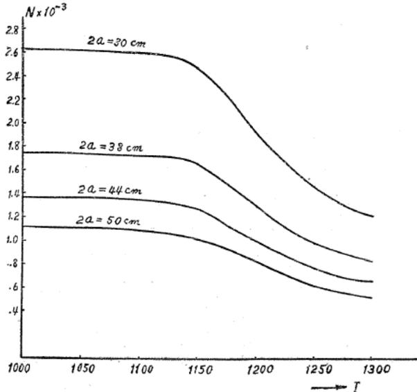
Fig. 6. Demagnetizing factor specimen of pure iron.  $d = 0.5$  mm,  $2b = 9.74$  mm,  $2a = 50 \sim 30$  cm.
