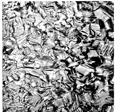
FIG. 22. Annealed at 600°C, before stressing (800×).
