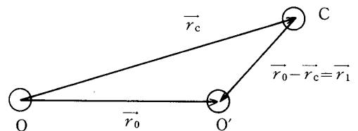
$$M\vec{a}_0 = -G \frac{MM_s}{r_0^3} \vec{r}_0 - G \frac{MM_c}{r_1^3} \vec{r}_1$$
