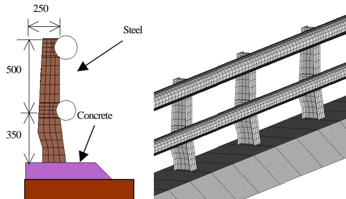
Figure 2: Steel fence model (mm)
