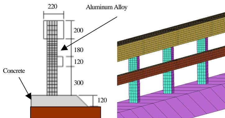
Figure 3: Aluminum alloy fence model (mm)
