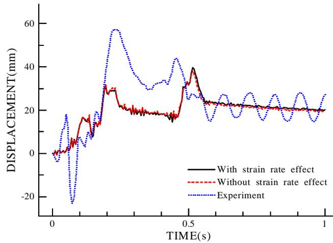
Figure 9: Displacement response at the top of column8 (Aluminum alloy bridge guard fence)
