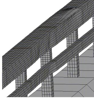
Figure 11: Mode shape of the aluminum alloy guard fence
