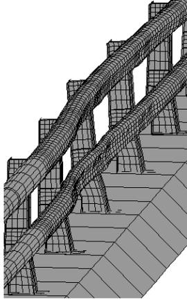
Figure 10: Mode shape of the steel guard fence
