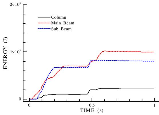
Figure 12: Energy distribution of the steel guard fence
