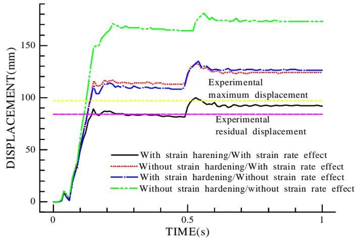
Figure 8: Displacement response at the top of column10 (Steel bridge guard fence)
