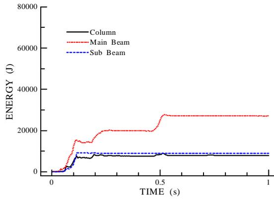
Figure 13: Energy distribution of the aluminum alloy guard fence
